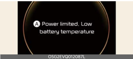
A: Power limited. Low battery temperature
