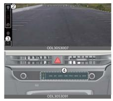
The front view function displays the vehicle's front situation on the navigation system according to the driver's settings, assisting in safe driving.
