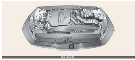
\* The actual engine compartment in your Kia may differ from the illustration. 1. Engine coolant reservoir 8-19 8-21 2. Brake fluid reservoir 3. Air cleaner 8-14 4. Engine oil dipstick 8-17 5. Engine oil filler cap 8-17 6. Windshield washer fluid reservoir 8-23 7. Fuse box 8-45 8. Positive battery terminal 8-27 9. Negative battery terminal 8-27
