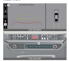
The rearview function of the Surround View Monitor displays the vehicle's rear situation on the navigation system according to the driver's settings, assisting in safe parking.
