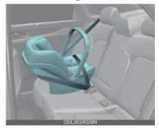
A rear-facing child seat provides restraint with the seating surface against the back of the child. The harness system holds the child in place, and in an accident, acts to keep the child positioned in the seat and reduces the stress to the neck and spinal cord. They should be used in rear seating positions only. All children under age one must always ride in a rear-facing infant child restraint. Convertible and 3-in-1 child seats typi-
