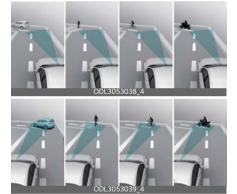
Forward Collision-Avoidance Assist may not detect other vehicles, powered two-wheelers, pedestrians or cyclists in front of you when driving on curved roads adversely affecting the performance of the sensors. This may result in no warning, braking assist when necessary.
