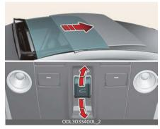
Push the sunroof switch rearward to the first detent position, the sunroof glass opens. However, if the power sunshade is close, the power sunshade will open first. Push the sunroof switch forward to the first detent position, the sunroof glass closes. If the sunroof glass is close, the power sunshade will close.
