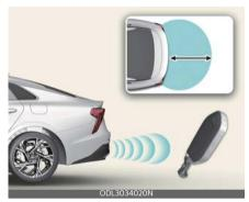
The Smart Trunk operates with a welcome alert if the smart key is detected within 20-39 inches (50-100 cm) from the trunk
