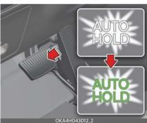
When coming to a complete stop by pressing the brake pedal, the AUTO HOLD indicator changes from white to green indicating the AUTO HOLD is engaged. The vehicle will remain at a
