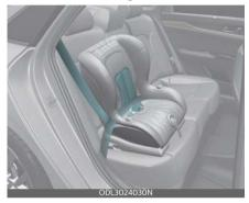
All passenger seat belts move freely under normal conditions and only lock under extreme or emergency conditions (emergency locking mode). To secure a child restraint, you must manually pull the seat belt all the way out to shift the retractor to the "automatic locking" mode.
