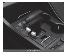
Whether the vehicle is stationary or in motion, manual mode can be selected by pushing the shift lever from the D (Drive) position into the manual gate. To return to D (Drive) range operation, push the shift lever back into the main gate. Manual mode manages the driving dynamics by automatically adjusting the steering effort, and the engine and transmission control logic for enhanced
