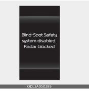
When the rear bumper around the rear corner radar or sensor is covered with foreign material, such as snow or rain, or installing a trailer or carrier, it can reduce the detecting performance and temporarily limit or disable Blind-Spot Collision-Avoidance Assist.
