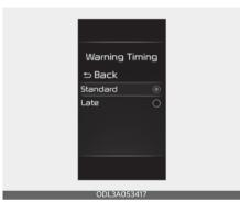
With the ENGINE START/STOP button in the ON position, select 'Driver Assistance → Warning Timing' from the Settings menu to change the initial warning activation time for Rear Cross-Traffic Collision-Avoidance Assist.
