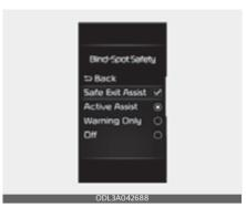
With the ENGINE START/STOP button in the ON position, select 'Driver Assistance → Blind-Spot Safety → Safe Exit Assist' from the Settings menu to turn on Safe Exit Assist and deselect to turn off the function
