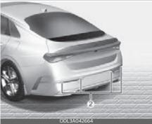
[1]: Wide-rear view camera[2]: Rear ultrasonic sensors
