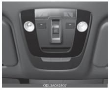
The sunroof can only be operated when the ENGINE START/STOP button is in the ON or START position. The sunroof can be operated for approximately 10 minutes after the ENGINE START/STOP button is in the ACC or OFF position. However, if the front door is open, the sunroof cannot be operated even within the 10 minutes period.
