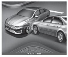
In an angled collision, the force of impact may direct the occupants in a direction where the air bags would not be able to provide any additional benefit, and thus the sensors may not deploy any air bags.
