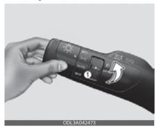
The fog lights will turn on when the fog light switch (1) is turned to the on position after the headlight is turned on.
