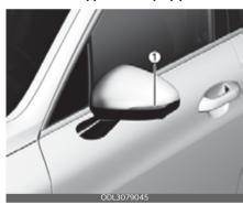
If the side repeater lamp LED (1) does not operate, have the vehicle checked by an authorized Kia dealer.
