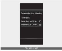
With the ENGINE START/STOP button in the ON position, select or deselect 'Driver Assistance → Driver Attention Warning' from the Settings menu to set whether or not to use each function.
