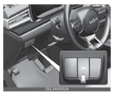
With the ENGINE START/STOP button in the ON position, press the Lane Safety button located on the instrument panel to turn on Lane Keeping Assist. The
