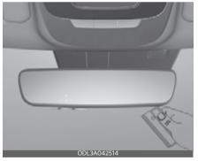
3. While the HomeLink indicator light (7) is flashing orange, press and hold the hand-held remote button. Continue pressing the hand-held remote button until the HomeLink indicator light (7) light changes from orange to green. You may now release the hand-held remote button.
