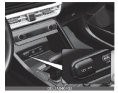
The devices should draw less than 10 amps with the vehicle on.
