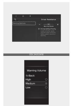
You can adjust the Warning Methods with the ignition switch or ENGINE START/ STOP button in the ON position.
