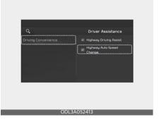
With the ENGINE START/STOP button in the ON position, select 'Driver Assistance → Driving Convenience → Highway Auto Speed Change' from the Settings menu to turn on Navigation-based Smart Cruise Control and deselect to turn off the function.
