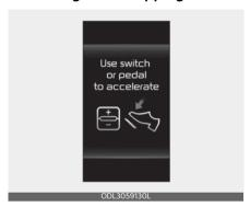
When Highway Driving Assist is operating, your vehicle will stop if the vehicle ahead of you stops. Also, if the vehicle ahead of you starts moving approximately within 30 seconds after the stop, your vehicle will start as well. In addition, after the vehicle has stopped and approximately 30 seconds have passed, the 'Use switch or pedal to accelerate' message will appear on the cluster. Depress the accelerator pedal or operate the + switch, - switch or | switch to start driving.
