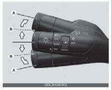
The ENGINE START/STOP button must be on for the turn signals to function. To turn on the turn signals:
