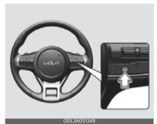
With the ENGINE START/STOP button in the ON position, shortly press Lane Following Assist button located on the steering wheel to turn on Lane Following Assist. The white or green indicator light will appear on the cluster.
