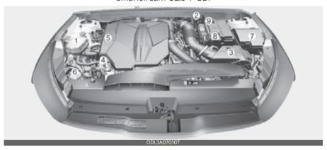
\* The actual engine room in the vehicle may differ from the illustration. 1. Engine coolant reservoir 8-21 8-24 2. Brake fluid reservoir 3. Air cleaner 8-26 4. Engine oil dipstick 8-18 5. Engine oil filler cap 8-18 6. Windshield washer fluid reservoir 8-25 7. Fuse box 8-47 8-31 8. Positive battery terminal 9. Negative battery terminal 8-31
