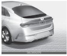
[1]: Wide-rear view camera Refer to the picture for the detailed location of the detecting sensor.
