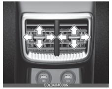
You can adjust the direction of air delivered from these vents using the vent control lever as shown. If you do not want the air delivered, place the vent control lever to the close  $\bigotimes$  position.
