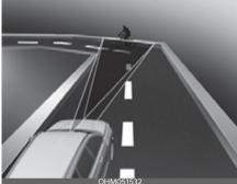
Forward Collision-Avoidance Assist may detect a vehicle, pedestrian or cyclist in the next lane or outside the lane when driving on a curved road. If this occurs, Forward Collision-Avoidance Assist may unnecessarily warn the driver and control the brake. Always check the traffic conditions around the vehicle.
