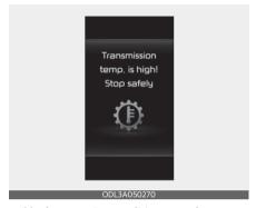
Under certain conditions, such as repeated stop-and-go launches on steep grades, sudden take off or acceleration, or other harsh driving conditions, the clutch temperature will increase excessively. Finally, the clutch in transmission could be over-
