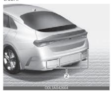
The rear ultrasonic sensors (2) are located inside the rear bumper to detect objects in the rear area. If the sensors are covered with foreign material, such as snow or rain, it may adversely affect sensor performance and Reverse Parking Collision-Avoidance Assist may not
