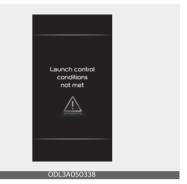
If you use Launch Control when the transmission oil temperature exceeds a certain level, a warning message will be displayed and the Launch Control will not be activated.
