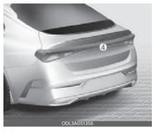
[4]: Wide-rear view camera Refer to the picture for the detailed location of the detecting sensors.
