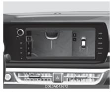
If top view is selected, the top view will be displayed on the right side of top view in Surround View Monitor screen. • The top view also works in pair with the front top view and rear top view quideline display.
