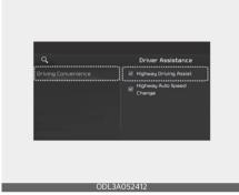
With the ENGINE START/STOP button in the ON position, select or deselect 'Driver Assistance → Driving Convenience' from the Settings menu to set whether or not to use each function.
