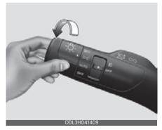
When the light switch is in the position lamp position, the front position lamp and auxiliary lamp (if equipped), tail, license light will turn ON.
