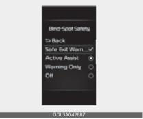
With the ENGINE START/STOP button in the ON position, and select 'Driver Assistance → Blind-Spot Safety → Safe Exit Warning' to turn on Safe Exit Warning and deselect to turn off.
