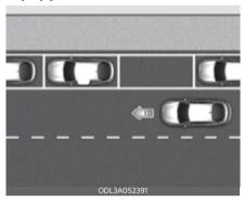
After the vehicle stops, when an approaching vehicle from the rear area is detected as soon as a passenger opens a door, Safe Exit Assist will warn the driver with a warning message and an audible warning to help prevent a collision.
