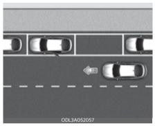
After the vehicle stops, when an approaching vehicle from the rear area is detected as soon as a passenger opens a door, Safe Exit Warning will warn the driver with a warning message and an audible warning to help prevent a collision.
