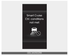
If the Driving Assist to button, + switch, - switch or | switch is operated when Smart Cruise Control's operating conditions are not satisfied, the 'Smart Cruise Control conditions not met' will appear on the cluster, and an audible warning will sound.
