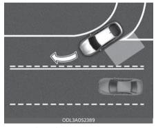
Blind-Spot Collision-Avoidance Assist may not operate properly when driving where the road merges or divides. Blind-Spot Collision-Avoidance Assist may not detect the vehicle in the next lane.
