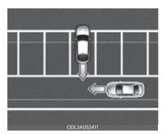
Rear Cross-Traffic Collision-Avoidance Assist may detect vehicles passing by behind you when parking backwards into a parking space. If this occurs, the function may unnecessarily warn the driver and control the brake.
