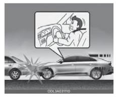
Front air bags are not designed to inflate in rear collisions, because occupants are moved backward by the force of the impact. In this case, inflated air bags would not be able to provide any additional benefit.
