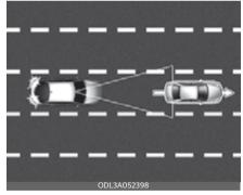
If the vehicle in front abruptly departures, Leading Vehicle Departure Alert may not operate properly.
