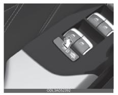
In addition, when the electronic child safety lock button is in the LOCK position and an approaching vehicle from the rear area is detected, the electronic child safety lock button will not unlock even if the driver presses the button to prevent the rear doors from opening.
