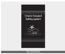
When Forward Collision-Avoidance Assist is not working properly, the 'Check Forward Safety system' warning message will appear, and the and
