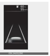
If the vehicle ahead and/or both lane markings are detected and your driving speed is below 110 mph (180 km/h), the green indicator light will appear on the cluster, and the function will help the vehicle stay in lane by assisting the steering wheel.
