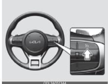
Press the Driving Assist 50 button to turn Smart Cruise Control off.
