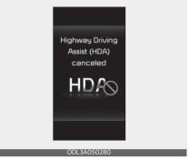
If the driver still does not have their hands on the steering wheel after the hands-off warning, the 'Highway Driving Assist (HDA) canceled' warning message will appear and Highway Driving Assist and Lane Following Assist will be automatically canceled.
