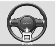
The horn will operate only when this area is pressed. Check the horn regularly to be sure it operates properly.
