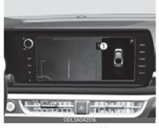
When you touch the icon (1), the top view is displayed on the screen and shows the distance from the vehicle behind you while parking.
