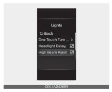
With the ENGINE START/STOP button in the ON position, select 'Lights → High Beam Assist' from the Settings menu to turn on High Beam Assist and deselect to turn off the function.
