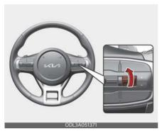
Push the + switch up or - switch down or press the | | switch to resume Cruise Control.
