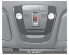
The sunroof can only be operated when the ENGINE START/STOP button is in the ON or START position. The sunroof can be operated for approximately 10 minutes after the ENGINE START/STOP button is in the ACC or OFF position. However, if the front door is open, the sunroof cannot be operated even within the 10 minutes period.
