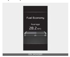
The trip computer mode displays information related to vehicle driving parameters including fuel economy, tripmeter information and vehicle speed.
