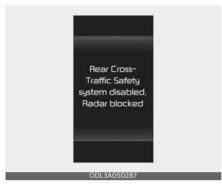
When the rear bumper around the rearside radar or sensor is covered with foreign material, such as snow or rain, or towing a trailer or carrier, it can reduce the detecting performance and temporarily limit or disable Rear Cross-Traffic Collision-Avoidance Assist.
