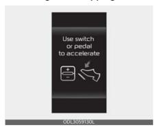
When Highway Driving Assist is operating, your vehicle will stop if the vehicle ahead of you stops. Also, if the vehicle ahead of you starts moving approximately within 30 seconds after the stop, your vehicle will start as well. In addition, after the vehicle has stopped and approximately 30 seconds have passed, the 'Use switch or pedal to accelerate' message will appear on the cluster. Depress the accelerator pedal or operate the + switch, - switch or \(\text{V} \) switch to start driving.
