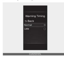
With the ENGINE START/STOP button in the ON position, select 'Driver Assistance → Warning Timing' from the Settings menu to change the initial warning activation time for Driver Attention Warning. When the vehicle is first delivered, Warning Timing is set to 'Normal'. If you change the Warning Timing, the warning time of other Driver Assistance systems may change.
