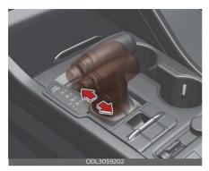
Whether the vehicle is stationary or in motion, manual mode can be selected by pushing the shift lever from the D (Drive) position into the manual gate. To return to D (Drive) range operation, push the shift lever back into the main gate. Manual mode manages the driving
