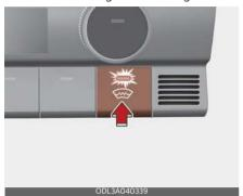
If there is heavy accumulation of snow on the front window, brush it off before operating the front glass heater.
