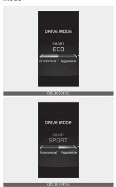
With the standard driving style in the center, the left side of the gauge is 'Econ.' and right side is 'Dynamic' style. When the left side of the driver's style gauge is filled up and after a certain time passes, the SMART ECO mode is activated automatically. When the right side of the gauge is filled up and sporty driving condition is detected, the SMART SPORT mode is activated.
