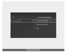
With the ENGINE START/STOP button in the ON position, select or deselect 'Driver Assistance → Parking Safety' from the Settings menu to set whether or not to use the function.
