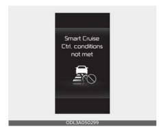
If the Driving Assist The button, + switch, - switch or \(\bigcap\_{\infty}\) switch is operated when Smart Cruise Control's operating conditions are not satisfied. the 'Smart Cruise Control conditions not met' will appear on the cluster, and an audible warning will sound.
