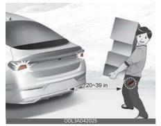
If you are positioned in the detecting area (20~39 inches (50~100 cm)) behind the vehicle) carrying a smart key, the hazard warning lights will blink and chime will sound to alert you the smart key has been detected and the trunk will open.
