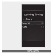
With the ENGINE START/STOP button in the ON position, select 'Driver Assistance → Warning Timing' from the Settings menu to change the initial warning activation time for Rear Cross-Traffic Collision-Avoidance Assist.
