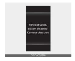
When the front windshield where the front view camera is located, is covered with foreign material, such as snow or rain, it can reduce the detecting performance and temporarily limit or disable Forward Collision-Avoidance Assist. If this occurs, the 'Forward Safety system disabled. Camera obscured' warning message, and the same and safety and safety warning lights will illuminate on the cluster
