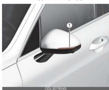
If the side repeater lamp LED (1) does not operate, have the vehicle checked by an authorized Kia dealer.
