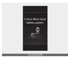
When Blind-Spot Collision-Avoidance Assist is not working properly, the 'Check Blind-Spot Safety system' warning message will appear on the cluster, and Blind-Spot Collision-Avoidance Assist will turn off automatically or Blind-Spot Collision-Avoidance Assist will be limited. In this case, have your vehicle inspected by an authorized Kia dealer.
