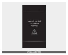
If you use Launch Control when the transmission oil temperature exceeds a certain level, a warning message will be displayed and the Launch Control will not be activated.
