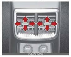
You can adjust the direction of air delivered from these vents using the vent control lever as shown. If you do not want the air delivered, place the vent control lever to the close opinion
