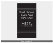
When Highway Driving Assist is not working properly, the 'Check Highway Driving Assist (HDA) system' warning message will appear, and the warning light will illuminate on the cluster. In this case, have your vehicle inspected by an authorized Kia dealer.
