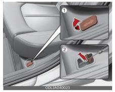
Open the cable cover(1) under the rear seat with a mechanical key and pull the cable (2) for unlocking the trunk. The cable is fixed firmly so it may hard to pull. Therefore, please put auxiliary equipment such as a screwdriver to the loop and pull it comfortably.
