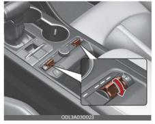
The temperature setting of the seat changes according to the levers position.
