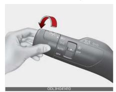
When the light switch is in the head light position, head light (low beam), tail, license light will turn ON.
