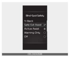
With the ENGINE START/STOP button in the ON position, select 'Driver Assistance → Blind-Spot Safety → Safe Exit Assist' from the Settings menu to turn on Safe Exit Assist and deselect to turn off the function
