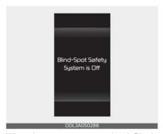
When the engine is restarted with Blind-Spot Collision-Avoidance Assist off, the 'Blind-Spot Safety System is Off' message will appear on the cluster.
