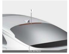
If the high mounted stop lamp (LED type) (1) does not operate, have the vehicle checked by an authorized Kia dealer.
