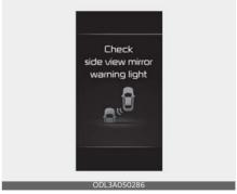
When the side view mirror warning light is not working properly, the 'Check side view mirror warning light' warning message will appear on the cluster. In this
