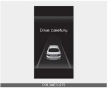
When the vehicle is stopped due to emergency braking, the 'Drive carefully' warning message will appear on the cluster.
