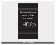
If the driver still does not have their hands on the steering wheel after the hands-off warning, the 'Highway Driving Assist (HDA) canceled' warning message will appear and Highway Driving Assist and Lane Following Assist will be automatically canceled.
