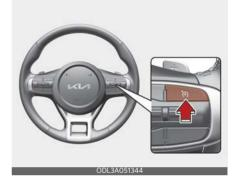
Release the accelerator pedal. The desired speed will automatically be maintained.
