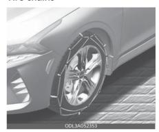
Since the sidewalls on some radial tires are thinner than other types of tires, they may be damaged by mounting certain types of tire chains on them. Therefore, the use of snow tires is recommended instead of tire chains. Do not mount tire chains on vehicles equipped with aluminum wheels; if unavoidable, use a wire type chain. Install the tire chain after reviewing the instructions provided with the tire chains.
