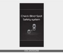
When Safe Exit Warning is not working properly, the 'Check Blind-Spot Safety system' warning message will appear on the cluster, and Safe Exit Warning will turn off automatically or Safe Exit Warning will be limited. In this case, have your vehicle inspected by an authorized Kia dealer.
