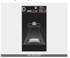
If you want to speed up temporarily when Smart Cruise Control is on, depress the accelerator pedal. While the speed is increasing, the set speed, distance level and target distance will blink on the cluster.
