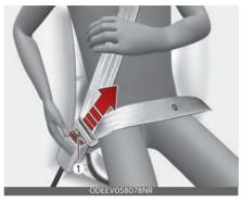
• Press the release button (1) in the locking buckle.
