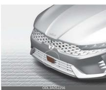
[1]: Front view camera, [2]: Front radar Refer to the picture for the detailed location of the detecting sensors.
