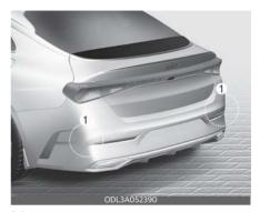
[1]: Rear corner radar Refer to the picture for the detailed location of the detecting sensors.
