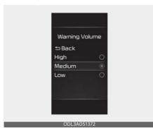
With the ENGINE START/STOP button in the ON position, select 'Driver Assistance → Warning Volume' from the Settings menu to change the Warning Volume to 'High', 'Medium' or 'Low' for Forward Collision-Avoidance Assist.
