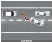
When a vehicle in front of you merges out of the lane, Smart Cruise Control may not immediately detect the new vehicle that is now in front of you.
