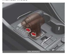
Whether the vehicle is stationary or in motion, manual mode can be selected by pushing the shift lever from the D (Drive) position into the manual gate. To return to D (Drive) range operation, push the shift lever back into the main gate. Manual mode manages the driving dynamics by automatically adjusting the steering effort, and the engine and transmission control logic for enhanced driver performance.
