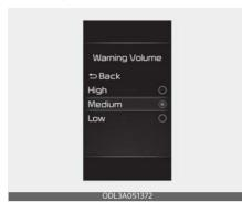
With the ENGINE START/STOP button in the ON position, select 'Driver Assistance → Warning Volume' from the Settings menu to change the Warning Volume to 'High', 'Medium' or 'Low' for Hands-off warning.
