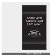
When Lane Keeping Assist is not working properly, the 'Check Lane Keeping Assist (LKA) system' warning message will appear and the yellow randicator light will illuminate on the cluster. If this occurs, have your vehicle inspected by an authorized Kia dealer.
