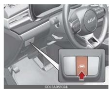
With the ENGINE START/STOP button in the ON position, press the Lane Safety button located on the instrument panel to turn on Lane Keeping Assist. The white 'a indicator light will illuminate on the cluster.
