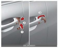
If you lock the driver's door with a mechanical key, the driver's door will lock. If you unlock the driver's door with a mechanical key, you can open and close the driver's door only.
