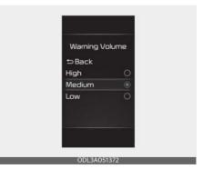
With the ENGINE START/STOP button in the ON position, select 'Driver Assistance → Warning Volume' from the Settings menu to change the Warning Volume to
