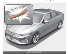
When all the doors (and trunk) are closed and locked, the door handle lamp will come on for about 15 seconds if any of the below is performed.
