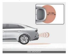
The Smart Trunk operates with a welcome alert if the smart key is detected within 20~39 inches (50~100 cm) from the trunk.
