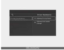
With the ENGINE START/STOP button in the ON position, select or deselect 'Driver Assistance → Driving Convenience' from the Settings menu to set whether or not to use each function.
