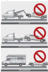
Do not tow the vehicle backwards with the front wheels on the ground, as this may cause damage to the transmission.
