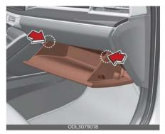
Remove the climate control air filter cover by pulling out right side of the cover.
