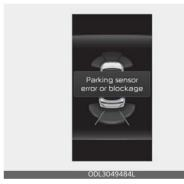
The 'Rear camera error or blockage' or 'Parking sensor error or blockage' warning message will appear on the cluster if the following situations occur:
