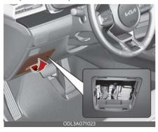
3. Pull the suspected fuse straight out.
