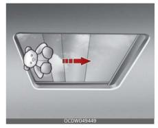
If the power sunshade or sunroof glass senses any obstacle while it is closing automatically, it will reverse direction then stop at a certain position. The auto reverse function may not work if an object thin or soft is caught between the sliding power sunshade or sunroof glass and sunroof sash.
