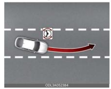
Lane Keeping Assist is designed to help detect lane markings while driving over a certain speed. Lane Keeping Assist will warn the driver if the vehicle leaves the lane without using the turn signal, or will automatically assist the driver's steering to help prevent the vehicle from departing the lane.
