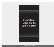
When Rear Cross-Traffic Collision-Avoidance Assist is not working properly, the 'Check Rear Cross-Traffic Safety system' warning message will appear on the cluster, and Rear Cross-Traffic Collision-Avoidance Assist will turn off automatically or it will be limited. In this case, have your vehicle inspected by an authorized Kia dealer.
