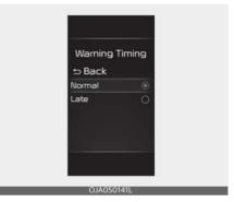
With the ENGINE START/STOP button in the ON position, select 'Driver Assistance → Warning Timing' from the Settings menu to change the initial warning activation time for Forward Collision-Avoidance Assist.
