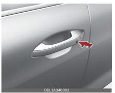
Pressing the button of the front driver side door handles with all doors (and trunk) closed and any door unlocked, locks all the doors (and trunk). If all doors (and trunk) and engine hood are closed, the hazard warning lights will blink once and the chime will sound once to indicate.
