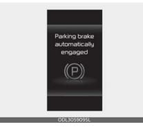
When the conversion from AUTO HOLD to EPB is not working properly a warning will sound and a message will appear.
