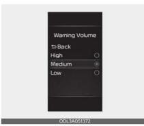
With the ENGINE START/STOP button in the ON position, select 'Driver Assistance → Warning Volume' from the Settings menu to change the Warning Volume to 'High', 'Medium' or 'Low' for Rear Cross-Traffic Collision-Avoidance Assist.
