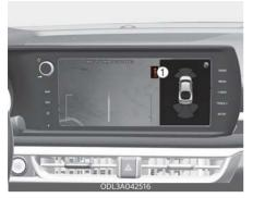
When you touch the icon (1), the top view is displayed on the screen and shows the distance from the vehicle in the back of your vehicle while parking.
