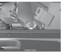
Use a funnel to help prevent oil from being spilled on engine components. Use only the specified engine oil. (Refer to "Recommended lubricants and capacities" on page 9-7.)
