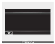
This gauge indicates the current outside air temperatures within 1°F (1°C).
