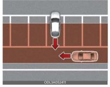
Rear Cross-Traffic Collision Warning may detect vehicles passing by behind you when parking backwards into a parking space. If this occurs, the function may unnecessarily warn the driver. Always check your surroundings while backing up.
