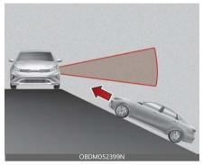
Rear Cross-Traffic Collision Warning may be limited when the vehicle is on a uphill or downhill slope, or near it, and may not detect the vehicle approaching from the left or right. If this occurs, the function may not warn the driver.
