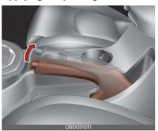
To engage the parking brake, first apply the foot brake and then pull up the parking brake lever as far as possible.
