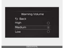
With the ignition switch or ENGINE START/STOP button in the ON position, select 'Driver Assistance → Warning Volume' from the 'User Settings (LCD display) or Setup → Vehicle (Infotainment System screen)' menu to change the Warning Volume to 'High', 'Medium' or 'Low' for Lane Keeping Assist.
