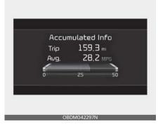
The trip computer mode displays information related to vehicle driving parameters including Accumulated info, Driving information, etc.
