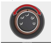
Air can be directed to the floor, dashboard outlets, or windshield. Five symbols are used to represent Face, Bi-Level, Floor, Floor-Defrost and Defrost air position.
