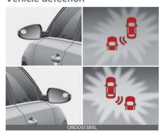
To warn the driver a vehicle is detected, the warning light on the side view mirror will illuminate.  Blind-Spot Collision-Avoidance Assist will operate when your vehicle speed is above 12 mph (20 km/h) and the speed of the vehicle in the blind spot area is above 7 mph (10 km/h).
