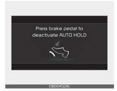
When you press the [AUTO HOLD] switch, if the driver's door, trunk, and hood is not closed, a warning will sound and a message will appear on the LCD display.
