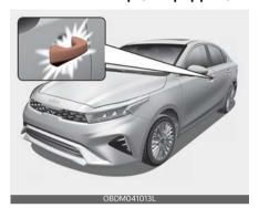
When all the doors (and trunk) are closed and locked, the door handle lamp will illuminate for about 15 seconds if any of the following is performed:
