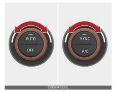
The temperature will increase to the maximum (HI) by rotating the knob in a clockwise direction.
