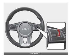
To resume Manual Speed Limit Assist after the function was canceled, operate the +, - or | switch.
