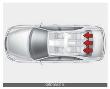
The rear seat is equipped with headrests for the occupant's safety and comfort. The headrest not only provides comfort, but also helps to protect the head and neck in the event of a collision.
