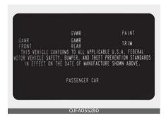
The certification label is located on the driver's door sill at the center pillar.
