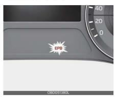
If the EPB malfunction indicator remains on, it indicates that the EPB may have malfunctioned. If this occurs, have the system checked by an authorized Kia dealer.
