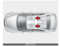
The driver's and front passenger's seats are equipped with a headrest for safety and comfort.
