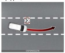
Lane Keeping Assist is designed to help detect the lane markers while driving over a certain speed. Lane Keeping Assist will warn the driver if the vehicle leaves the lane without using the turn signal, or will automatically assist the driver's steering to help prevent the vehicle from departing the lane.
