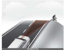
Forward Collision-Avoidance Assist may not detect a vehicle, pedestrian
