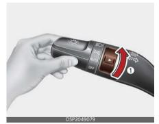
The fog lights will turn on when the fog light switch (1) is turned to the on position after the headlights are turned on.
