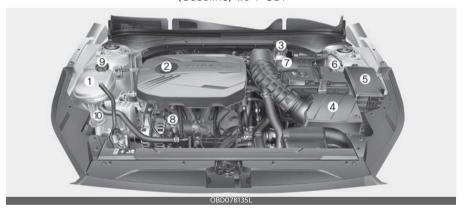
\* The actual engine compartment in your Kia may differ from the illustration. 1. Engine coolant reservoir 8-20 2. Engine oil filler cap 8-18 3. Brake / clutch fluid reservoir 8-23 4. Air cleaner 8-26 5. Fuse box 8-49 6. Negative battery terminal 8-31 7. Positive battery terminal 8-31 8. Engine oil dipstick 8-18 8-20 9. Radiator cap 10. Windshield washer fluid reservoir 8-24
