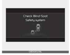
When Safe Exit Warning is not working properly, the 'Check Blind-Spot Safety system' warning message will appear on the cluster for several seconds, and the master (\( \bigcap \)) warning light will illuminate on the cluster. In this case, have the vehicle inspected by an authorized Kia dealer.
