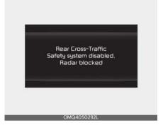
When the rear bumper around the rear corner radar or sensor is covered with foreign matters, such as snow or rain, or installing a trailer or carrier, it can reduce the detecting performance and temporarily limit or disable Rear Cross-Traffic Collision-Avoidance Assist.
