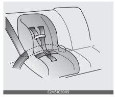
Since all passenger seat belts move freely under normal conditions and only lock under extreme or emergency conditions (emergency locking mode), you must manually pull the seat belt all the way out to shift the retractor to the
