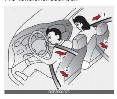
Your vehicle is equipped with driver's and front passenger's pre-tensioner seat belts (retractor pre-tensioner and EFD (Emergency Fastening Device). The pre-tensioner seat belts may be activated, when a frontal collision is severe enough, together with the air bags, depending on the crash severity, angle, speed and point of impact.
