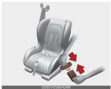
3. Pull the shoulder portion of the seat belt all the way out. When is fully extended, it will shift the retractor to the "Automatic Locking" (child restraint) mode.
