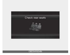
You can activate or deactivate the Rear Occupant Alert by selecting 'User Settings (LCD display) or Settings → Vehicle (Infotainment System screen) → Convenience → Rear Occupant Alert'.
