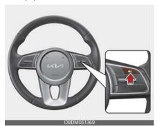
2. Press the Driving Assist button at the desired speed. The set speed and Cruise ( CRUISE) indicator will illuminate on the cluster.
