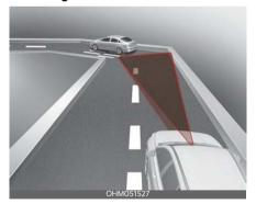
On curves, Smart Cruise Control may not detect a vehicle in the same lane, and may accelerate to the set speed. Also, the set speed may rapidly decrease when the vehicle ahead is detected suddenly.
