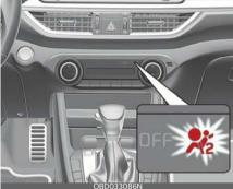
Your vehicle is equipped with an ODS in the front passenger's seat.
