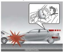
Front air bags may inflate in a frontal collision depending on the severity, speed and angles of impact.
