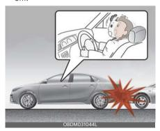
Front air bags may not inflate in side impact collisions, because occupants move to the direction of the collision. In side impacts, frontal air bag deployment would not provide additional occupant protection.
