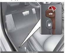
To open the trunk from inside the vehicle, pull the trunk release lever.
