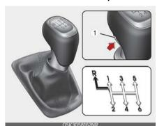
The shift lever can be moved without pushing the button (1).
