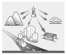
FM broadcasts are transmitted at high frequencies and do not bend to follow the earth's surface. Because of this, FM broadcasts generally begin to fade within short distances from the station. FM signals are easily affected by buildings, mountains, and obstructions. This
