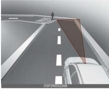
Forward Collision-Avoidance Assist may not detect other vehicle, pedestrian in front of you when driving on curved roads adversely affecting the performance of the sensors. This may result in no warning or no braking assist when necessary.
