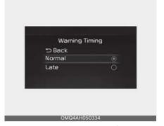
With the ignition switch or ENGINE START/STOP button in the ON position, select 'Driver Assistance → Warning Timing' from the 'User Settings (LCD display) or Setup → Vehicle (Infotainment System screen)' menu to change the initial warning activation time for Blind-Spot Collision-Avoidance Assist. When the vehicle is first delivered, Warning Timing is set to 'Normal'. If you change the Warning Timing, the Warning Timing of other Driver Assistance systems may change.
