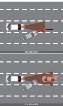
If a vehicle cuts in front of your vehicle, Leading Vehicle Departure Alert may not operate properly.
