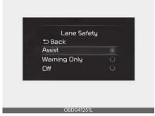
With the ignition switch or ENGINE START/STOP button in the ON position, select 'Driver Assistance → Lane Safety' from the 'User Settings (LCD display) or Setup → Vehicle (Infotainment System screen)' menu to set whether to use each function.
