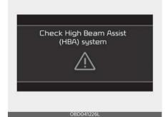
When High Beam Assist is not working properly, the warning message will iluminate for a few seconds. After the message disappears, the master warning light ( ( ) will illuminate.
