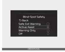
With the ignition switch or ENGINE START/STOP button in the ON position, select 'Driver Assistance → Blind-Spot Safety' from the 'User Settings (LCD display) or Setup → Vehicle (Infotainment System screen)' menu to set whether to use each function.
