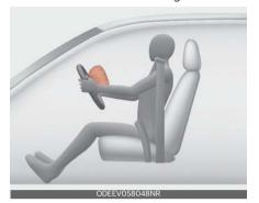
Upon deployment, tear seams molded directly into the pad covers will separate under pressure to allows full inflation of the air bags.
