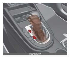
Whether the vehicle is stationary or in motion, manual mode is selected by pushing the shift lever from the D (Drive) position into the manual gate. To return to D (Drive) operation, push the shift lever into the main gate.
