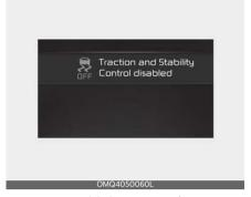
Press the ESC OFF button for more than 3 seconds, ESC OFF indicator light and message illuminates and ESC OFF warning chime will sound. The will not operate.
