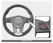
Press and hold the Driving Assist button on the steering wheel, at the
