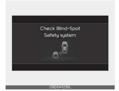
When Blind-Spot Collision Warning is not working properly, the 'Check Blind-Spot Safety system' warning message will
