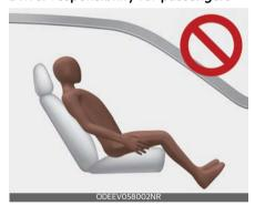
The driver must advise passengers to keep seatbacks in upright positions whenever the vehicle is in motion. If a seat is reclined during an accident, the restraint system's ability to restrain the passenger will be greatly reduced.
