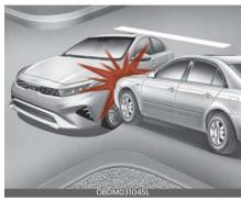
In an angled collision, the force of impact may direct the occupants in a direction where the air bags would not be able to provide any additional benefit, and the sensors may not deploy any air bags.
