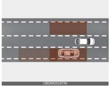
Blind-Spot Collision Warning helps detect and informs the driver that a vehicle is in the blind spot.
