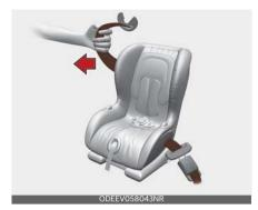
4. Slowly allow the shoulder portion of the seat belt to retract and listen for an audible "clicking" or "ratcheting" sound. This indicates that the retractor is in the "Automatic Locking" mode. If no distinct sound is heard, repeat steps 3 and 4.
