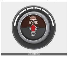
Press the "SYNC" button to adjust the driver and passenger side temperature equally.
