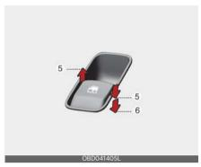
Pressing the power window switch momentarily to the second detent position (6) completely lowers the window even when the switch is released. To stop the window at the desired position while the window is in operation, pull up the switch momentarily.
