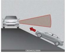
Rear Cross-Traffic Collision-Avoidance Assist may be limited when the vehicle is on a uphill or downhill slope, or near it, and may not detect the vehicle approaching from the left or right. If this occurs, the function may not warn the driver or control the brakes.
