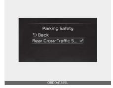
With the ignition switch or ENGINE START/STOP button in the ON position, select 'Driver Assistance → Parking Safety → Rear Cross-Traffic Safety' from the 'User Settings (LCD display) or Setup
