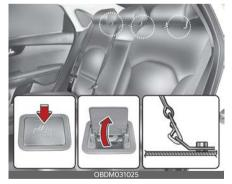
First secure the child restraint with the LATCH lower anchors or the seat belt. If the child restraint manufacturer recommends that the top tether strap be attached, attach and tighten the top
