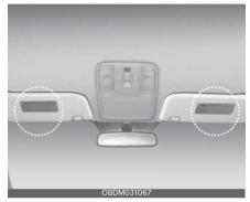
Air bag warning labels, required by the U.S. National Highway Traffic Safety Administration (NHTSA, U.S. only), are attached to the sun visor to alert the driver and passengers of potential risks of the air bag system.
