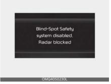
When the rear bumper around the rear corner radar or sensor is covered with foreign material, such as snow or rain, or installing a trailer or carrier, it can reduce the detecting performance and temporarily limit or disable Blind-Spot Collision-Avoidance Assist.
