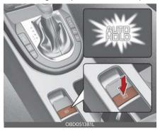
Before the Auto Hold will engage, the driver's door, trunk, and hood must be closed.
