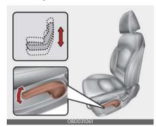
To change the height of the seat, push the lever up or down.
