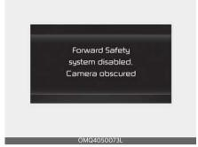
When the front windshield where the front view camera is located, is covered with foreign material, such as snow or rain, it can reduce the detecting performance and temporarily limit or disable Forward Collision-Avoidance Assist. If this occurs, the 'Forward Safety system disabled. Camera obscured' warning message will appear (turns off after a certain time), and the same and safety warning lights will illuminate on the cluster.
