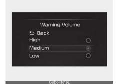
With the ignition switch or ENGINE START/STOP button in the ON position, select 'Driver Assistance → Warning Volume' from the 'User Settings (LCD display) or Setup → Vehicle (Infotainment System screen)' to change the Warning Volume to 'High', 'Medium', 'Low' for
