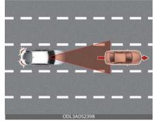
If the vehicle in front abruptly departs, Leading Vehicle Departure Alert may not operate properly.
