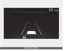
If the vehicle ahead or both lane markings are detected and your vehicle speed is below 110 mph (180 km/h), the green ( ) indicator light will illuminate on the cluster, and the function will help center the vehicle in the lane by controlling the steering wheel.
