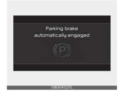
If the driver turns the engine off by mistake while Auto Hold (if equipped) is operating, EPB will be automatically applied. If the driver turns the engine off and pushes the EPB switch for 1 second, the EPB does not apply.
