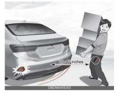
If you are positioned in the detecting area ( $20 \sim 40$  inches ( $50 \sim 100$  cm) behind the vehicle) carrying a smart key, the hazard warning lights will blink and the chime will sound to alert you the smart key has been detected and the trunk will open.
