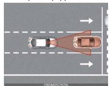
Forward Collision-Avoidance Assist is designed to help detect and monitor the vehicle ahead or help detect a pedestrian in the roadway and warn the driver that a collision is imminent with a warning message, audible warning and apply emergency braking.
