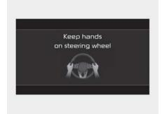
The hands-off warning appears when the function detects that the driver's hands are not on the steering wheel while Highway Driving Assist is in work.
