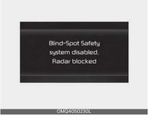
When the rear bumper around the rear corner radar or sensor is covered with foreign material, such as snow or rain, or installing a trailer or carrier, it can reduce the detecting performance and tempo-
