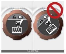
Make sure that the tiny protrusions inside the coolant cap are securely interlocked. 8
