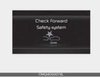
When Forward Collision-Avoidance Assist is not working properly, the 'Check Forward Safety system' warning message will appear (turns off after a certain time), and the and and armoning lights will illuminate on the cluster. In this case, have the vehicle inspected by an authorized Kia dealer.
