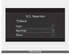
The sensitivity of set speed when following the front vehicle to maintain the set distance can be adjusted. With the ignition switch or ENGINE START/STOP button in the ON position, select 'Driver Assistance  $\rightarrow$  SCC Reaction' from the 'User Settings (LCD display) or Setup  $\rightarrow$  Vehicle (Infotainment System screen)' menu to set one of the three stages you prefer.
