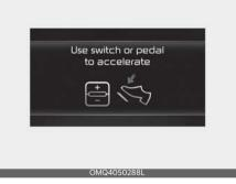
When Highway Driving Assist is operating, your vehicle will stop if the vehicle ahead of you stops. Also, if the vehicle ahead of you starts moving within 30 seconds after the stop, your vehicle will start as well. In addition, after the vehicle has stopped and 30 seconds have passed, the 'Use switch or pedal to accelerate' message will appear on the cluster. Depress the accelerator pedal or push the + switch, - switch or (| ) switch to start driving.
