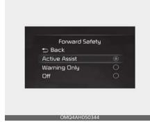
With the ignition switch or ENGINE START/STOP button in the ON position, select 'Driver Assistance → Forward Safety' from the 'User Settings (LCD display) or Setup → Vehicle (Infotainment System screen)' menu to set whether to use each function.
