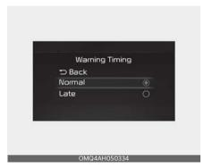
With the ignition switch or ENGINE START/STOP button in the ON position, select 'Driver Assistance → Warning Timing' from the 'User Settings (LCD display) or Setup → Vehicle (Infotainment System screen)' to change the initial warning activation time for Rear Cross-Traffic Collision Warning.
