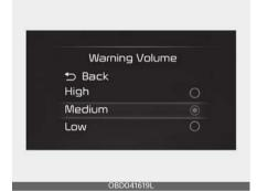
With the ignition switch or ENGINE START/STOP button in the ON position, select 'Driver Assistance → Warning Volume' from the 'User Settings (LCD display) or Setup → Vehicle (Infotainment System screen)' menu to change the Warning Volume to 'High', 'Medium' or 'Low' for Rear Cross-Traffic Collision-Avoidance Assist.
