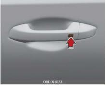
Pressing the button of the front driver side door handles with all doors (and trunk) closed and any door unlocked, locks all the doors (and trunk). If all doors, trunk and hood are closed, the hazard warning lights will blink once and the chime will sound once to indicate the vehicle is locked.
