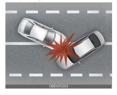
Just before an impact, drivers may brake heavily. Such heavy braking may lowers the front portion of the vehicle causing it to "ride" under a vehicle with a higher ground clearance. Air bags may not inflate in this "under-ride" situation because deceleration forces that are detected by sensors may be significantly reduced by such "under-ride" collisions.
