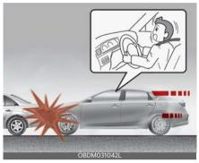
Air bags are not designed to inflate in rear collisions, because occupants are moved backward by the force of the impact. In this case, inflated air bags would not provide any additional benefit.
