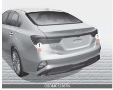
[1]: Rear corner radar Refer to the picture above for the detailed location of the detecting sensor.
