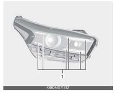
If the position lamp/daytime running lamp (LED) (1) does not operate, have the vehicle checked by an authorized Kia dealer.
