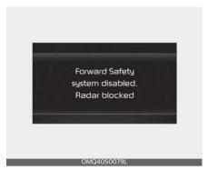
When the front windshield where the front view camera is located, front radar cover or sensor is covered with foreign material such as snow or rain, it can reduce the detecting performance and temporarily limit or disable Forward Collision-Avoidance Assist. If this occurs the 'Forward Safety system disabled. Radar blocked' warning message will appear (turns off after a certain time), and the
