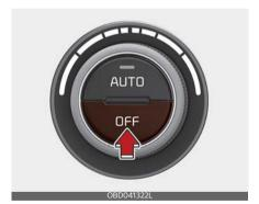
Press the OFF button to turn off the air climate control system. You can still operate the mode and air intake buttons if the ignition switch or the ENGINE START/STOP button is in the ON position.
