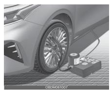
With the TMK you can continue to drive even after experiencing a tire puncture. The system compressor and sealing compound effectively seal most punctures in a passenger car tire caused by nails or similar objects, and reinflate the tire.
