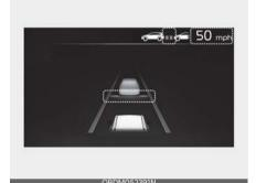
If you want to speed up temporarily when Smart Cruise Control is on, depress the accelerator pedal for a certain amount. While depressing the accelerator pedal for a certain amount, the set speed, distance level and target distance will blink on the cluster. However, if the accelerator pedal is insufficiently depressed, the vehicle may slow down.
