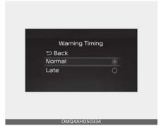
With the ignition switch or ENGINE START/STOP button in the ON position, select 'Driver Assistance → Warning Timing' from the 'User Settings (LCD display) or Setup → Vehicle (Infotainment System screen)' menu to change the initial warning activation time for Driver Attention Warning. When the vehicle is first delivered, Warning Timing is set to 'Normal'. If you change the Warning Timing, the Warning Timing of other Driver Assistance systems may change.
