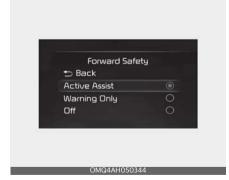
With the ignition switch or ENGINE START/STOP button in the ON position, select 'Driver Assistance → Forward Safety' from the 'User Settings (LCD display) or Setup → Vehicle (Infotainment
