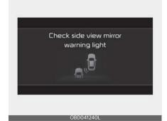
When the warning light on the side view mirror (outside mirror) is not working properly, the 'Check side view mirror warning light' warning message will
