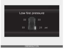
When the TPMS warning indicators are illuminated and warning message displayed on the instrument cluster LCD display, one or more of your tires is significantly under-inflated.
