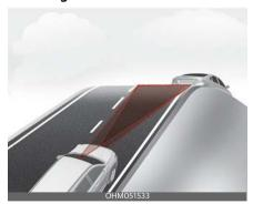
During uphill or downhill driving, Smart Cruise Control may not detect a moving vehicle in your lane, and cause your vehicle to accelerate to the set speed. Also, the set speed will rapidly decrease when the vehicle ahead is detected suddenly.
