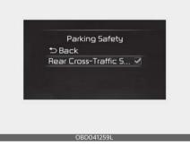
With the ignition switch or ENGINE START/STOP button in the ON position, select 'Driver Assistance → Parking Safety → Rear Cross-Traffic Safety' from the 'User Settings (LCD display) or Setup → Vehicle (Infotainment System screen)' menu to turn on Rear Cross-Traffic Collision Warning and deselect to turn off the function.
