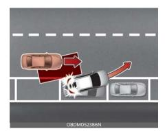
When changing lanes by detecting the lane ahead, if Blind-Spot Collision-Avoidance Assist judges that there is a collision risk with an approaching vehicle in the blind spot, it can help avoid collisions by applying the differential brake.
