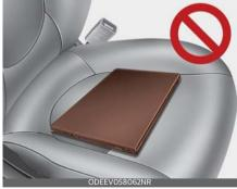
Wet Passenger Seat Do not spill liquid in the passenger seat. Spilled liquid on the passenger seat may cause the air bag warning light to illuminate or malfunction. If any liquid is spilled, make sure the seat has been completely dried before driving the vehicle.
