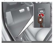
The fuel-filler door must be opened from inside the vehicle by pulling up on the fuel-filler door opener located on the front floor area on the driver's seat. If the fuel filler door does not open because ice has formed around it, tap lightly or push on the door to break the ice and release the door. Do not pry on the door. If necessary, spray an approved de-icer fluid around the door. Do not use radiator anti-freeze. You can also move the vehicle to a warm place and allow the ice to melt.
