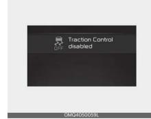
Press the ESC OFF button quickly (ESC OFF indicator light and message illuminates). The traction control function part of ESC will not operate but the brake control function will operates.
