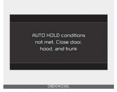
Press the [AUTO HOLD] button after closing the driver's door, hood and trunk.
