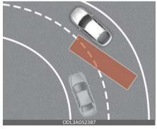
Blind-Spot Collision Warning may not operate properly when driving on a curved road. The function may not detect the vehicle in the next lane.
