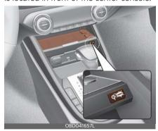
Firmly close all doors, and ensure the ignition switch or ENGINE START/STOP button is ON. To start wireless charging, place the smart phone equipped with wireless charging function on the wireless charging pad.
