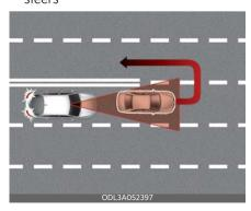
If the vehicle in front makes a sharp turn, such as to turn left or right or make a Uturn, etc., Leading Vehicle Departure Alert may not operate properly.
