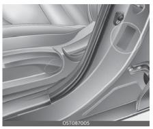
The vehicle certification label attached on the driver's (or front passenger's) side center pillar gives the VIN.
