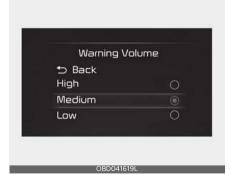
With the ignition switch or ENGINE START/STOP button in the ON position, select 'Driver Assistance → Warning Volume' from the 'User Settings (LCD dis-
