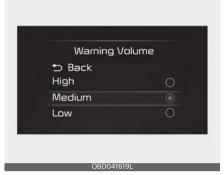
With the ignition switch or ENGINE-START/STOP button in the ON position, select 'Driver Assistance → Warning Volume' from the 'User Settings (LCD display) or Setup → Vehicle (Infotainment System screen)' to change the Warning Volume to 'High', 'Medium', 'Low' for Rear Cross-Traffic Collision Warning. If you change the Warning Volume, the Warning Volume of other Driver Assistance systems may change.
