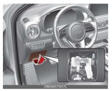
3. Pull the suspected fuse straight out.
