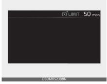
The set speed limit will be displayed on the cluster. If you would like to drive over the preset speed limit, depress the accelerator pedal beyond the pressure point to activate the kickdown function.
