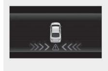
To warn the driver of an approaching vehicle from the rear left/right side of your vehicle, the side view mirror will blink and a warning will appear on the cluster. At the same time, an audible warning will sound. If Rear View Monitor is operating, a warning will also appear on the infotainment screen.
