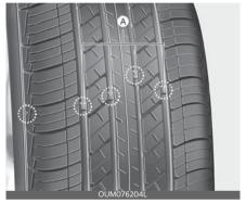
This shows there is less than 1/16 inch (1.6 mm) of tread left on the tire. Replace the tire when this happens.
