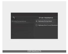
With the ignition switch or ENGINE START/STOP button in the ON position, select 'Driver Assistance → Driving Convenience' from the Setup menu to set whether to use each function.
