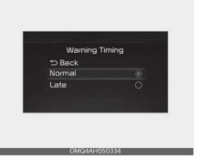
With the ignition switch or ENGINE START/STOP button in the ON position, select 'Driver Assistance → Warning Timing' from the 'User Settings (LCD dis-
