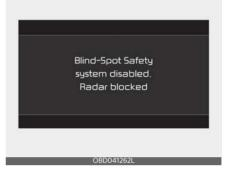
When the rear bumper around the rear corner radar or sensor is covered with foreign matters, such as snow or rain, or installing a trailer or carrier, it can reduce the detecting performance and temporarily limit or disable Safe Exit Warning. If this occurs, the 'Blind-Spot Safety system disabled. Radar blocked' warning message will appear on the cluster. Safe Exit Warning will operate properly when such foreign matters or trailer, etc., is removed, and then the engine is restarted.
