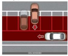
• When the vehicle is parked rearward Rear Cross-Traffic Collision-Avoidance Assist may detect vehicles passing by behind you when parking backwards into a parking space. If this occurs, the function may unnecessarily warn the driver and control the brake.
