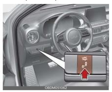
If you press the Blind-Spot Safety button while 'Warning Only' or 'Active Assist' selected the indicator on the button extinguishes and the function deactivates, and if you press the Blind-Spot Safety button while the function is off, indicator on the button illuminates and the function will operate as before it was turned off.
