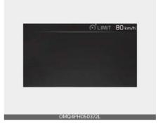
The set speed limit will be displayed on the cluster. If you would like to drive over the preset speed limit, depress the accelerator pedal beyond the pressure point to activate the kickdown mechanism.
