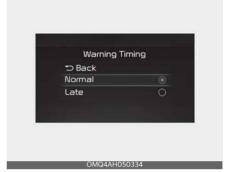
With the ignition switch or ENGINE START/STOP button in the ON position, select 'Driver Assistance → Warning Timing' from the 'User Settings (LCD display) or Setup → Vehicle (Infotainment System screen)' menu to change the initial warning activation time for Forward Collision-Avoidance Assist.
