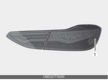
If the side marker (LED) (1) does not operate, have the vehicle checked by an authorized Kia dealer. The LED lamp cannot be replaced as a single component because it is an integrated unit. The LED lamp has to be replaced with the unit. A skilled technician should check or repair the side marker (LED), for it may damage related parts of the vehicle.
