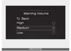
With the ignition switch or ENGINE START/STOP button in the ON position, and select 'User Settings (LCD display) or Settings → Vehicle (Infotainment System screen) → Driver Assistance → Warning Volume' to change the Warning Volume to 'High', 'Medium' or 'Low' for Safe Exit Warning.
