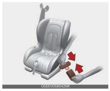
Pull the shoulder portion of the seat belt all the way out. When the shoulder portion of the seat belt is fully extended, it will shift the retractor to the "Automatic Locking" (child restraint) mode.
