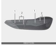
If the stop (1) and tail (2) lamp (LED), does not operate, have the vehicle checked by an authorized Kia dealer.
