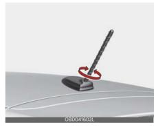
Your car uses a micro pole antenna to receive broadcast signal. The antenna pole is a removable type.
