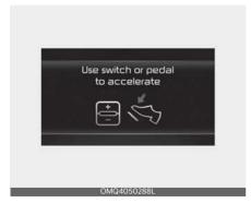
In traffic, your vehicle will stop if the vehicle ahead of you stops. Also, if the vehicle ahead of you starts moving, your vehicle will start as well. In addition, after
