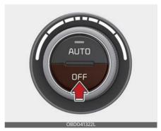
Press the OFF button to turn off the air climate control system. However, you can still operate the mode and air intake buttons as long as the ignition switch or the ENGINE START/STOP button is in the ON position.
