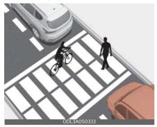
If there is a pedestrian or cyclist in between you and the vehicle in front, Leading Vehicle Departure Alert may not operate properly. · When in a parking lot
