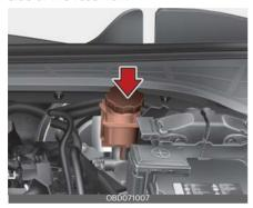
Before removing the reservoir cap and adding brake/clutch fluid, clean the area around the reservoir cap thoroughly to prevent brake/clutch fluid contamination.
