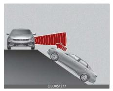
• When the vehicle is on or near a slope Rear Cross-Traffic Collision-Avoidance Assist may be limited when the vehicle is on a uphill or downhill slope, or near it, and may not detect the vehicle approaching from the left or right. If this occurs, the function may not warn the driver or control the brakes when necessary.
