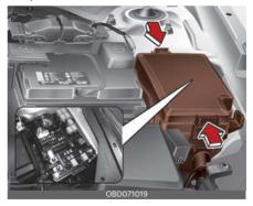
3. Check the removed fuse; replace it if it is blown. To remove or insert the fuse, use the fuse puller in the engine compartment fuse panel.
