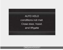
At this moment, press the Auto Hold button after closing the driver's door, engine hood and liftgate.
