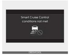
If the Driving Assist button, +, - or | switch is pushed when Smart Cruise Control's operating conditions are not satisfied, the 'Smart Cruise Control conditions not met' will appear on the cluster, and an audible warning will sound.
