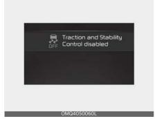
Press the ESC OFF button for more than 3 seconds. ESC OFF indicator light and message illuminates and ESC OFF warning chime will sound. At this state, the engine control function and brake control function does not operate. In other words, the vehicle
