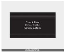
When Rear Cross-Traffic Collision-Avoidance Assist is not working properly, the 'Check Rear Cross-Traffic Safety system' warning message will appear (turns off after a certain time). and the / warning light will illuminate on the cluster. In this case, have your vehicle inspected by an authorized Kia dealer.
