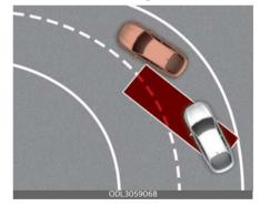
Blind-Spot Collision-Avoidance Assist may not operate properly when driving on the curved road. The function may recognize the vehicle in the same lane. Always pay attention to road and driving conditions while driving.
