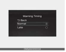
With the ignition switch or ENGINE START/STOP button in the ON position, select 'Driver Assistance → Warning
