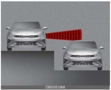
Blind-Spot Collision-Avoidance assist may not operate properly when driving where the heights of the lanes are different. The function may not detect the vehicle on a road with different lane heights (underpass joining section, grade separated intersections, etc.). Always pay attention to road and driving conditions while driving.
