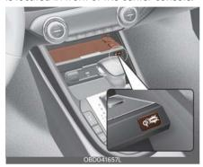
Firmly close all doors, and the ignition switch or ENGINE START/STOP button is ON. To start wireless charging, place the smart phone equipped with wireless charging function on the wireless charging pad.
