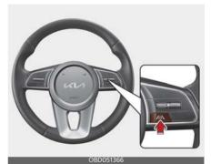
With the ignition switch or ENGINE START/STOP button in the ON position, press and hold the Lane Driving Assist button ( ) located on the steering wheel to turn off Lane Keeping Assist. Press and hold the button again to turn on the function.
