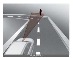
Forward Collision-Avoidance Assist may detect a vehicle or pedestrian in the next lane or outside the lane when driving on a curved road.
