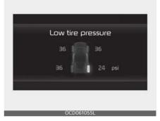
When the tire pressure monitoring system warning indicators are illuminated and warning message displayed on the cluster LCD display, one or more of your tires is significantly under-inflated.
