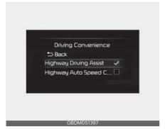
With the ignition switch or ENGINE START/STOP button in the ON position, select 'Driver Assistance → Driving Convenience' from the 'User Settings (LCD display) or Setup → Vehicle (Infotainment System screen)' menu to set whether to use each function.
