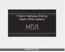
When Highway Driving Assist is not working properly, the 'Check Highway Driving Assist (HDA) system' warning message will appear, and the warning light will illuminate on the cluster. Have your vehicle inspected by an authorized Kia dealer.
