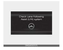
When Lane Following Assist is not working properly, the 'Check Lane Following Assist (LFA) system' warning message will appear on the cluster (turns off after a certain time) and the \( \bigcap \) warning light will illuminate. In this case, have the function checked by an authorized Kia dealer
