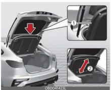
Use the cover to hide items stored in the cargo area. The cargo area cover will be lifted when the liftgate is opened. Disconnect the strap (1) from holder if you want to return the cover to original position. To remove the cargo area cover completely, lift the cover to a 43- degree angle and pull it out to the full (2). For installation of the cover, reverse the removal procedure.
