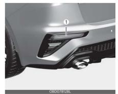
If the rear turn signal lamp (1) does not operate, have the vehicle checked by an authorized Kia dealer.
