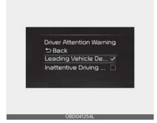
If 'Leading Vehicle Departure Alert' is selected, the function will inform the driver when a detected vehicle in front departs from a stop.
