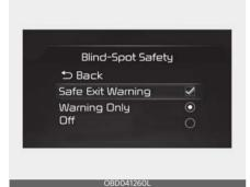
With the ignition switch or the ENGINE START/STOP button in the ON position, and select 'User Settings (LCD display) or Settings → Vehicle (Infotainment System screen) → Driver Assistance → Blind-Spot Safety → Safe Exit Warning' to turn on Safe Exit Warning and deselect to turn off the function.
