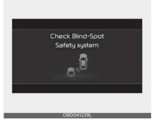
When Safe Exit Warning is not working properly, the 'Check Blind-Spot Safety system' warning message will appear on the cluster for several seconds, and the master ( ) warning light will illuminate on the cluster. In this case, have the vehicle inspected by an authorized Kia dealer.
