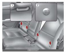
The LATCH anchors are located between the seatback and the seat cushion of the rear seat left and right outboard seating positions.
