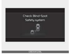
When Blind-Spot Collision-Avoidance Assist is not working properly, the 'Check Blind-Spot Safety system' warning message will appear (turns off after a certain time), and \( \bigcap \) warning light will illuminate on the cluster. In this case, have your vehicle inspected by an authorized Kia dealer.
