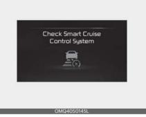
When Smart Cruise Control is not working properly, the 'Check Smart Cruise Control system' warning message will appear (turns off after a certain time), and the \( \frac{1}{2} \) warning light will illuminate on the cluster. In this case, take your vehicle to an authorized Kia dealer and have the function checked.
