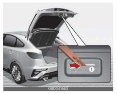
Your vehicle is equipped with the emergency liftgate safety release lever located on the bottom of the liftgate. When someone is inadvertently locked in the luggage compartment.
