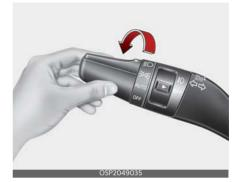
When the light switch is in the head light position, The head, tail, position, license and instrument panel lights will turn ON.
