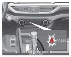
As a reminder to the front passenger, the front passenger's seat belt warning lights will illuminate for approximately 6 seconds each time you turn the ignition switch or the ENGINE START/STOP button in ON regardless of belt fastening. If the front passenger continue not to fasten the seat belt and drive below 20 km/h (12 mph), the warning light will stay illuminated.
