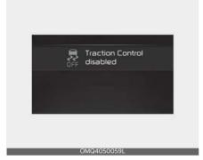
Press the ESC OFF button shortly (ESC OFF indicator light and message illuminates). At this state, the engine control function does not operate. In other words, the traction control function does not operate but only the brake control function operates.
