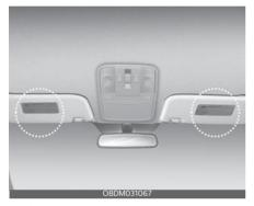
Air bag warning labels, some required by the Canada Motor Vehicle Safety Standard (CMVSS), are attached to the sun visor to alert the driver and passengers of potential risks of the air bag system.
