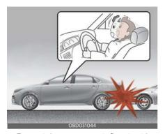
Front air bags may not inflate in side impact collisions, because occupants move to the direction of the collision, and thus in side impacts, frontal air bag deployment would not provide additional occupant protection.
