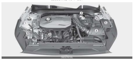
\* The actual engine room in the vehicle may differ from the illustration. 1. Engine coolant reservoir 7-23 2. Engine oil filler cap 7-21 3. Brake / clutch fluid reservoir 7-26 4. Air cleaner 7-28 5. Fuse box 7-54 6. Negative battery terminal 7-34 7-34 7. Positive battery terminal 8. Engine oil dipstick 7-21 7-23 9. Radiator cap 10. Windshield washer fluid reservoir 7-27
