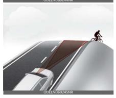
Forward Collision-Avoidance Assist may not detect other vehicle, pedestrian or cyclist in front while driving uphill or downhill and this may result in no warning, or braking assist when necessary.
