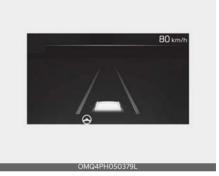
If the vehicle ahead or both lane markings are detected and your vehicle speed is below 180 km/h (110 mph), the green ( ) indicator light will illuminate on the cluster, and the function will help center the vehicle in the lane by controlling the steering wheel.
