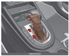
Whether the vehicle is stationary or in motion, manual mode is selected by pushing the shift lever from the D (Drive) position into the manual gate. To return to D (Drive) range operation, push the shift lever back into the main gate. Manual mode manages the driving dynamics by automatically adjusting the steering effort, and the engine and
