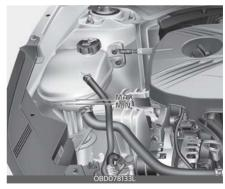
Check the condition and connections of all cooling system hoses and heater hoses. Replace any swollen or deteriorated hoses.
