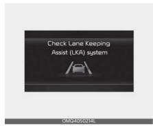
When Lane Keeping Assist is not working properly, the 'Check Lane Keeping Assist (LKA) system', warning message will appear and the yellow ( ) indicator light will illuminate on the cluster. In this case, have the function inspected by an authorized Kia dealer.
