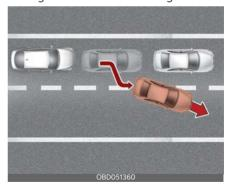
When a vehicle in front of you merges out of the lane, Smart Cruise Control may not immediately detect the new vehicle that is now in front of you. Always pay attention to road and driving conditions while driving.
