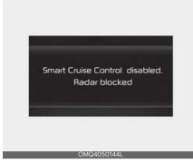
When the front radar cover or sensor is covered with snow, rain, or foreign matters, it can reduce the detecting performance and temporarily limit or disable Smart Cruise Control.
