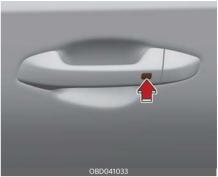
Pressing the button of the front driver side door handles with all doors (and liftgate) closed and any door unlocked, locks all the doors (and liftgate). If all doors (and liftgate) and engine hood are closed, the hazard warning lights will blink once and the chime will sound once to indicate the vehicle is locked.
