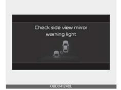
When the outside rear view mirror warning light is not working properly, the 'Check side view mirror warning light' warning message will appear on the cluster for several seconds, and the master ( ) warning light will appear on
