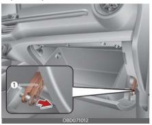
Remove the climate control air filter cover while pressing the lock on the left side of the cover.
