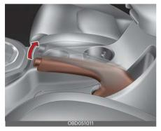
Check the stroke of the parking brake by counting the number of "clicks" heard while fully applying it from the released position. Also, the parking brake alone should securely hold the vehicle on a fairly steep grade. If the stroke is more or less than specified, have the parking brake adjusted by an authorized Kia dealer.
