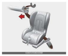
Slowly allow the shoulder portion of the seat belt to retract and listen for an audible "clicking" or "ratcheting" sound. This indicates that the retractor is in the "Automatic Locking" mode. If no distinct sound is heard, repeat steps 3 and 4.
