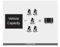
Item Description Total Vehicle Capacity 385 ka Α (849 lbs) Weight Subtract Occu-365 kg В pant Weight 73 kg (805 lbs)  $(161 lbs) \times 5$ Available Cargo 20 kg (44 C and Luggage lbs) weight
