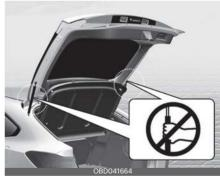
Do not grasp the part supporting the liftgate (gas lifter), as this may cause serious injury.
