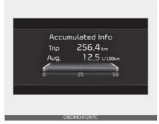
The trip computer mode displays information related to vehicle driving parameters including Accumulated info, Driving information, and so on.
