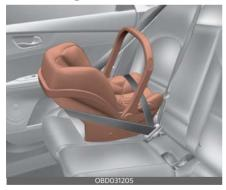
A rear-facing child seat provides restraint with the seating surface against the back of the child. The harness system holds the child in place, and in an accident, acts to keep the child positioned in the seat and reduces the stress. to the neck and spinal cord.
