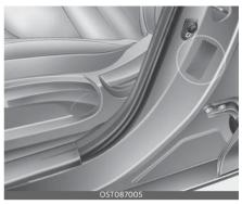
The vehicle certification label attached on the driver's (or front passenger's) side center pillar gives the vehicle identification number (VIN).
