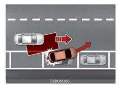
When changing lanes by detecting the lane ahead, if Blind-Spot Collision-Avoidance Assist judges that there is a collision risk with an approaching vehicle in the blind spot, it can help avoid collisions by applying the differential brake.
