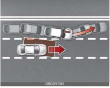
When you are driving forward out of a parking space, if Blind-Spot Collision-Avoidance Assist judges that there is a collision risk with an approaching vehicle in the blind spot, it can help avoid collisions by applying the brake.
