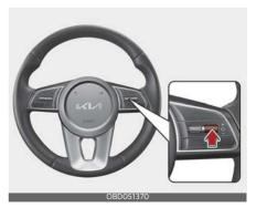
Push the | switch to temporarily pause the set speed limit. The set speed limit will turn off but the Speed Limit indicator will stay on.
