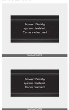
When the front windshield where the front view camera is located, front radar cover or sensor is covered with foreign material such as snow or rain, it can reduce the detecting performance and temporarily limit or disable Forward Collision-Avoidance Assist. If this occurs the 'Forward Safety system disabled. Radar blocked' warning message will appear (turns off after a certain time), and the
