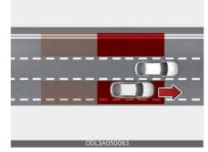
Blind-Spot Collision-Avoidance Assist helps detect and informs the driver that a vehicle is in the blind spot.
