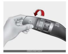
The parking light and headlight will be turn ON or OFF automatically depending on the amount of daylight as measured by the ambient light sensor on the center dash when the parking brake is not engaged and shift lever is not in P(Park). The parking light and headlight will be turned OFF when the vehicle speed is less than 5 km/h and parking brake is engaged or shift lever is in P(Park).
