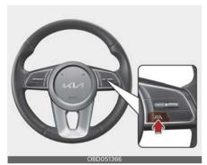
With the ignition switch or ENGINE START/STOP button in the ON position, press the Lane Driving Assist button located on the steering wheel to turn on Lane Following Assist. The white or green ((A)) indicator light will illuminate on the cluster.
