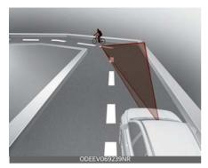
The front view camera or radar sensor recognition function may not detect the vehicle, pedestrian or cyclist traveling in front on a curved road. Always pay attention to road and driving conditions, and if necessary, depress the brake pedal to reduce your driving speed in order to maintain a safe distance.
