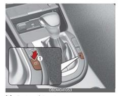
[1]: Parking/View buttonPress the Parking/View button to turn on Rear View Monitor.
