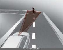
Forward Collision-Avoidance Assist may detect a vehicle or pedestrian in the next lane or outside the lane when driving on a curved road. If this occurs, the unnecessarily alarm the driver and apply the brake. Always check the traffic conditions around the vehicle.
