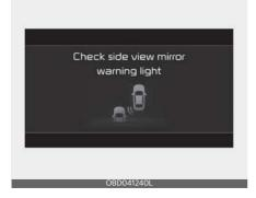
When the warning light on the side view mirror is not working properly, the 'Check side view mirror warning light' warning message will appear (turns off after a certain time), and warning light will illuminate on the cluster. In this case, have your vehicle inspected by an authorized Kia dealer.
