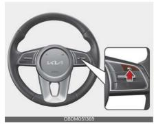
2. Press the Driving Assist button at the desired speed. The set speed and Cruise ( CALLISE) indicator will illuminate on the cluster.
