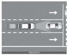
Forward Collision-Avoidance Assist is designed to help detect and monitor the vehicle ahead or help detect a pedestrian in the roadway and warn the driver that a collision is imminent with a warning message, audible warning and apply emergency braking.
