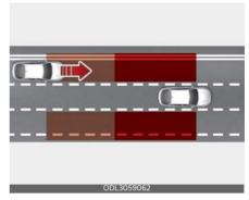
Blind-Spot Collision-Avoidance Assist helps detect and informs the driver that a vehicle is approaching at high speed from the blind spot area.
