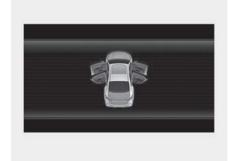
This warning is displayed indicating which door, or the hood, or the liftgate is open.
