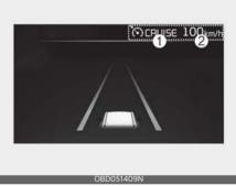
You can see the status of the Smart Cruise Control operation in the Driving Assist view on the cluster. Refer to "Instrument cluster" on page 4-51.
