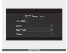
The sensitivity of vehicle speed when following the front vehicle to maintain the set distance can be adjusted. With the ignition switch or ENGINE START/STOP button in the ON position, select 'Driver Assistance → SCC Reaction' from the 'User Settings (LCD display) or Setup → Vehicle (Infotainment System screen)' menu to set one of the three stages you prefer.
