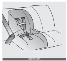
Since all passenger seat belts move freely under normal conditions and only lock under extreme or emergency conditions (emergency locking mode), you must manually pull the seat belt all the way out to shift the retractor to the "Automatic Locking" mode to secure a child restraint.
