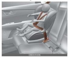
A forward-facing child seat provides restraint for the child's body with a harness. Keep children in a forwardfacing child seat with a harness until they reach the top height or weight limit allowed by your child restraint's manufacturer.
