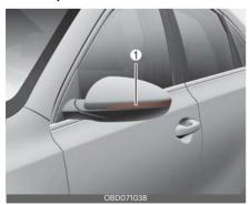
If the side repeater lamp (LED) (1) does not operate, have the vehicle checked by an authorized Kia dealer. The LED lamp cannot be replaced as a single component because it is an integrated unit. The LED lamp has to be replaced with the unit. A skilled technician should check or repair the side repeater lamp (LED), for it may damage related parts of the vehicle.
