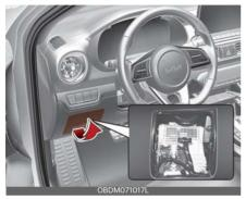
3. Pull the suspected fuse straight out. Use the removal tool provided on the engine fuse panel cover.
