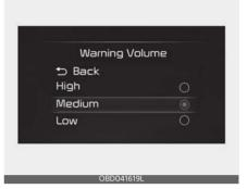
With the ignition switch or ENGINE START/STOP button in the ON position, select 'Driver Assistance → Warning Volume' from the 'User Settings (LCD display) or Setup → Vehicle (Infotainment System screen)' to change the Warning Volume to 'High', 'Medium', 'Low' for Highway Driving Assist.
