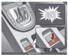
Before the Auto Hold will engage, the driver's door, liftgate, and engine hood must be closed.
