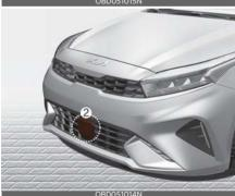
[1]: Front view camera, [2]: Front radar The front view camera and front radar are used as a detecting sensor to detect vehicles in front. Refer to the picture above for the detailed location of the detecting sensor.
