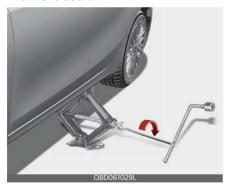
9. Loosen the wheel nuts and remove them with your fingers. Slide the wheel off the studs and lay it flat so it cannot roll away. To put the wheel on the hub, pick up the spare tire, line up the holes with the studs and slide the wheel onto them.
