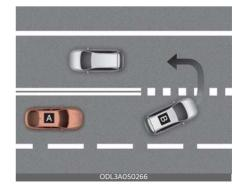
[A]: Your vehicle, [B]: Front vehicle If the vehicle in front makes a sharp turn, such as to turn left or right or make a Uturn, etc., Leading Vehicle Departure Alert may not operate properly.
