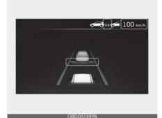
If you want to speed up temporarily when Smart Cruise Control is on, depress the accelerator pedal for a certain amount. While depressing the accelerator pedal for a certain amount, the set speed, distance level and target distance will blink on the cluster. However, if the accelerator pedal is insufficiently depressed, the vehicle may slow down.
