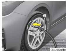
7. Unscrew the valve cap from the valve of the defective wheel and screw filling hose (3) of the sealant bottle onto the valve.
