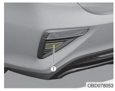
If the back up lamp (1) does not operate, have the vehicle checked by an authorized Kia dealer.
