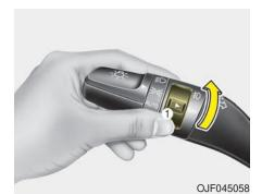
Fog lights are used to provide improved visibility when visibility is poor due to fog, rain or snow, etc. The fog lights will turn on when the fog light switch (1) is turned to the on position after the headlights are turned on.
