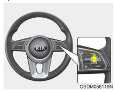
Press the CRUISE button, to turn the system on. The CRUISE indicator in the instrument cluster will illuminate. Accelerate to the desired speed.The smart cruise control speed
