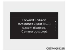
When the sensor is covered or the sensor lens is dirty with foreign substances, such as snow or rain, the FCA system may not be able to detect vehicles. In this case, a warning message ("Forward Collision-Avoidance Assist (FCA) system disabled. Camera blocked") will appear to notify the driver. Remove the foreign substances to allow the FCA system to function property.
