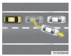
When vehicles are at a standstill and the vehicle in front of you changes to the next lane, be careful when your vehicle starts to move because it may not immediately recognize the stopped vehicle in front of you.
