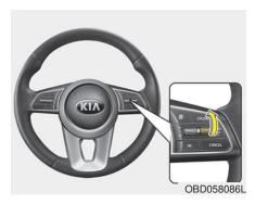
If any method other than the CRUISE ON-OFF switch was used to cancel cruising speed and the system is still activated, the most recent set speed will automatically resume when you move the lever up.
