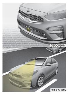
By detecting the vehicle or pedestrian ahead the vehicle, the sensor helps to operate the Forward Collision-Avoidance Assist when the vehicle is at risk of a collision.
