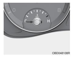
This gauge shows the temperature of the engine coolant when the ignition switch is ON.
