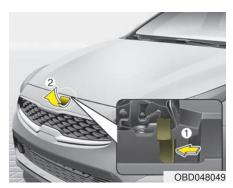
2. Go to the front of the vehicle, raise the hood slightly, push the secondary latch (1) inside of the hood center and lift the hood (2).
