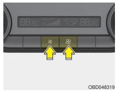
The fan speed can be set to the desired speed by operating the fan speed control button.
