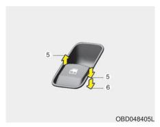
Pressing the power window switch momentarily to the second detent position (6) completely lowers the driver's window even when the switch is released. To stop the window at the desired position while the window is in operation, briefly pull up the switch to the opposite direction of the window movement.
