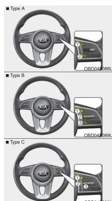
The LCD window modes can be changed by using the control buttons on the steering wheel.
