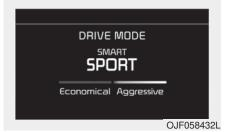
SMART mode selects the **SMART** proper driving mode among ECO, NORMAL and SPORT by judging the driver's driving habits (i.e. mild or dynamic) from the brake pedal depression or the steering wheel operation.
