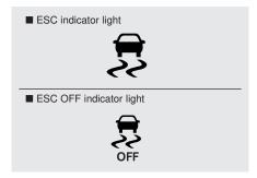
When ignition switch is turned to ON, the indicator light illuminates, then goes off if the ESC system is operating normally.
