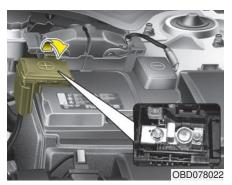
If the battery fuse is blown, it must be removed as follows:
