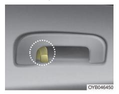
The clothes hanger is located on the roof of rear seats.
