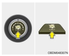
The air intake control is used to select the outside (fresh) air position or recirculated air position.
