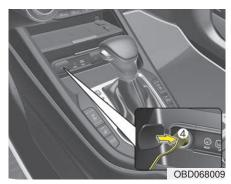
8. Connect between compressor and the vehicle power outlet using the cable and connectors (4).
