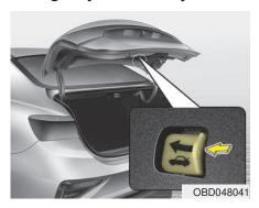
Your vehicle is equipped with an emergency trunk release lever located inside the trunk. If someone is inadvertently locked in the trunk, moving the handle in the direction of the arrow will release the trunk latch mechanism and open the trunk.
