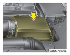
The air filter must be replaced when necessary, and should not be washed.
