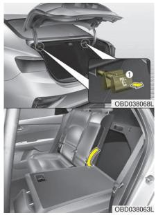
3. Pull out the seatback locking knob(1) in the trunk, then fold the seat toward the front of the vehicle.
