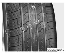
If the tire is worn evenly, a tread wear Indicator (A) will appear as a solid band across the tread. This shows there is less than 1.6 mm (1/16 inch) of tread left on the tire. Replace the tire when this happens.
