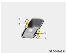
Pressing or pulling up the power window switch momentarily to the second detent position (6) completely lowers or lifts the window even when the switch is released. To stop the window at the desired position while the window is in operation, pull up or press and release the switch to the opposite direction of the movement. If the power window is not operated correctly, the automatic power window system must be reset as follows:
