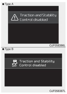
At this state, the car stability control function does not operate any more.
