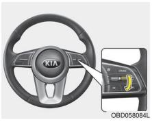
Move the lever down (to SET-), and release it at the desired speed. The SET speed on the LCD screen will appear. Release the accelerator at the same time. The desired speed will automatically be maintained.
