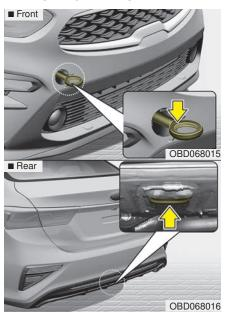
If towing is necessary, we recommend you to have it done by an authorized Kia dealer or a commercial tow truck service. If towing service is not available in an emergency, your vehicle may be temporarily towed using a cable or chain secured to the emergency towing hook under the front (or rear) of the vehicle. Use extreme caution when towing the vehicle. A driver must be in the vehicle to steer it and operate the brakes.
