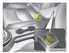
The USB car charger allows drivers to charge their digital devices like smartphone, and PC tablets. Connect the device to the USB port using a manufacturer certified cable to begin charging.
