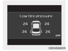
When the tire pressure monitoring system warning indicators are illuminated, one or more of your tires is significantly under-inflated.
