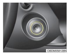
Whenever a front door is opened, the ignition switch will illuminate for your convenience, provided the ignition switch is not in the ON position. The light will go off immediately when the ignition switch is turned on. It will also go off after about 30 seconds when the door is closed.
