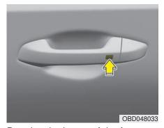
Pressing the button of the front outside door handles with all doors closed and any door unlocked, locks all the doors (and hood, trunk).
