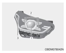
If the Low/High beam lamp(1), Day time running lamp/Position lamp(2), side marker(3) do not operate, have the vehicle checked by an authorized Kia dealer.
