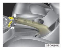
To release the parking brake, first apply the foot brake and pull up the parking brake lever slightly. Secondly depress the release button (1) and lower the parking brake lever (2) while holding the button.
