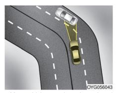
Your vehicle speed can be reduced due to a vehicle in the adjacent lane. Adjust your vehicle speed by depressing the brake pedal according to the road and driving conditions ahead. Apply the accelerator pedal and select the appropriate set speed. Check to be sure that the road conditions permit safe operation of the smart cruise control.
