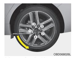
6. Loosen the wheel lug nuts counterclockwise one turn each, but do not remove any nut until the tire has been raised off the ground.
