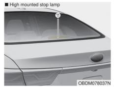
(11) High mounted stop lamp (Bulb or LED type)
