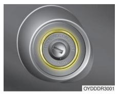
Whenever a front door is opened, the ignition switch will illuminate for your convenience, provided the ignition switch is not in the ON position. The light will go off immediately when the ignition switch is turned on. It will also go off after about 30 seconds after the door is closed.
