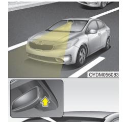
The Lane Keeping Assist System detects lane markers on the road, and assists the driver's steering to help keep the vehicle between lanes.
