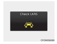
The LKAS fail indicator (yellow) will illuminate with an audible warning if the LKAS is not working properly. We recommend that you contact an authorized Kia dealer.
