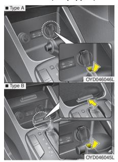
The power outlet is designed to provide power for mobile telephones or other devices designed to operate with vehicle electrical systems. The devices should draw less than 12V, 15A with the engine running.
