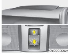
To open the sunroof, push the sunroof control lever upward until the sunroof moves to the desired position.
