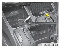
If your vehicle has an aux and/or USB(universal serial bus) port or iPod® port, you can use an aux port to connect audio devices and an USB port to plug in an USB and also an iPod® port to plug in an iPod®.
