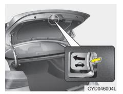
Your vehicle is equipped with an emergency trunk release lever located inside the trunk. If someone is inadvertently locked in the trunk, moving the handle in the direction of the arrow will release the trunk latch mechanism and open the.
