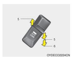
Pressing the power window switch momentarily to the second detent position (6) completely lowers the driver's window even when the switch is released. To stop the window at the desired position while the window is in operation, momentarily pull up the switch to the opposite direction of the window movement.
