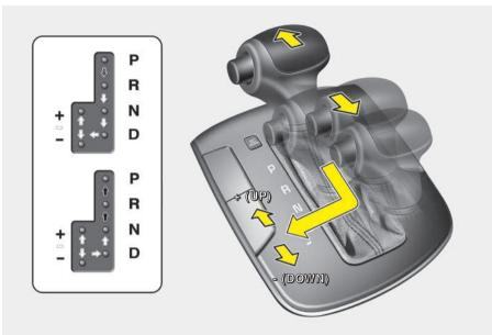
Depress the brake pedal and press the shift button while moving the shift lever.
