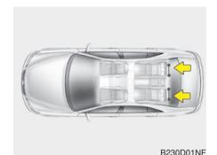
Some child seat manufacturers make child restraint seats that are labeled as LATCH or LATCH-compatible child restraint seats. LATCH stands for "Lower Anchors and Tethers for Children". These seats include two rigid or webbing mounted attachments that connect to two LATCH anchors at specific seating positions in your vehicle. This type of child restraint seat eliminates the need to use seat belts to attach the child seat in the rear seats.
