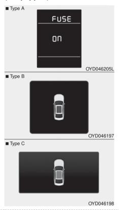
If the driver removes the ignition key (smart key: turns off the engine) and opens the driver-side door when the sunroof is not fully closed, the warning chime will sound for a few seconds and a warning image will appear on the LCD display.
