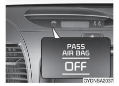
Your vehicle is equipped with an occupant detection system in the front passenger's seat.
