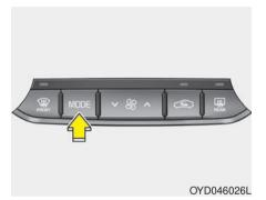
The mode selection button controls the direction of the air flow through the ventilation system.
