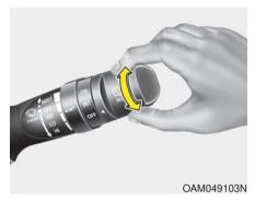
The rear window wiper and washer switch is located at the end of the wiper and washer switch lever. Turn the switch to desired position to operate the rear wiper and washer.
