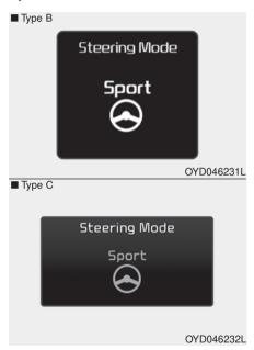
The steering wheel becomes heavier. The sport mode is usually used when driving on the highway.
