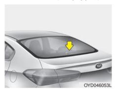
When the radio power switch is turned on while the ignition switch is in either the "ON" or "ACC" position, your car will receive both AM and FM broadcast signals through the antenna in the rear window glass.
