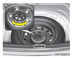
Turn the tire hold-down wing bolt counterclockwise.
