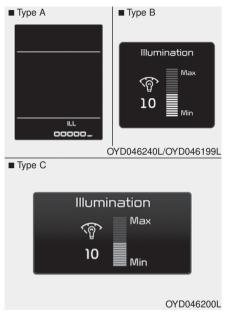
If you hold the illumination control button ("+" or "-"), the brightness will be changed continuously.  If the brightness reaches to the maximum or minimum level, an alarm will sound.
