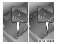
When using a floor mat on the floor carpet, make sure it attaches to the floor mat anchor(s) in the front and rear floor carpet of your vehicle. This keeps the floor mat from sliding forward.
