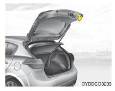
To close the tailgate, lower and push down the tailgate firmly. Make sure that the tailgate is securely latched. Make sure your hands, feet and other parts of your body are safely out of the way before closing the tailgate.
