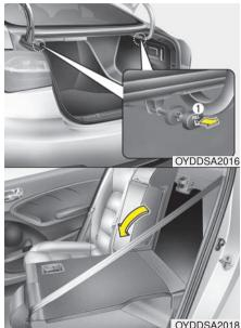
Pull the lock release lever (1) and fold the rear seatback forward and down firmly.
