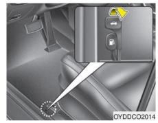
To open the trunk from inside the vehicle, pull the trunk lid release lever.
