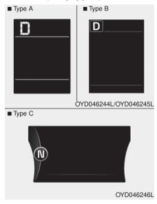
This indicator displays which automatic transaxle shift lever is selected.
