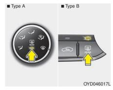
The defroster heats the window to remove frost, fog and thin ice from the interior and exterior of the rear window, while the engine is running.
