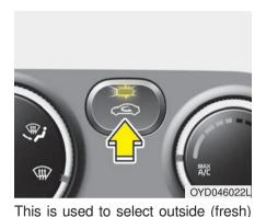
air position or recirculated air position. To change the air intake control position, push the control button.
