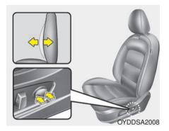
The lumbar support can be adjusted by pressing the lumbar support switch on the side of the driver's seat. Press the front portion of the switch to increase support, or the rear portion of the switch to decrease support.
