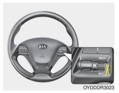
3.Move the lever down (to SET-), and release it at the desired speed. The SET indicator light in the instrument cluster will illuminate. Release the accelerator pedal at the same time. The desired speed will automatically be maintained.
