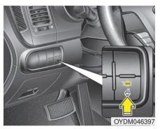
With the ignition switch in the ON position, pressing the heated steering wheel button warms the steering wheel. The indicator on the button will illuminate and notify you on the LCD display.
