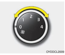
The ignition switch must be in the ON position for fan operation.
