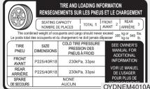
The label located on the driver's door sill gives the original tire size, cold tire pressures recommended for your vehicle, the number of people that can be in your vehicle and vehicle capacity weight.
