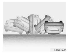
Front air bags may not inflate in rollover accidents because front air bag deployment would not provide additional occupant protection. However, side and curtain air bags may inflate when the vehicle is rolled over.
