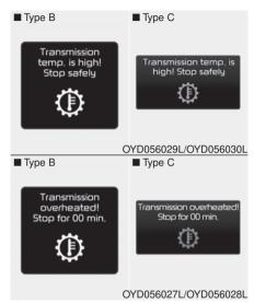
Under certain conditions such as repeated launch on steep grades, the clutch in the transmission could overheat. When the clutch is overheated, the safe protection mode engages.
