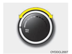
The temperature control knob allows you to control the temperature of the air flowing from the ventilation system. To change the air temperature in the passenger compartment, turn the knob to the right for warm air or left for cooler air.
