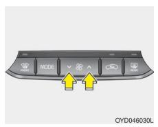
The fan speed can be set to the desired speed by pressing the fan speed control switch.
