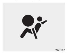
The purpose of the air bag warning light in your instrument panel is to alert you of a potential problem with your air bag - Supplemental Restraint System (SRS).
