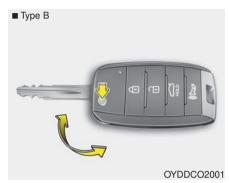
To unfold the key, press the release button and the key will unfold automatically.
