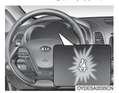
As a reminder to the driver, the driver's seat belt warning lights will illuminate for approximately 6 seconds each time you turn the ignition switch ON regardless of belt fastening.
