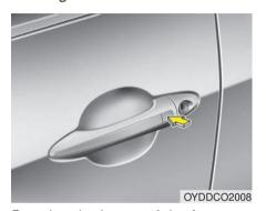
Pressing the button of the front outside door handles with all doors closed and any door unlocked, locks all the doors. The hazard warning lights will blink and the chime will sound once to indicate that all doors are locked. The button will only operate when the smart key is within 0.7~1 m (28~40 in.) from the outside door handle. If you want to make sure that a door has locked or not, you should check the door lock button inside the vehicle or pull the outside door handle.
