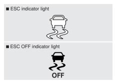
When the ignition switch is turned ON, the indicator light illuminates, then goes off if ESC system is operating normally.
