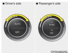
The temperature control knob allows you to control the temperature of the air flowing from the ventilation system. To change the air temperature in the passenger compartment, turn the knob to the right for warm air or left for cooler air.
