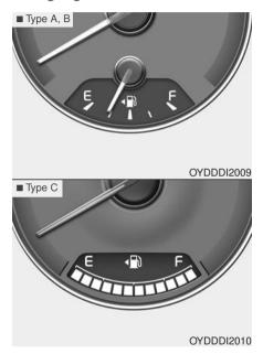
The fuel gauge indicates the approximate amount of fuel remaining in the fuel tank. The fuel tank capacity is given in chapter 8. The fuel gauge is supplemented by a low fuel warning light, which will illuminate when the fuel tank is nearly empty.
