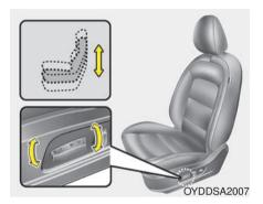
Pull the front portion of the control switch up to raise or down to lower the front part of the seat cushion. Pull the rear portion of the control switch up to raise or down to lower the rear part of the seat cushion. Release the switch once the seat reaches the desired position.
