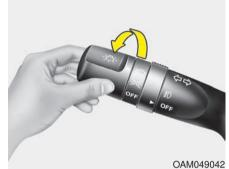
When the light switch is in the headlight position (2nd position) the head, tail, position, license and instrument panel lights will turn ON.
