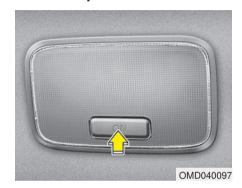
To turn the room lamp ON or OFF, push the switch.
