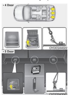
Child restraint hook holders are located on the package tray (4 Door) or the floor behind the rear seat (5 Door).
