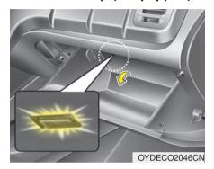
The glove box lamp comes on when the glove box is opened. To prevent unnecessary charging system drain, close the glove box securely after use.
