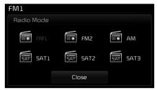
Pressing the **[RADIO]** button will change the operating mode in the order of FM1 → FM2 → AM → SAT1 → SAT2 → SAT3.
