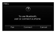
If Bluetooth® Wireless Technology devices are paired but none are currently connected, pressing the [PHONE] button or the [CALL] button on the steering wheel control displays the following screen. Press the [Pair] to pair a new device or press the [Connect] to connect a previously paired device.
