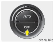
Press the OFF button to turn off the air climate control system. However you can still operate the mode and air intake buttons as long as the ignition switch is in the ON position.
