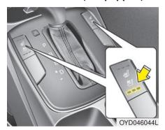
The ventilated seat is provided to cool or warm the seat during hot or cold weather by blowing air through small vent holes on the surface of the seat and seatback. While the engine is running, push the rear portion of the switch (blue color) to cool the seat, and push the front portion of the switch (red color) to warm the seat.
