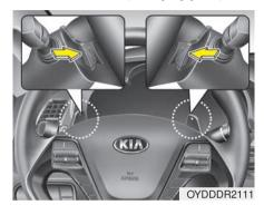
The paddle shifter is available when the shift lever is in the D (Drive) position or the manual mode.
