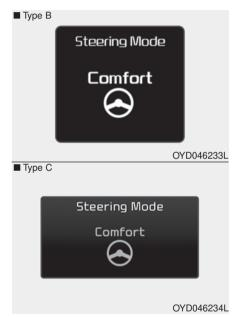
The steering wheel becomes lighter. The comfort mode is usually used when driving in the city or when parking the vehicle.
