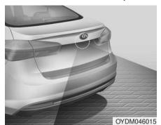
The rear view camera will activate with the ignition switch on and the shift lever in the R (Reverse) position.
