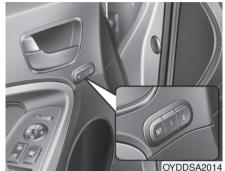
A driver position memory system is provided to store and recall the driver seat position with a simple button operation. By saving the desired position into the system memory, different drivers can reposition the driver seat based upon their driving preference. If the battery is disconnected, the desired seat position memory will need to be re-saved.
