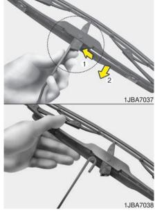
2. Compress the clip (1) and slide the blade assembly downward (2).
