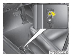
The fuel filler lid must be opened from inside the vehicle by pulling up the fuel filler lid opener.
