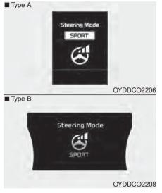
The steering wheel becomes heavier. The sport mode is usually used when driving on the highway.
