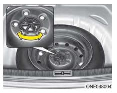
Turn the tire hold-down wing bolt counterclockwise.
