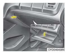
To open the glove box, push the button (1) and the glove box will automatically open. Close the glove box after use. Always keep the glove box closed while the vehicle is in motion.
