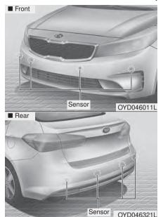
The parking assist system assists the driver during movement of the vehicle by chiming if any object is sensed within the distance of 100 cm (39.3 in ) in front or 120 cm (47 in) behind the vehicle.
