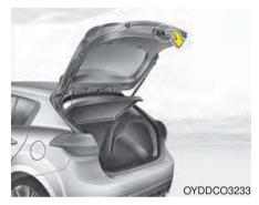
To close the liftgate, lower and push down the liftgate firmly. Make sure that the liftgate is securely latched.
