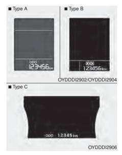
The odometer indicates the total distance the vehicle has been driven.
