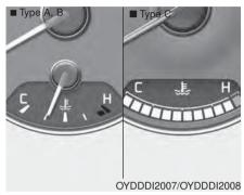
This gauge shows the temperature of the engine coolant when the ignition switch is ON.
