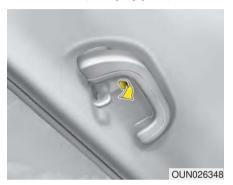
To use the coat hook, pull down the upper portion of the coat hook.
