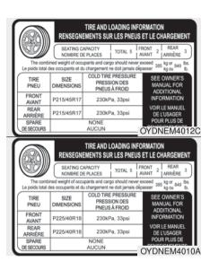
The label located on the driver's door sill gives the original tire size, cold tire pressures recommended for your vehicle, the number of people that can be in your vehicle and vehicle capacity weight.
