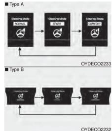
When the steering mode button is pressed, the selected steering mode will appear on the LCD display.
