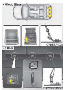
Child restraint hook holders are located on the package tray (4 Door, 2 Door) or the floor behind the rear seat (5 Door).
