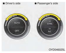
2. Turn the temperature control knob to set the desired temperature.
