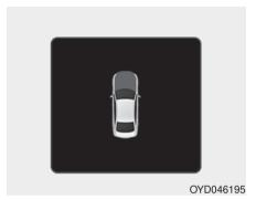
The warning message (if equipped) will appear on the LCD display when hood is open.
