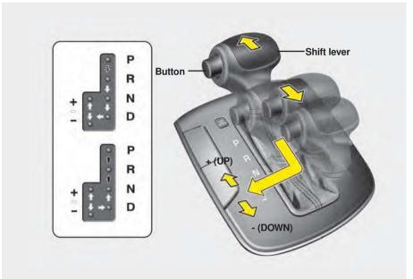
To shift, depress the brake pedal and press the button when the ignition switch is in the ON position.
