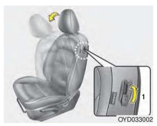
The driver and front passenger's seatback should be tilted to enter the rear seat.
