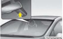
The Lane Keeping Assist System detects lane markers on the road, and assists the driver's steering to help keep the vehicle between lanes.
