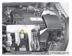
Pull the suspected fuse straight out. Use the removal tool provided in the engine compartment fuse panel.
