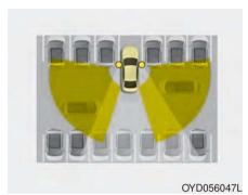
When your vehicle moves backwards from a parking position, the sensor detects approaching vehicles to the left or right side direction and gives information to the driver.
