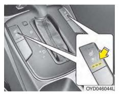
The climate control seat is provided to cool or warm the seat during hot or cold weather by blowing air through small vent holes on the surface of the seat and seatback. While the engine is running, push the rear portion of the switch (blue color) to cool the seat, and push the front portion of the switch (red color) to warm the seat.
