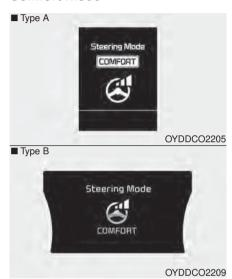
The steering wheel becomes lighter. The comfort mode is usually used when driving in the city or when parking the vehicle.
