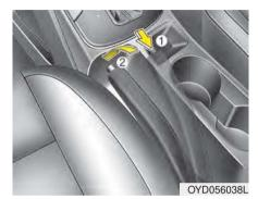
To release the parking brake, first apply the foot brake and pull up the parking brake lever slightly. Secondly, press the release button (1) and lower the parking brake lever (2) while holding the button.
