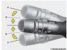
The ignition switch must be on for the turn signals to function. To turn on the turn signals, move the lever up or down (A). The green arrow indicators on the instrument panel indicate which turn signal is operating. They will self-cancel after a turn is completed. If the indicator continues to flash after a turn, manually return the lever to the OFF position.
