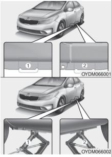
7. Place the jack at the front or rear jacking position closest to the tire you are changing. Place the jack at the designated locations under the frame. The jacking positions are plates welded to the frame with two tabs and a raised dot to index with the jack.
