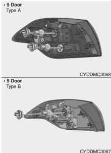
Remove the socket from the assembly by turning the socket counterclockwise until the tabs on the socket align with the slots on the assembly.
