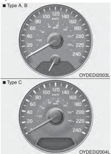
The speedometer indicates the forward speed of the vehicle.
