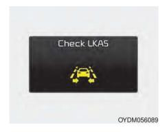
The LKAS fail indicator (yellow) will illuminate with an audible warning if the LKAS is not working properly. We recommend that you contact an authorized Kia dealer.
