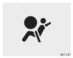
The SRS (Supplement Restraint System) air bag warning light on the instrument panel displays the air bag symbol depicted in the illustration.
