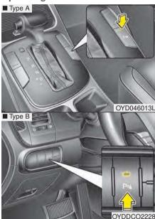
This system will activate when the parking assist button is pressed with the engine running.
