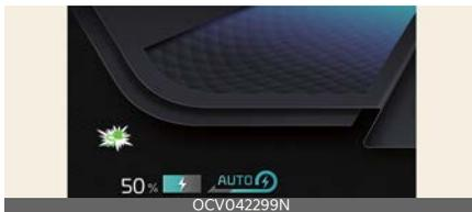
When the charging connector is not connected properly, reconnect the charging cable to charge it again.
