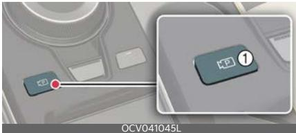
Press the Parking/View button (1) to turn on or off Rear View Monitor while P (Park) position is selected.
