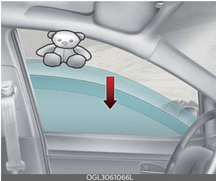
If the window detects the resistance while the power window switch is pulled up continuously, the window will stop upward movement then lower approximately 2.5 cm (1 inch).
