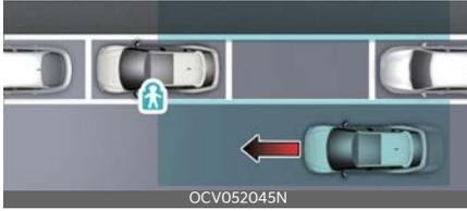
After the vehicle stops, when an approaching vehicle from the rear area is detected as soon as a passenger opens a door, Safe Exit Assist will warn the driver with a warning message and an audible warning to help prevent a collision.
