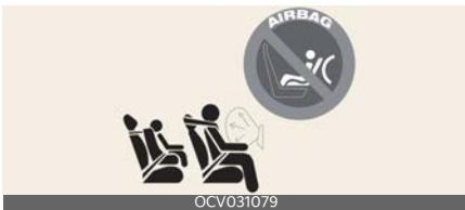
If the air bag deploys, it would impact the rear-facing child restraint, causing serious or fatal injury.
