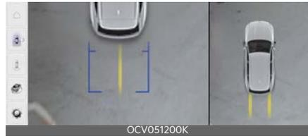
Parking guidance is displayed on the right side of the 360° camera monitoring system screen when the **Front or Rear Top View Parking Guidance** is selected.
