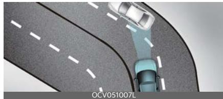
The smart regeneration system may recognize a vehicle in an adjacent lane when driving on a curved road. In this case, the system increase the braking level and slow the vehicle.
