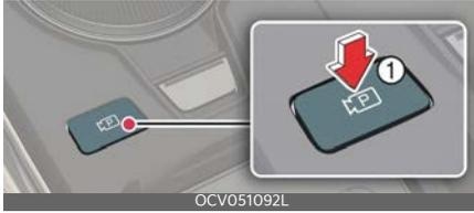
1. With the vehicle turned on, depress the brake pedal and shift the gear to P (Park) or N (Neutral).
