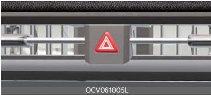
It should be used whenever emergency repairs are being made or when the vehicle is stopped near the edge of a roadway.
