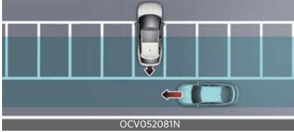
Rear Cross-Traffic Collision-Avoidance Assist may detect vehicles passing by behind you when parking backwards into a parking space. If this occurs, the function may unnecessarily warn the driver and control the brake.
