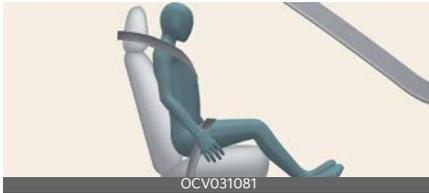
When an adult is seated in the front passenger seat, if the PASSENGER AIR BAG OFF indicator is on, change EV button to the OFF position and ask the passenger to sit properly (sitting upright with the seatback in an upright position, centered on the seat cushion with their seat belt on, legs comfortably extended and their feet on the floor). Restart the vehicle and have the person remain in that position. This will allow the system to detect the person and to enable the passenger air bag.
