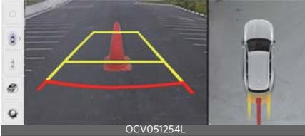
Parking distance warning is displayed on the right side of the 360° camera monitoring system top view screen when the **Parking Distance Warning** is selected.
