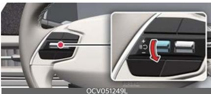
Push the - switch down and release it immediately. The set speed will decrease by 1 km/h (1 mph) each time the switch is operated in this manner.
