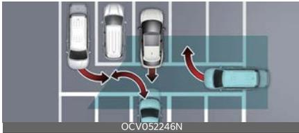
Rear Cross-Traffic Collision-Avoidance Assist may detect vehicles which are parking or pulling out near your vehicle (for example: a vehicle leaving beside your vehicle, a vehicle parking or pulling out in the rear area, a vehicle approaching your vehicle making a turn, etc.). If this occurs, the function may unnecessarily warn the driver and control the brake.
