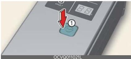
5. Each time the button (1) is pressed, the control box display is sequentially changed to 12 A, 10 A and 8 A. Once the charging current setting is complete, start charging (refer to "Portable charge (sold separately)" on page 1-30 for more information).
