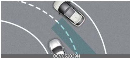
Blind-Spot Collision-Avoidance Assist may not operate properly when driving on a curved road. Blind-Spot Collision-Avoidance Assist may not detect the vehicle in the next lane.
