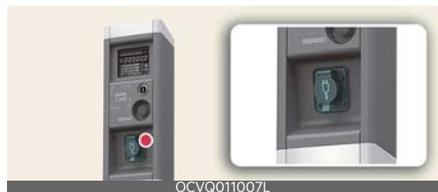
2. Hold the charging connector handle (2) and pull it while pressing the release button (1).
