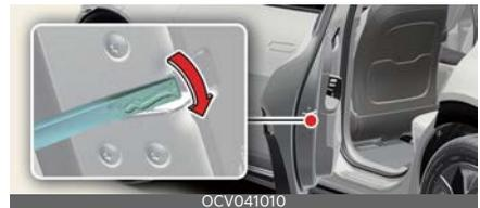
In case of emergency such as when the battery is discharged, the only way to lock the door(s) is with the mechanical key from the outside key hole. Doors without an outside key hole can be locked as follows:
