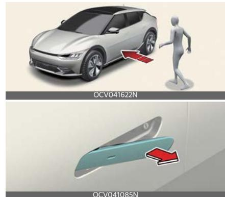
If you approach (within 30 cm (1 ft.)) the driver or front passenger's door handle possessing the smart key, the outside door handles slide out and the doors are unlocked. In this case, Hazard Warning
