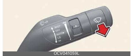
1. Move the wiper speed control switch to the OFF position.
