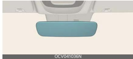
The sensor mounted in the mirror senses the light level around the vehicle, and automatically controls the headlamp glare from the vehicles behind you. When the vehicle is running, the glare is automatically controlled by the sensor mounted in the rear view mirror.
