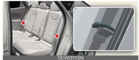
4. Pull on the seatback folding lever, then fold the seat toward the front of the vehicle. When you return the seatback to its upright position, always be
