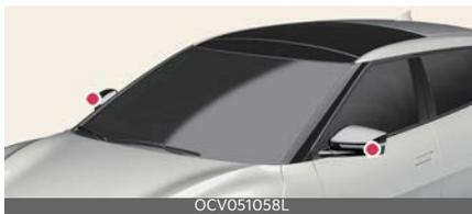
(camera located at bottom of the mirror)
