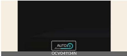
If the front radar recognizes the vehicle in front, 'AUTO' is displayed in blue. The regenerative braking level is automatically controlled depending on the driving condition of the vehicle in front and the level is indicated with arrows.
