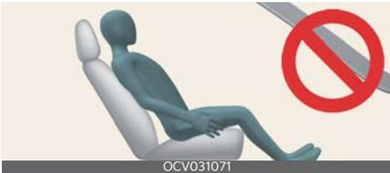
The driver must advise the passengers to keep the seatback in an upright position whenever the vehicle is in motion. If a seat is reclined during an accident, the restraint system's ability to restrain will be greatly reduced.
