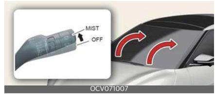
After turning off the vehicle, move the wiper switch to the single wiping (MIST) position within 20 seconds and hold the switch more than 2 seconds until the wiper blade is in the fully up position.
