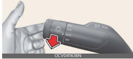
It will return to the normal (low beam) position when released. The headlight switch does not need to be on to use this flashing feature.
