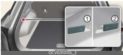
Pull the rear seatback folding switch (1, 2) located on both sides of the cargo area.
