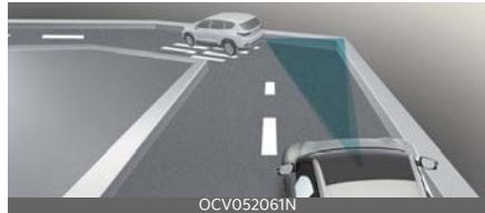
On curved roads, Smart Cruise Control may not detect a vehicle in the same lane, and may accelerate to the set speed. Also, vehicle speed may rapidly decrease when the vehicle ahead is detected suddenly.
