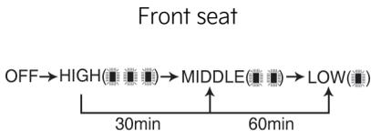
You may manually press the button to increase the seat temperature. However, it soon returns to the automatic mode again. When pressing the button for more than 1.5 seconds with the seat warmer operating, the seat warmer will turn OFF. The seat warmer defaults to the OFF position whenever the vehicle is in the ON position.
