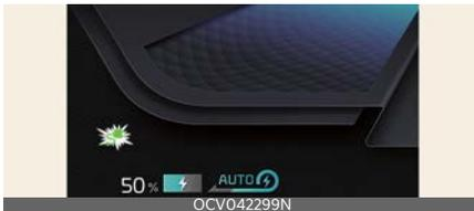
Charging does not occur when the charging indicator lamp is OFF. When the charging connector and charging plug are not connected properly, reconnect the charging cable to charge.
