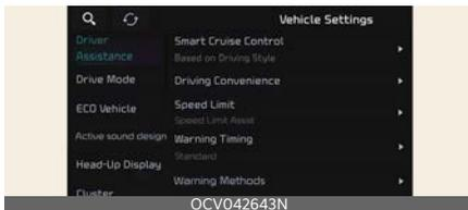
Select **Setup** → **Vehicle** → **Driver Assistance** on the infotainment system screen to set the Driver Assistance function.
