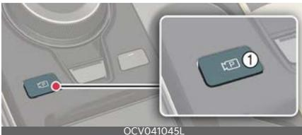
Press the Parking/View button (1) to turn on or off 360° camera monitoring system.
