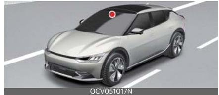
The front view camera is used to detect driving patterns and front vehicle departure while vehicle is being driven.
