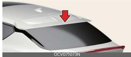
If the high mounted stop lamp (LED) does not operate, have your vehicle checked by an authorized Kia dealer.
