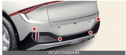
Refer to the picture above for the detailed location of the detecting sensors.
