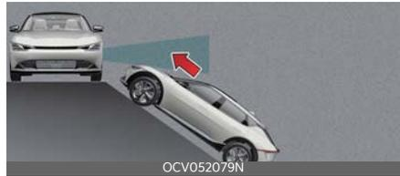
Rear Cross-Traffic Collision-Avoidance Assist may be limited when the vehicle is on a uphill or downhill slope, or near it, and may not detect the vehicle approaching from the blind spot area. If this occurs, the function may not warn the driver or control the brakes when necessary.
