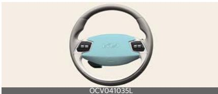
The horn will operate only when this area is pressed. Check the horn regularly to be sure it operates properly.
