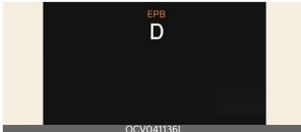
If the EPB malfunction indicator remains on, comes on while driving, or does not come on when the EV button is changed to the ON position, this indicates that the EPB may have malfunctioned.
