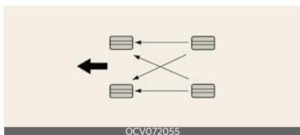
Rotate radial tires that have an asymmetric tread pattern only from front to rear and not from right to left.
