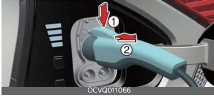
To prevent charging cable theft, the charging connector cannot be disconnected from the inlet when the vehicle's doors are locked. Unlock all doors to disconnect the charging connector from the inlet.
