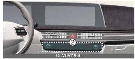
Front view function is displayed on the screen when the gear is in N (Neutral) or D (Drive) to assist in parking. The front view has a top view, front view, side view and 3D view. Also, other view modes can be selected by pressing the view icons on the 360° camera monitoring system screen.
