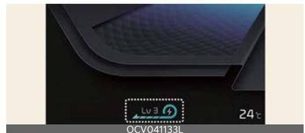
Initial setting of the regenerative braking level and adjustable range vary according to the selected Drive mode.
