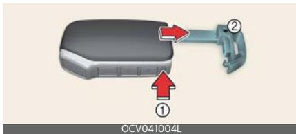
To reinstall the mechanical key, put the key into the hole and push it until a click sound is heard.
