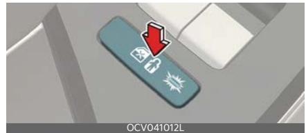
If you push the electronic child safety lock switch and the indicator appears, rear passengers cannot open the rear door from inside the vehicle.
