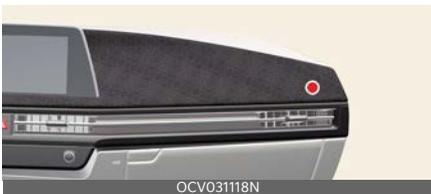
The indication of the system's presence are the letters "AIR BAG" located on the air bag pad cover on the steering wheel and the passenger's side front panel pad above the glove box.
