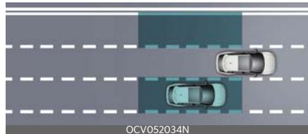
Blind-Spot Collision-Avoidance Assist helps detect and inform the driver that a vehicle is in the blind spot.
