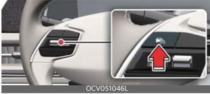
Press the Driving Assist (DA) button to turn Smart Cruise Control off.
