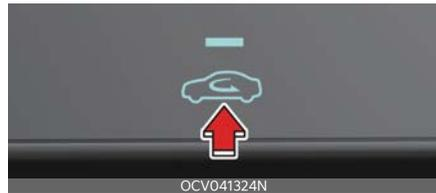
With the outside (fresh) air position selected, air enters the vehicle from outside and is heated or cooled according to the function selected. The indicator light will turn off.
