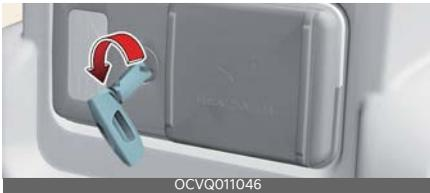
2. Connect to the power outlet located in the base of the rear seat with the EV button in the ON position.
