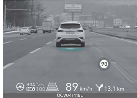
The Head-Up Display projects the instrument cluster and navigation information onto the windshield.
