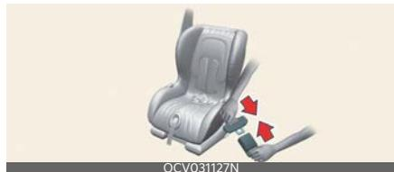
3. Pull the shoulder portion of the seat belt all the way out. When the shoulder portion of the seat belt is fully extended, it will shift the retractor to the "automatic locking" (child restraint) mode.
