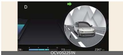
Blind-Spot View Monitor displays the rear blind spot area of the vehicle in the cluster when the turn signal is turned on to help safely change lanes.
