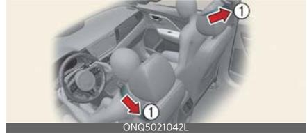
The pre-tensioner seat belts may be activated when a frontal collision is severe enough, together with the air bags.
