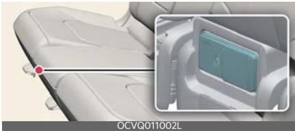
3. Check the operation status through the front indicator of the power outlet.
