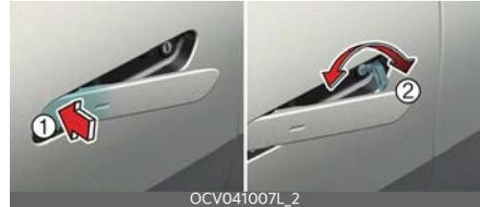
Press the front part (1) of the door handle to pull out the rear part of the door handle. While keep pressing the front part of the door handle, insert the mechanical key (2) to the lock with the key handle facing the ground as shown. To lock the door, turn the key toward the front (left side) of the vehicle. To unlock, turn the key toward the rear (right side) of the vehicle.
