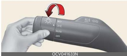
When the light switch is in the parking light position, the tail, license and instrument panel lights will turn ON.
