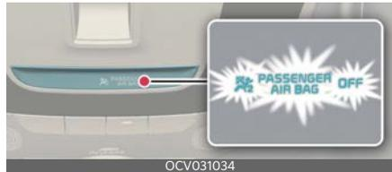
The occupant detection system is designed to detect the presence of a properly-seated front passenger and determine if the passenger's front air bag should be enabled (may inflate) or not. Only the front passenger front air bag is controlled by the Occupant Detection System.
