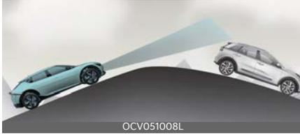
When driving uphill or downhill, the system may not detect the vehicle in your lane and the regenerative braking level will reduce automatically, making you feel that the vehicle is accelerating.
