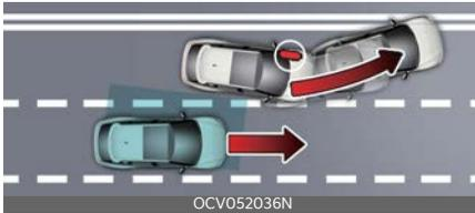
When changing lanes by detecting the lane ahead, if Blind-Spot Collision-Avoidance Assist judges that there is a collision risk with an approaching vehicle in the blind spot, it will help avoid collision by applying the brake.
