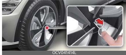
For 20 inch wheel, take out the remover tool in the Tire Mobility Kit. Insert the tool to the hole and pull out the wheel cover.
