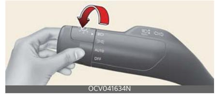
When the light switch is in the headlamp (Low beam) position, the head, tail, license lights will turn ON.
