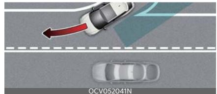
Blind-Spot Collision-Avoidance Assist may not operate properly when driving where the road merges or divides. Blind-Spot Collision-Avoidance Assist may not detect the vehicle in the next lane.
