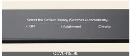
Press and hold the button to select the default mode for the control panel.
