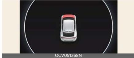
The warning chime will operate when the vehicle is being driven above 3 km/h (2 mph) with the hood open.
