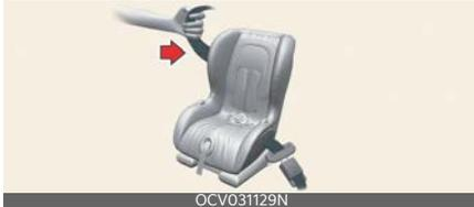
5. Remove as much slack from the belt as possible by pushing down on the child restraint system while feeding the shoulder belt back into the retractor.
