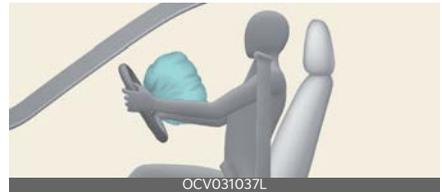
Upon deployment, tear seams molded directly into the pad covers will separate under pressure from the expansion of the air bags. Further opening of the covers then allows full inflation of the air bags.
