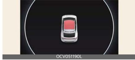
If the driver turns off the vehicle when the sunroof is not fully closed, the warning chime will sound for several seconds and the sunroof open warning will appear on the cluster LCD display. Close the sunroof securely when leaving your vehicle.
