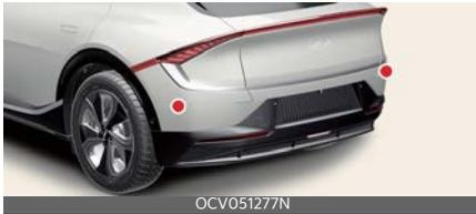
Refer to the picture above for the detailed location of the detecting sensors.
