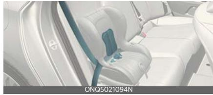
Since all passenger seat belts move freely under normal conditions and only lock under extreme or emergency conditions (emergency locking mode), you must manually pull the seat belt all the way out to shift the retractor to the "automatic locking" mode to secure a child restraint.
