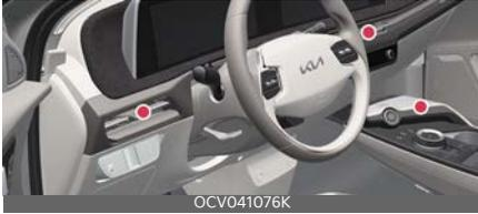
The ambient lights are installed in the front crash pad, front doors, and the top/bottom of the center console.
