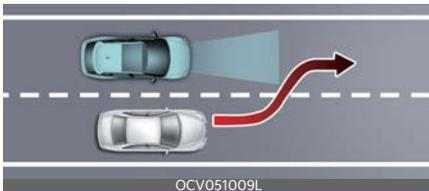
When a vehicle changes lanes in front of you, the smart regeneration system may not immediately detect the vehicle, especially if the vehicle changes lanes abruptly. In this case, you must maintain a safe braking distance, and if necessary, depress the brake pedal to reduce
