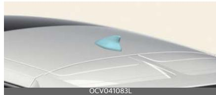
The shark fin antenna receives data transmitted from base stations and satellites (e.g. AM/FM, GPS, Sirius XM, LTE) and also transmits to base stations (e.g. LTE).
