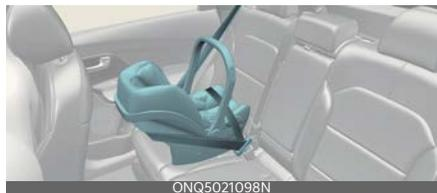
A rear-facing child seat provides restraint with the seating surface against the back of the child. The harness system holds the child in place, and in an accident, acts to keep the child positioned in the seat and reduces the stress to the neck and spinal cord.
