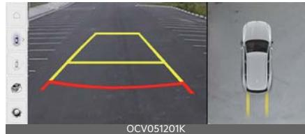
Rear view parking guidance is displayed in the rear view when the **Parking Guide in Rear View** is selected.
