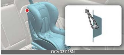
1. Route the child restraint tether strap over the child restraint seatback. Route the tether strap under the head restraint and between the head restraint posts, or route the tether strap over the top of the vehicle seatback. Make sure the strap is not twisted.
