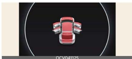
This warning is displayed if any door or the hood or the liftgate is left open. The warning will indicate which door is open in the display.
