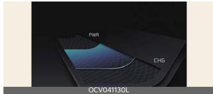
The Power/Charge gauge shows the energy consumption rate of the vehicle and the charge/discharge status of the regenerative brakes.
