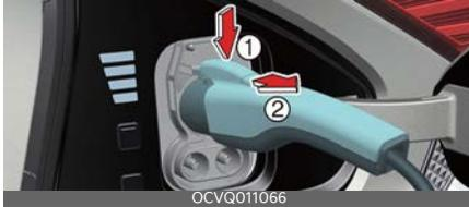
Before disconnecting the charging connector, make sure the vehicle's doors are unlocked. When the doors are locked, the charging connector lock system will be triggered. And the charging connector will not be disconnected.
