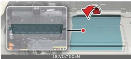
3. Remove the climate control air filter case (2) by pulling out left side of the cover (1).
