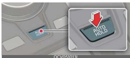
2. When coming to a complete stop by depressing the brake pedal, the AUTO HOLD indicator changes from white to green indicating the AUTO HOLD is engaged.
