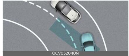
Blind-Spot Collision-Avoidance Assist may not operate properly when driving on a curved road. Blind-Spot Collision-Avoidance Assist may detect a vehicle in the same lane.
