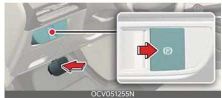
1. Releasing the parking brake with EPB switch,
