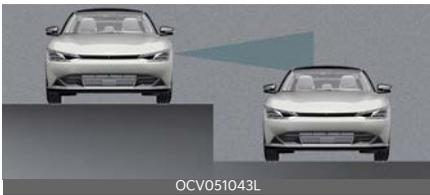
Blind-Spot Collision-Avoidance Assist may not operate properly when driving where the heights of the lanes are different. Blind-Spot Collision-Avoidance Assist may not detect the vehicle on a road with different lane heights.
