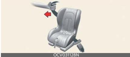
4. Slowly allow the shoulder portion of the seat belt to retract and listen for an audible "clicking" or "ratcheting" sound. This indicates that the retractor is in the "automatic locking" mode. If no distinct sound is heard, repeat steps 3 and 4.
