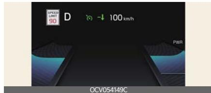
If the speed limit of the road changes during the operation of Manual Speed Limit Assist or Smart Cruise Control, an arrow in the direction of up or down is displayed to inform the driver that the set speed needs to be changed. At this time, the driver can change the set speed according to the speed limit by using the + or - switch on the steering wheel.
