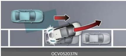
When you are driving forward out of a parking space, if Blind-Spot Collision-Avoidance Assist judges that there is a collision risk with an approaching vehicle in the blind spot, it will help avoid collision by applying the brake.
