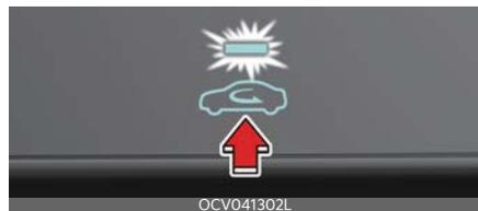
With the recirculated air position selected, air from the passenger compartment will be drawn through the heating system and heated or cooled according to the function selected. Prolonged operation of the heater in the recirculated air position (without air con-
