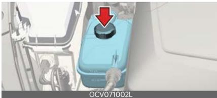
Replace any swollen or deteriorated hoses. The coolant level should be filled between F (MAX) and L (MIN) marks on the side of the coolant reservoir when motor compartment is cool. When the coolant level (in the reservoir) is low, have your vehicle inspected by an authorized Kia dealer. Use only designated coolant water for electric vehicles,
