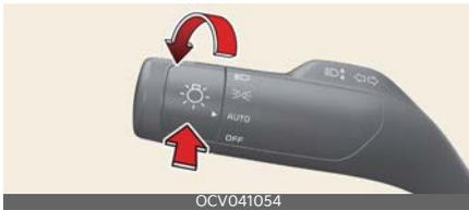
High Beam Assist is a function that automatically adjusts the headlamp range (switches between high beam and low beam) depending on the brightness of detected vehicles and certain road conditions.
