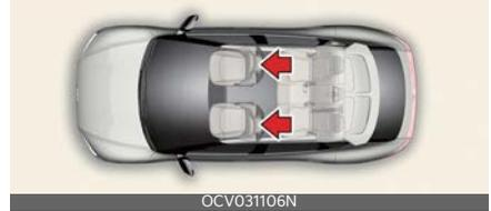
The headrest not only provides comfort for the driver and front passenger, but also helps protect the head and neck in the event of a rear collision.
