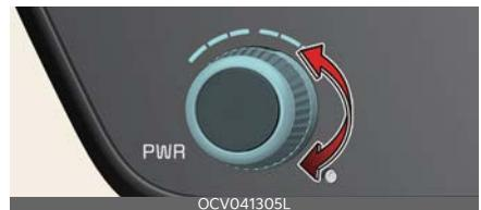
The temperature will increase to the maximum (HI) by turning the knob to the extreme right.
