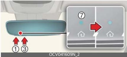
1. Press and hold the buttons (1) and (3) simultaneously
