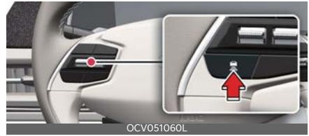
Each time the button is pressed, the vehicle distance changes as follows:
