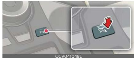
Press the Parking Safety (P<sub>SA</sub>) button to turn on or off Forward/Reverse Parking Distance Warning.
