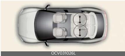
LATCH anchors have been provided in the left and right outboard rear seating positions. Their locations are shown in the illustration. There are no LATCH anchors provided for the center rear seating position.
