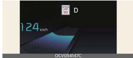
When driving at a speed higher than the displayed speed limit, the red speed limit indicator will blink.
