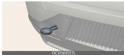
1. Open the liftgate, and remove the towing hook from the tool case.
