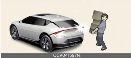
If you are positioned in the detecting area (50~100 cm [20~40 inches] behind the vehicle) carrying a smart key, the hazard warning lights will blink and chime will sound to alert you the smart key has been detected and the liftgate will open.
