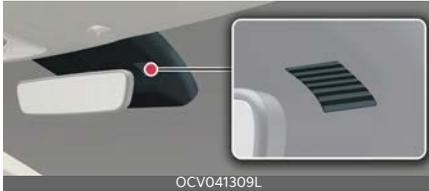
The auto defogging system operates when the heater or air conditioning is on. The indicator appears when the auto defogging system senses the moisture on the inside of the windshield and operates.
