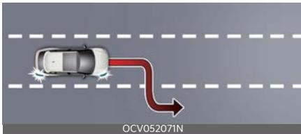
Highway Lane Change Assist function helps change lanes to the direction the driver slightly moves the turn signal switch if the function judges that lane change is possible.
