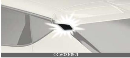
When all doors are locked and closed, the body silhouette lamp will come on for 15 seconds if any of the below is performed.
