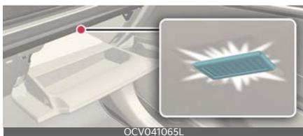
The glove box lamp comes on when the glove box is opened.
