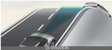
During uphill or downhill driving, the Smart Cruise Control may not detect a moving vehicle in your lane, and cause your vehicle to accelerate to the set speed. Also, vehicle speed will rapidly decrease when the vehicle ahead is detected suddenly.
