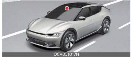
The front view camera is used as a detecting sensor to detect ambient light and brightness while driving. Refer to the picture above for the detailed location of the detecting sensor.
