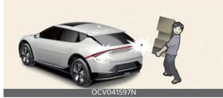
After the hazard warning lights blink and the chime sounds 6 times, the smart liftgate will open.
