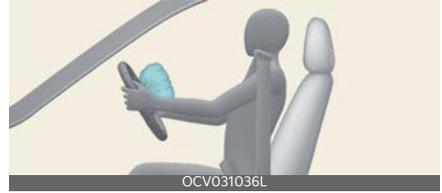
The front air bag modules are located both in the center of the steering wheel and in the front passenger's panel above the glove box. When the SRSCM detects a sufficiently severe impact to the front of the vehicle, it will automatically deploy the front air bags.
