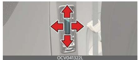
The outlet vents can be opened or closed by moving the vent left or right. Also, you can adjust the direction of air delivery from these vents using the vent control lever as shown.
