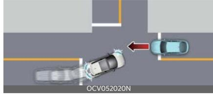
Junction Turning function may help avoid a collision with an oncoming vehicle in an adjacent lane when turning left at a crossroad with the turn signal on by applying emergency braking.
