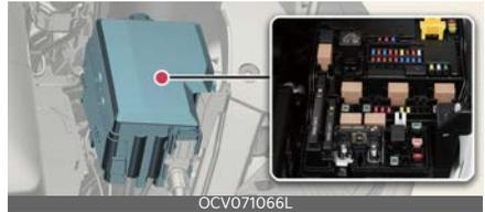
3. Check the removed fuse; replace it if it is blown. To remove or insert the fuse, use the fuse puller in the motor compartment fuse panel.
