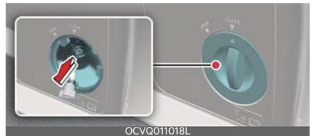
If the charging cable does not detach due to battery discharge and failure of the electric wires, open the liftgate and slightly pull the emergency cable on the right side area as shown above. The charging connector will then unlock.
