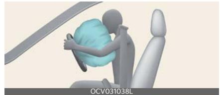
A fully inflated air bag, in combination with a properly worn seat belt, slows the driver's or the passenger's forward motion, reducing the risk of head and chest injury.
