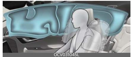
Side and/or curtain air bags are designed to inflate when an impact is detected by side collision sensors depending on the severity of impact resulting from a side impact collision.
