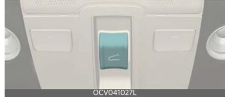
The sunroof can only be operated when the EV button is in the ON or START position.
