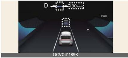
If you want to speed up temporarily without altering the set speed while Smart Cruise Control is operating, depress the accelerator pedal. While the accelerator pedal is depressed, the set speed, distance level and target distance will blink on the cluster.
