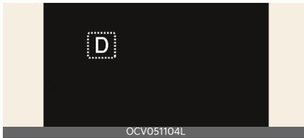
The indicator in the instrument cluster displays the gear position when the EV button is in the ON position.
