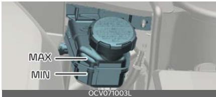
1. Before removing the reservoir cap and adding brake fluid, clean the area around the reservoir cap thoroughly to prevent brake fluid contamination.
