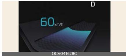
The speedometer indicates the speed of the vehicle and is calibrated in kilometers per hour (km/h) and/or miles per hour (mph).
