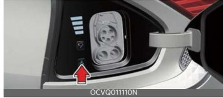
When you press the charging button for immediate charging, the scheduled charge setting is not completely deactivated. If you need to completely deactivate the scheduled charge setting, use the multimedia system or the Kia Connect application on your smart phone.
