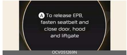
**A: To release EPB, fasten seatbelt and close door, hood and liftgate**
