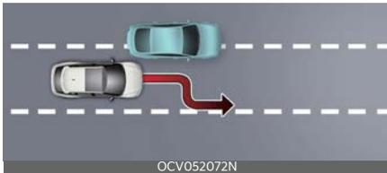
When vehicle speed is above 60 km/h (40 mph), if a vehicle around you is driving at a close distance, your vehicle will control steering in the opposite direction of the vehicle to assist in safe driving. If there are vehicles in both sides of the lane that are driving close to you, the function will not veer to the opposite side of the lane.
