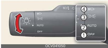
To operate the lights, turn the knob at the end of the control lever to one of the following positions:
