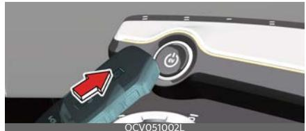
The side with the lock button should contact the EV button directly.
