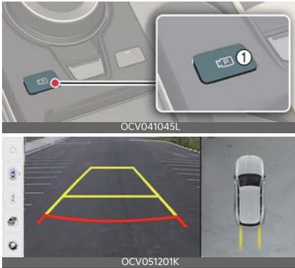
360° camera monitoring system can assist in parking by allowing the driver to see around the vehicle.
