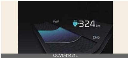
The distance to empty is displayed differently according to the selected drive mode in the drive mode integrated control system.
