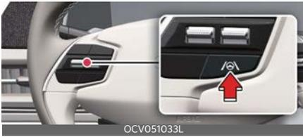
With the vehicle on, press and hold the Lane Driving Assist button located on the steering wheel to turn on Lane Keeping Assist. The gray (LKA) indicator light will appear on the cluster.
