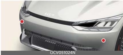
The front view camera, front radar, and front corner radars (if equipped) are used as a detecting sensor to detect the vehicles in front.
