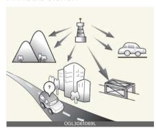
FM broadcasts are transmitted at high frequencies and do not bend to follow the earth's surface. Because of this, FM broadcasts generally begin to fade within short distances from the station. Also, FM signals are easily affected by buildings, mountains, and obstructions.
