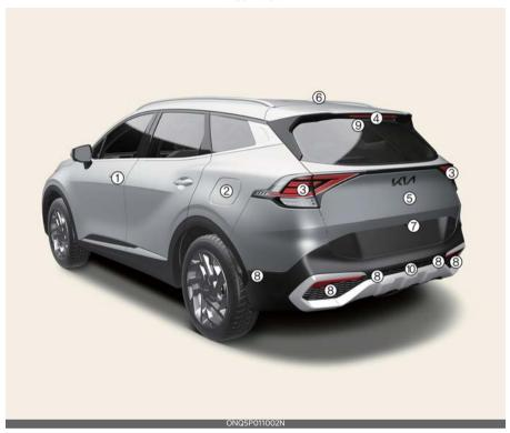
\* The actual shape of your Kia may differ from the illustration. 1. Doors 5-15 2. Fuel filler door 5-40 5-98, 9-58 3. Rear combination lamp 4. High mounted stop lamp 5-98, 9-58 5. Liftgate 5-24 6. Antenna 5-143 7. Wide-rear view camera 7-90 8. Rear ultrasonic sensor 7-109 5-103, 9-25 9. Rear wiper 10.Backup lamp 5-98, 9-58
