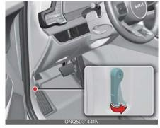
Go to the front of the vehicle, raise the hood slightly, push the secondary hood release lever (1) to the left and lift the hood (2).
