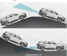
Blind-Spot Collision-Avoidance Assist may not operate properly when driving on an inclined road. Blind-Spot Collision-Avoidance Assist may not detect the vehicle in the next lane or may incorrectly detect the ground or structure.
