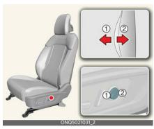
The lumbar support can be adjusted by pressing the lumbar support switch on the side of the seat.
