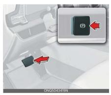
Releasing the parking brake with EPB switch.
