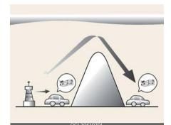
AM broadcasts can be received at greater distances than FM broadcasts. This is because AM radio waves are transmitted at low frequencies. These long distance, low frequency radio waves can follow the curvature of the earth rather than traveling straight. In addition, they curve around obstructions resulting in better signal coverage.
