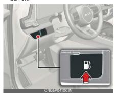
Wait until the fuel tank is depressurized. The message is displayed when the fuel filler door unlocks after the fuel tank is depressurized.
