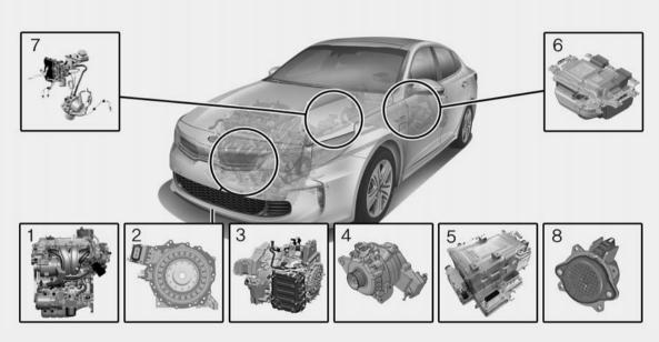
1. Engine: 2.0L 2. Motor: 35kW
