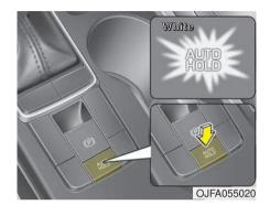
1.Depress the brake pedal, start the engine and then press the Auto Hold button. The white AUTO HOLD indicator will come on indicating the system is in standby. Before the Auto Hold will engage, the driver's door, engine hood must be closed and the driver's seat belt must be fastened.
