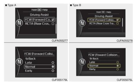
The driver can select the initial warning activation time in the User Settings in the instrument cluster LCD display. The options for the initial Forward Collision Warning include the following:
