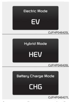
A corresponding message is displayed when a mode is selected by pressing the HEV button.
