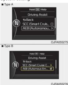
The driver can activate the AEB by placing the engine start/stop button to the ON position and by selecting 'User Settings', 'Driving Assist', and 'Autonomous Braking System'. The AEB deactivates, when the driver cancels the system setting.
