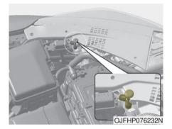
If the charging door does not open due to battery discharge, open the hood and slightly pull the emergency cable which is located in headlamp cover as shown above.
