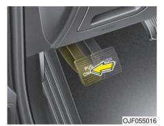
To release the parking brake, depress the parking brake pedal a second time while applying the foot brake. The pedal will automatically extend to the fully released position.
