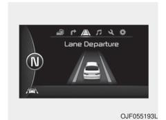
If you select this symbol, the LDWS mode on the LCD display will appear. If the system detects that your vehicle is leaving the lane when the LDWS is operating and vehicle speed exceeds 64 km/h (40 mph), the warning operates as follows:
