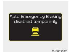
When the sensor is covered or the sensor lens is dirty with foreign substances, such as snow or rain, the AEB operation may temporarily stop. In this case, a warning message will appear to notify the driver.
