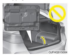
Never touch the safety plug. Safety plug is attached to high voltage hybrid battery system. Touching safety plug will result in death or serious injury. Service personnel should follow procedure in service manual.
