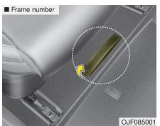
The vehicle identification number (VIN) is the number used in registering your vehicle and in all legal matters pertaining to its ownership, etc. The number is punched on the floor under the passenger seat.
