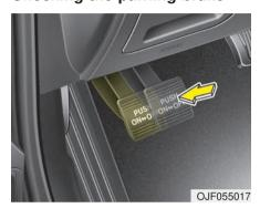
Check whether the stroke is within specification when the parking brake pedal is depressed with 30 kg, 294 N (66 lb) of force. Also, the parking brake alone should securely hold the vehicle on a fairly steep grade. If the stroke is more or less than specified, have the parking brake adjusted by an authorized Kia dealer.
