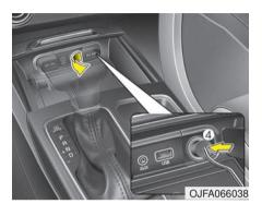
Connect between compressor and the vehicle power outlet using the cable and connectors (4).
