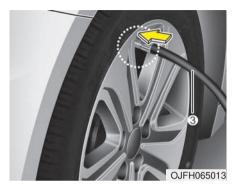
6. Unscrew the valve cap from the valve of the defective wheel and screw filling hose (3) of the sealant bottle onto the valve.
