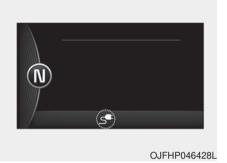
Check if the charging cable connection indicator of the high voltage battery in the instrument cluster is turned ON.
