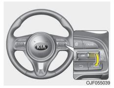
Move the lever down (to SET-), and release it at the desired speed. The SET indicator light in the instrument cluster will illuminate. Release the accelerator at the same time. The desired speed will automatically be maintained.
