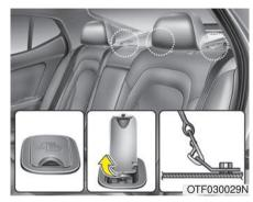
Child restraint hook holders are located on the package tray.
