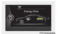
The mode means the vehicle at stop. (No energy flow)
