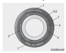
This information identifies and describes the fundamental characteristics of the tire and also provides the tire identification number (TIN) for safety standard certification. The TIN can be used to identify the tire in case of a recall.
