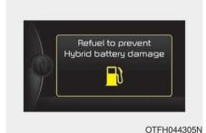
If the fuel tank is nearly empty, a message "Refuel to prevent Hybrid battery damage" will appear on the LCD display. Also, the chime will sound several times.
