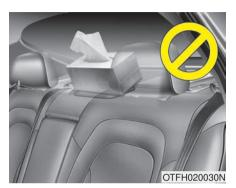
The hybrid battery air intake is located behind the rear seats. The hybrid battery air intake is used to cool the hybrid battery. If the hybrid battery air intake is blocked, the hybrid battery may overheat. Do not cover the air intake with objects.
