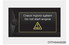
If the engine does not start and SOC (State Of Charge) is very low or vehicle defects the hybrid system's problem. a message will appear on the LCD display. Also, the chime will sound until the problem is solved.
