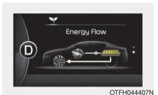
The engine and regenerative braking systems charge the hybrid battery during deceleration.
