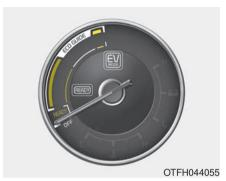
This is a gauge to let drivers know efficient the current driving conditions are. The fuel efficiency is high in the green zone but is low in the red zone.
