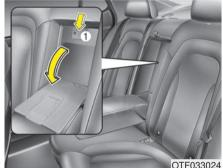
Pull the armrest down using the strap provided on the armrest. Pull the cover down while pushing the release lever down. Additional cargo space is provided to accommodate long/narrow cargo (skis, poles, lumber, etc.) not able to fit properly in the trunk when closed. Make sure the engine is off, the shift lever is in P and the parking brake is applied whenever loading or unloading cargo. The vehicle may move if the shift lever is inadvertently moved to another position.
