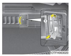
This service plug (1) located in the rear trunk as shown should always be pulled out to disconnect and turn off the hybrid system.
