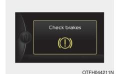
'Check brake' is displayed when the brake function is not well or the regenerative brake system is not operated with brake system malfunction. Refer to the "Brake system warning light" in this chapter.
