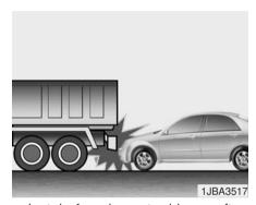
Just before impact, drivers often brake heavily. Such heavy braking lowers the front portion of the vehicle causing it to "ride" under a vehicle with a higher ground clearance. Air bags may not inflate in this "under-ride" situation because deceleration forces that are detected by sensors may be significantly replaced by such "under-ride" collisions.
