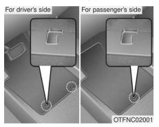
When using a floor mat on the floor carpet, make sure it attaches to the floor mat anchor(s) in your vehicle. This keeps the floor mat from sliding forward.
