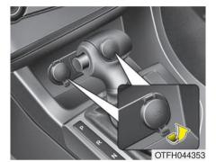
The power outlet is designed to provide power for mobile telephones or other devices designed to operate with vehicle electrical systems. The devices should draw less than 10 amps with the engine running.
