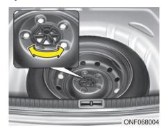
Turn the tire hold-down wing bolt counterclockwise.
