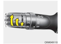
The light switch has a Headlight and a Parking light position.
