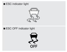
When the ignition switch is turned ON, the indicator light illuminates, then goes off if ESC system is operating normally.
