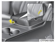
To open the center console storage, pull the lever up.
