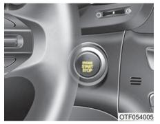
Whenever the front door is opened, the ENGINE START/STOP button will illuminate for your convenience. The light will go off after about 30 seconds after the door is closed.
