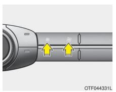
The fan speed can be set to the desired speed by pressing the fan speed control switch.
