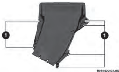
First Water Separation Chamber
