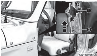
Attaching Mirror Bracket To The Vehicle
