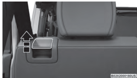
Lift Seatback Release Lever Up
