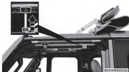
Attach Rear Door Rail Bolt
