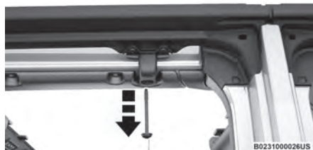
Remove Screws From Below Frame
