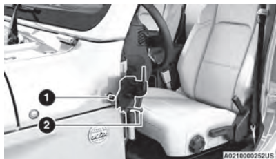
Attaching Mirror Bracket To The Vehicle
