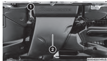
First Water Separation Chamber
