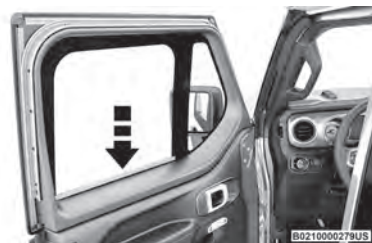
Push Down To Fully Seat Upper Half-Door Door Latch Alignment
