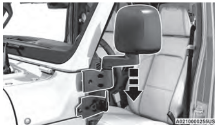
Lower Mirror Assembly Onto Bracket
