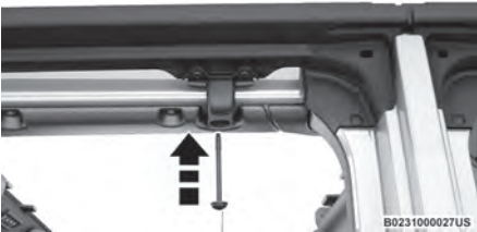
Insert Screws From Below Frame
