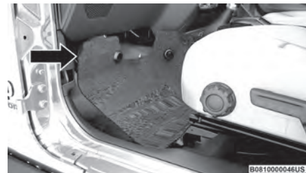
Front Carpet Pulled Away
