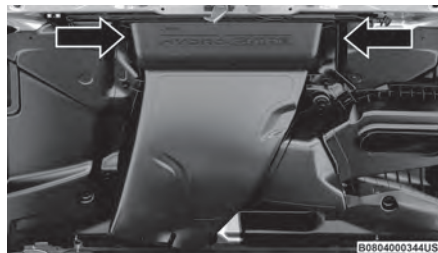
First Water Chamber Removal
