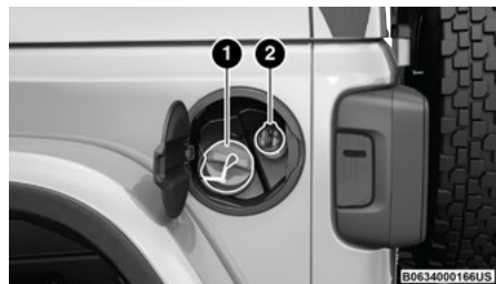
Fuel and Diesel Exhaust Fluid Fill Location
