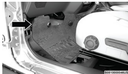
Front Carpet Pulled Away
