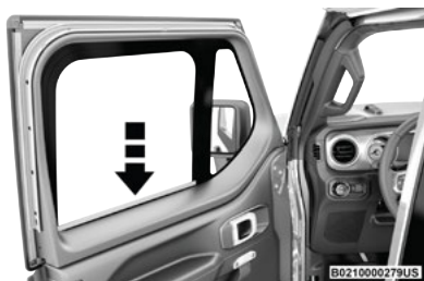
Push Down To Fully Seat Upper Half-Door
