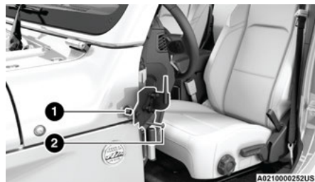
Attaching Mirror Bracket To The Vehicle
