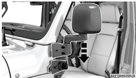
Lower Mirror Assembly Onto Bracket
