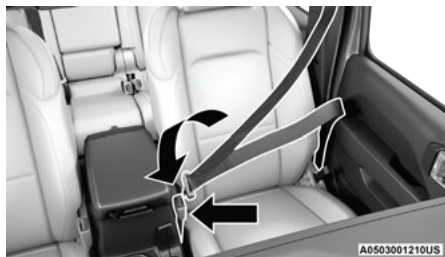
Inserting Latch Plate Into Buckle
