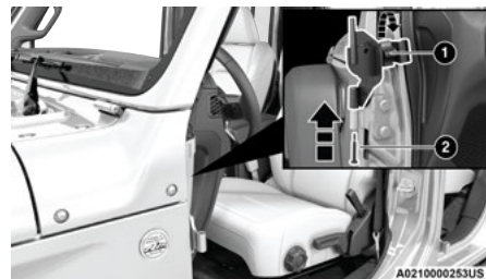
Attaching Mirror Bracket To The Vehicle
