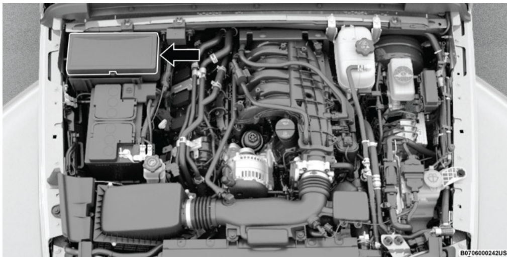
Power Distribution Center Location - Gasoline Engine
