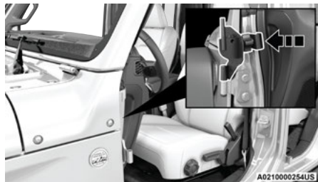
Push Bracket Onto A-pillar
