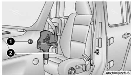
Attaching Mirror Bracket To The Vehicle
