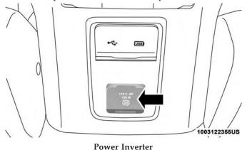
The power inverter is designed with built-in overload protection. If the power rating of 150 Watts is exceeded, the power inverter will automatically shut down. Once the electrical device has been removed from the outlet, the inverter should automatically reset. If the power rating exceeds approximately 170 Watts, the power inverter may have to be reset manually.
