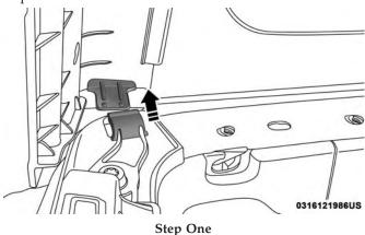
2. Starting at the rear of the vehicle, remove plastic retainer from along the bottom of the window moving toward the front of the vehicle.
