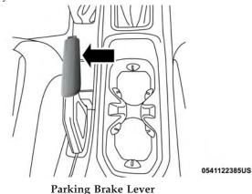
When the parking brake is applied with the ignition switch ON, the "Brake Warning Light" in the instrument cluster will illuminate.
