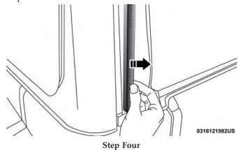
5. While keeping the rear window level, slide to the left until it is completely separate from its retainer. Do not pull downward while removing the rear window. Damage to the retainer could result.
