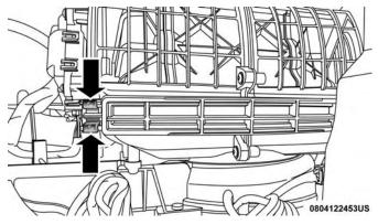
Air Filter Retaining Tabs
