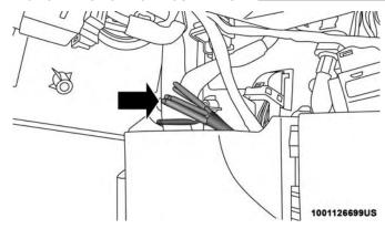
Auxiliary Switch Connections – Passenger Side Panel In addition to the four auxiliary switch wires, a fused battery wire and ignition wire are also located in the interior, in the passenger outboard foot well area.
