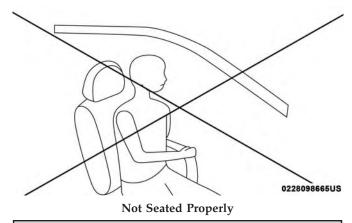
• If a child restraint system, child, small teenager or adult in the front passenger seat is seated improperly, the occupant may provide an output signal to the OCS that is different from the occupant's properly seated weight input. This may result in serious injury or death in a collision.
