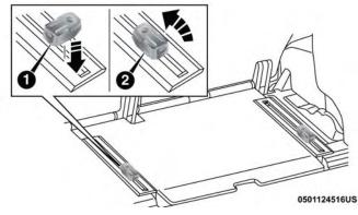
**Installing Adjustable Slides**
