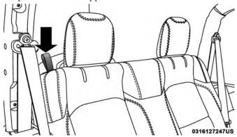
Rear Head Restraint Folding Strap Location
