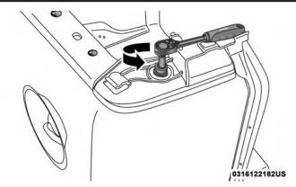
Remove Rear Retainers Installing The Soft Top — Four Door Models
