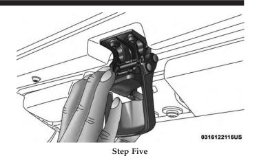
6. Pull the handle back upward while squeezing the hook, locking the latch into place.
