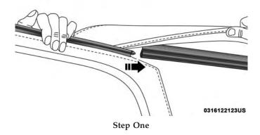
2. Insert the tailgate bar into the retainers at the bottom of the window from left to the right.
