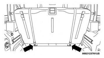
Tether Strap Anchorages (Two-Door Models) Four-Door Models:
