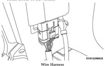
7. Release the locking tab by pushing it downward.
