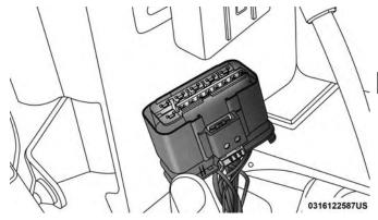
**Pull Wiring Harness To Separate**
