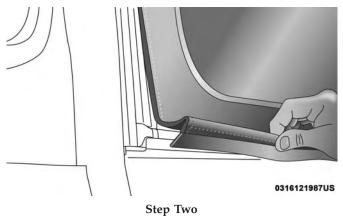
3. Remove plastic retainer from bottom to top of the window.
