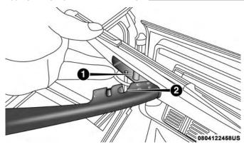
Wiper Blade Removed From Wiper Arm
