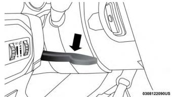
Tilt/Telescoping Steering Column Lever
