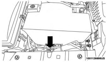
Auxiliary Switch Connections - Under Hood
