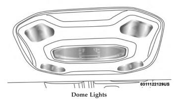
When a door is open and the interior lights are on, rotating the dimmer control to the extreme bottom position will cause all the interior lights to turn off. This is also known as "Party" mode because it allows the doors to stay open for extended periods of time without discharging the vehicle's battery.
