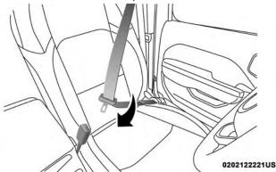
Inserting Latch Plate Into Buckle
