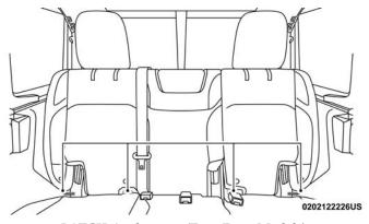
LATCH Anchorages (Four-Door Models) Locating The Upper Tether Anchorages
