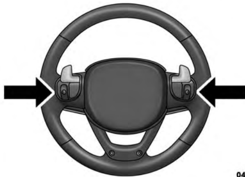
Remote Sound System Controls (Back View Of Steering Wheel)
