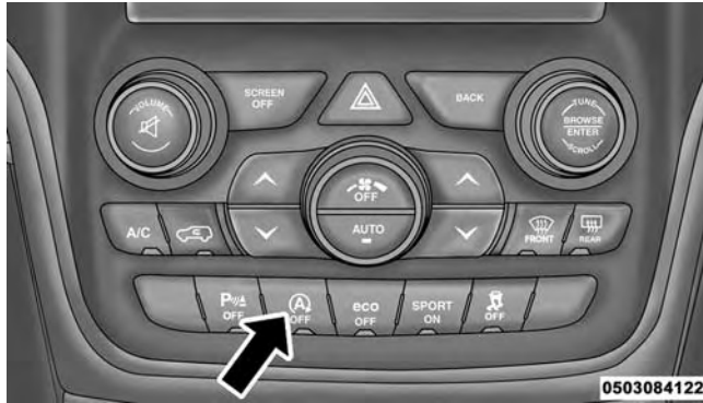
STOP/START Off Switch
