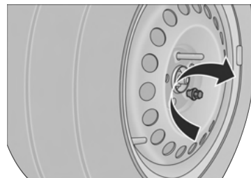
Installing Wheel Bolts
