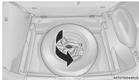
Removing Jack And Spare Tire Fastener
