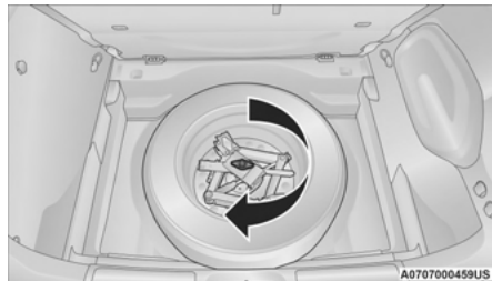
Reinstalling Jack and Tire Fastener
