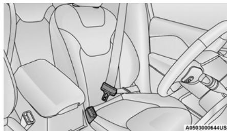
Pulling Out The Latch Plate
