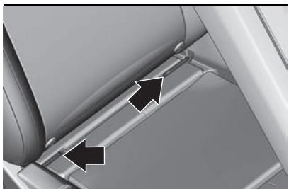
fig. 150 ISOFIX child restraints for the front passenger seat (where provided).
