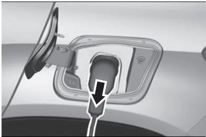
274 Disconnect the vehicle plug of the charging cable from the charging port fig. 274 within 30 seconds after unlocking.
