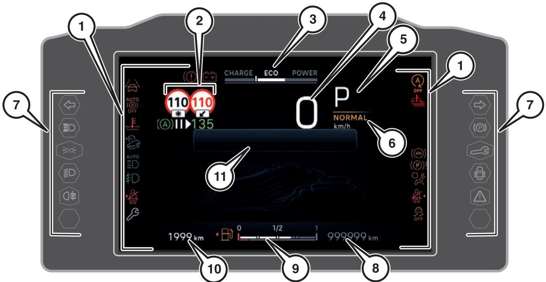
1. Warning, signalling and notification symbols 2. Driving assistance systems notifications 3. Auxiliary battery operating mode (where provided) 4. Digital speedometer 5. Engaged gear indicator 6. Drive mode indicator 7. Warning, signalling and notification lamps 8. Odometer 9. Digital fuel level gauge (the triangle on the left side of the symbol indicates the side of the vehicle with the fuel filler) 10. Estimated autonomy 11. Message area
