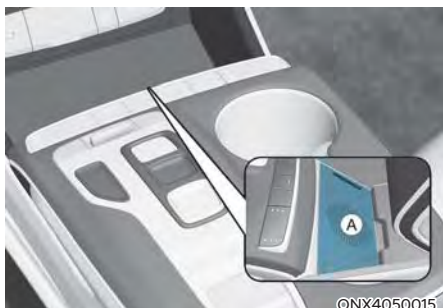
[A] : Wireless Charging Pad (In-vehicle Authentication Pad)
