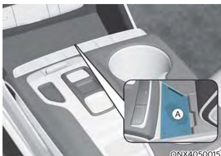
[A] : Wireless Charging Pad (In-vehicle Authentication Pad)
