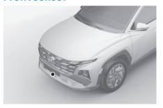
Front radar detects the distance between your vehicle and the vehicle ahead to control the regenerative braking intensity.
