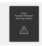
When Forward Attention Warning is not working properly, the "Check Forward Attention Warning system" warning message will appear on the cluster. If this occurs, have the vehicle inspected by an authorized HYUNDAI dealer.
