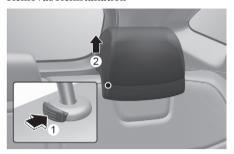
To remove the head restraint:
