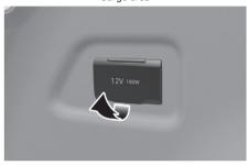
The power outlet is designed to provide power for mobile phones or other devices designed to operate with vehicle electrical systems. The devices should draw less than 12 V, 180 W with the engine running.
