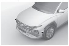
These ultrasonic sensors are mounted near the front wheels outside your vehicle.
