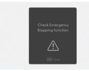
When Emergency Stop is not working properly, the "Check Emergency Stopping function." warning message appears, and the master (△) warning light illuminates on the instrument cluster. If this occurs, have your vehicle inspected by an authorized HYUNDAI dealer.
