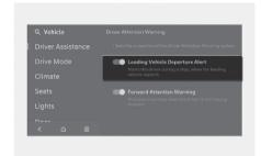
With the engine on, select or deselect Setup > Vehicle > Driver Assistance > Driver Attention Warning and then enable Leading Vehicle Departure alert in the infotainment system to set whether to use each function.
