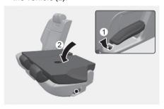
5. Lift and push the seatback rearward while lifting up the front portion of the folding lever.
