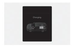
The high voltage battery is charged up by the regenerative brake system. (Wheel > Battery)
