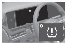
The TPMS Malfunction Indicator illuminates after it blinks for about one minute when there is a problem with the Tire Pressure Monitoring System.
