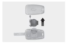
Battery type: CR2032 To replace the battery:
