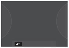
The outside ambient temperature appears in the lower portion of the cluster display. The temperature reads in Fahrenheit or Celsius depending on the units selected from the Settings menu in the infotainment system.
