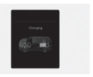
The engine braking is simultaneously used to decelerate the vehicle and to charge up the high voltage battery.
