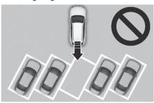
Remote Operation may not operate provide properly in a diagonal parking space.
