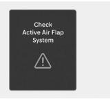
The active air flap system may not operate normally if the air flap is temporarily opened due to foreign factors or if the controller is contaminated by snow or rain, etc.
