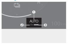
When the smart regeneration system is ON, the regenerative braking level appears as "AUTO" on the instrument cluster. The "AUTO" appears in grey in the ready state. The system automatically controls the regenerative braking level (2) according to the smart regeneration system operating conditions. If the front radar detects a vehicle in front, the indicator light (3) appears in green.
