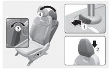
To reinstall the head restraint:
