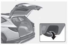
Lower the tailgate lid and press down until it locks. Always check it is secure by pulling on the handle.
