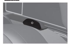
The in-cabin camera is mounted to the steering wheel.
