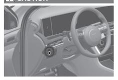
Detach the speed restriction label (1) from the Compressor (6), and place it in a highly visible place inside the vehicle such as on the steering wheel to remind the driver not to drive too fast.
