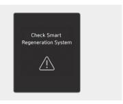
If the rear radar is covered by any foreign material, such as snow, rain, or dirt, the detecting performance may decrease and disable the smart regeneration system.
