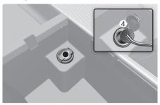
6. With the ignition switch ON, switch on the compressor and let it run for approximately 5~7 minutes to fill the sealant up to proper pressure. (refer to the "Tires and wheels" section in chapter 10). The inflation pressure of the tire after filling is unimportant and will be checked/corrected later.
