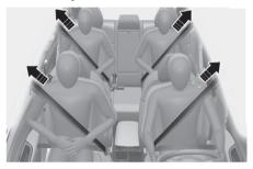
Your vehicle is equipped with driver's and front passenger's and rear passengers pretensioner seat belts (retractor pretensioner). The pretensioner makes sure the seat belts fit tightly against your body in certain frontal or side collision(s). The pretensioner seat belts may be activated in some crashes where the frontal or side collision(s) is severe enough, together with the airbags.
