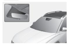
The rain sensor located on the upper end of the windshield glass senses the amount of rainfall and controls the interval of the wiping cycle.
