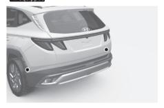
These ultrasonic sensors are mounted near the rear wheels outside your vehicle.
