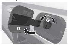
6. Place the fuel tank cap (2) on the fuel filler door (1).
