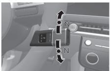
To shift the gear to N (Neutral), rotate the rotary gear shift dial to N (Neutral) from R (Reverse) or D (Drive) while depressing the brake pedal.
