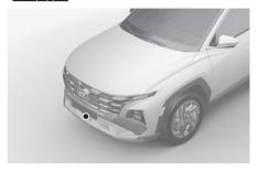
The front radar is mounted behind the front arill.
