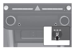
While the engine is running, press the button to cool the driver's seat or front passenger's seat.
