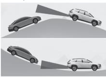
Blind-Spot Collision-Avoidance Assist may not operate properly when driving on a slope. The function may not detect the vehicle in the next lane or may incorrectly detect the ground or structure. Always pay attention to road and driving conditions while driving.
