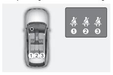
As a reminder to the rear passenger, the rear passenger's seat belt warning lights will illuminate for about 6 seconds each time the Engine Start/Stop button is in the ON position regardless of belt fastening.
