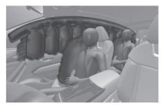
Side and curtain airbags are designed to inflate when an impact is detected by side collision sensors depending on the severity of impact resulting from a side impact collision.
