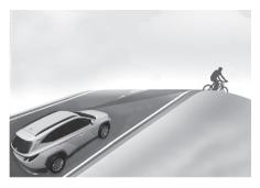
Forward Collision-Avoidance Assist may not detect other vehicles, powered two-wheelers, pedestrians or cyclists in front of you while driving uphill or downhill, adversely affecting the performance of the sensors.
