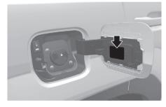
Charging label is located on the charging inlet cover's inside. For more details, refer to "Charging your plug-in hybrid vehicle" in the chapter 1.
