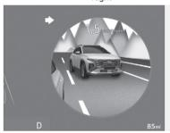
Blind-Spot View Monitor uses the wide-side view cameras to display the rear blind spot areas of your vehicle on the instrument cluster when the turn signal is turned on to help with safe lane changes.
