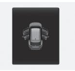
This warning appears if any door or hood or tailgate is left open. The warning indicates which door is open on the cluster display.
