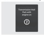
Repeated sudden acceleration and quick start may overheat the transmission. If the transmission is overheated, the self protection mode alarms the driver with an audible sound warning message.
