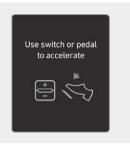
When Highway Driving Assist is operating, your vehicle will stop if the vehicle ahead of you stops. Also, if the vehicle ahead of you starts moving within 30 seconds after the stop, your vehicle will start as well. In addition, after the vehicle has stopped and 30 seconds have passed, the "Use switch or pedal to accelerate" message will appear on the instrument cluster. Depress the accelerator pedal or operate the + switch, - switch or IIO switch to start driving.
