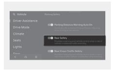
With the engine on, select or deselect **Vehicle** > **Driver Assistance** > **Parking Safety** in the infotainment system to set whether to use each function.
