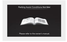
When "Parking Assist Conditions Not Met" message appears when Parking/View (P) button has been pressed and held while Remote Smart Parking Assist is in standby. After a while, press and hold the Parking/View (P) button again to see if Remote Smart Parking Assist works.
