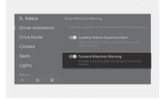
If 'Forward Attention Warning' is enabled, the function warns the driver when the driver's gaze is not focused on the road
