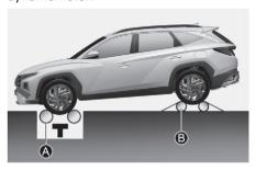
[A] Roll tester (Speedometer)[B] Temporary free roller
