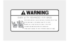
Airbag warning labels, required by the Canadian Motor Vehicle Safety Standards (CMVSS), are attached to alert the driver and passengers of potential risks of the airbag system. Be sure to read all of the information about the airbags that are installed on your vehicle in this Owners Manual.
