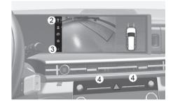
The front view appears on the screen when the gear is in N (Neutral) or D (Drive) to assist in parking.
