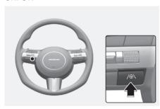
With the engine on, shortly press the Lane Driving Assist button located on the steering wheel to turn on Lane Following Assist. The gray or green (⋈) indicator light will illuminate on the instrument cluster.
