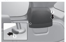
To reinstall the head restraint:
