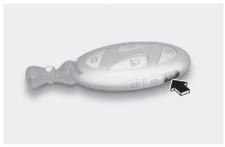
When the tailgate is closed, press the power tailgate open button for 1 second. The tailgate will open with a warning sound.
