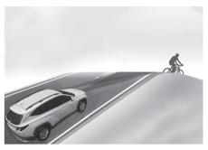
Forward Collision-Avoidance Assist may not detect other vehicles, powered two-wheelers, pedestrians or cyclists in front of you while driving uphill or downhill, adversely affecting the performance of the sensors.
