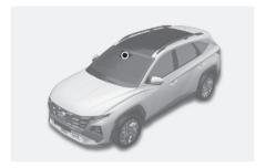
The front view camera is mounted near the top of the windshield inside your vehicle.
