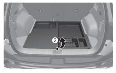
If the charging connector does not disconnect after pulling the emergency cable,
