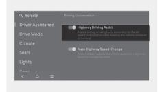
With the engine on, select or deselect Setup > Vehicle > Driver Assistance > Driving Convenience > Highway Driving Assist from the infotainment system to set whether to use each function.
