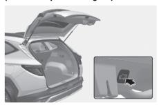
Press the power tailgate open/close button. The tailgate opens or closes automatically.
