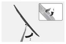
Lift up the wiper blade clip (1). Then pull down the wiper blade (2).
