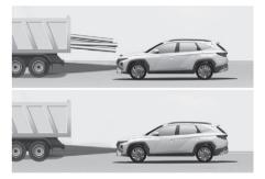
When the vehicle in front of the foregoing vehicle is at a stop and the foregoing vehicle changes the lane, the front sensors may be unable to recognize the stopped vehicle.
