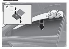
If a window senses any obstacle while it is closing automatically, it stops and lowers approximately 30 cm (12 in.) to allow the object to be cleared.
