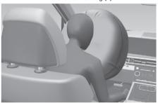
Upon deployment, tear seam in the pad cover separates from the expansion of the airbags.
