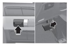
Press the **II 3** switch or depress the brake pedal to temporarily cancel Smart Cruise Control.
