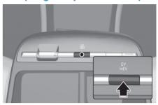
Pressing the EV/HEV button changes the plug-in hybrid system modes, between Electric (CD) mode and Hybrid (CS) mode.
