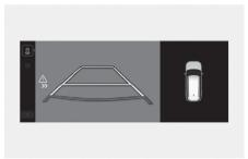
To warn the driver of an approaching vehicle from the rear left/right side of your vehicle, the warning light on the side view mirror will blink and a warning will appear on the instrument cluster. At the same time, an audible warning will sound. If Rear View Monitor is operating, a warning will also appear on the infotainment system.
