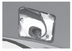
5. Remove the bulb from the socket by pressing it in and rotating it counterclockwise until the tabs on the bulb align with the slots in the socket. Pull the bulb out of the socket.
