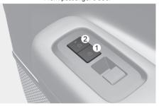
When pressing the  $(\triangle)$  portion (1) on the switch, all vehicle doors are locked.
