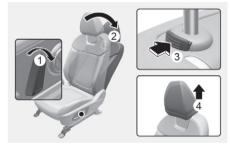
To remove the head restraint:
