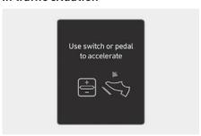
In traffic, your vehicle will stop if the vehicle ahead of you stops. Also, if the vehicle ahead of you starts moving, your vehicle will start as well. In addition, after the vehicle has stopped and a certain time have passed, the "Use switch or pedal to accelerate" message will appear on the instrument cluster. Depress the accelerator pedal or operate the + switch, - switch or IIO switch to start driving.
