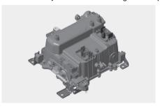
• High voltage battery system: Located under front seat
