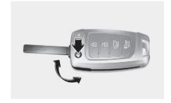
If the remote key does not operate normally, you can lock or unlock the door by using the mechanical key.
