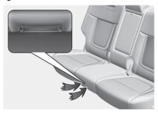
The hybrid battery cooling duct is located below the passenger seat. The cooling duct cools down the hybrid battery. When the hybrid battery cooling duct is blocked, the hybrid battery may be overheated.
