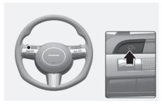
Press the Driving Assist button to turn Cruise Control off. The Cruise (MCRUISE) indicator will go off.
