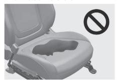
Do not place sharp objects on the front passenger seat. These may damage the occupant detection system, if they puncture the seat cushion.
