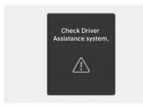
When Driver Attention Warning is not working properly, the "Check Driver Assistance system" warning message will appear on the cluster for several seconds, and the master (A) warning light and the inattentive driving (b) warning light will appear on the instrument cluster. If this occurs, have your vehicle inspected by an authorized HYUNDAI dealer.
