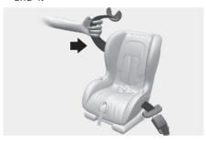
Remove as much slack from the belt as possible by pushing down on the Child Restraint System while feeding the shoulder belt back into the retractor.
