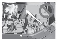
High voltage cut-off switch is a device located inside the engine compartment to block the battery's high voltage when your vehicle is inspected at an authorized HYUNDAI dealer.
