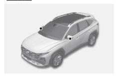
The wide-side view cameras are mounted to the bottom of the side view mirrors outside your vehicle.
