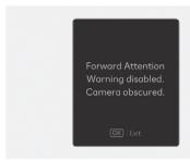
When there is an object right in front of the in-cabin camera or between the driver and the camera for a certain period of time, Forward Attention Warning does not operate properly, and the "Forward Attention Warning disabled. Camera obscured." warning message appears on the instrument cluster, and an audible warning sounds.
