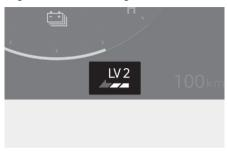
The selected regenerative braking level appears on the instrument cluster.
