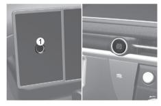
Place your finger on the fingerprint sensor (1) to verify your fingerprint. After it is successfully verified, start the engine by pressing the Engine Start/Stop button within 30 seconds.
