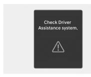
When Intelligent Speed Limit Assist is not working properly, the "Check Driver Assistance system." warning message will appear on the instrument cluster for several seconds, and the master (△) warning light and (□) warning light will illuminate on the instrument cluster. If this occurs, have your vehicle inspected by an authorized HYUNDAI dealer.
