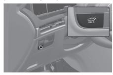
When the tailgate is closed, press the power tailgate open/close button for 1 second. The power tailgate opens with a warning sound.
