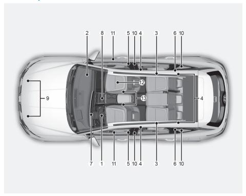
The SRS consists of the following components:
