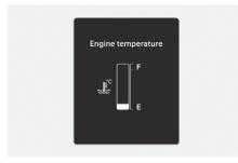
This engine coolant temperature gauge display shows the temperature of the engine coolant when the engine is running.
