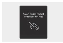
If the Driving Assist button, + switch, - switch or IIO switch is operated when Smart Cruise Control operating conditions are not satisfied, the "Smart Cruise Ctrl. conditions not met" will appear on the instrument cluster, and an audible warning will sound.
