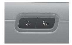
Integrated Memory System for the driver's seat is provided to store and recall the following memory settings with a simple button operation.
