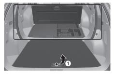
3. Open the emergency cable cover located in the cargo tray with a small blade tool (for example, screwdriver or similar) (2) and pull the emergency cable.
