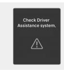
When Lane Following Assist is not working properly, the "Check Driver Assistance system." warning message will appear on the instrument cluster for several seconds, and the master (A) warning light appears on the instrument cluster. If this occur, have your vehicle inspected by an authorized HYUNDAI dealer.
