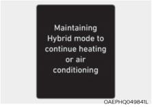
This message is displayed when the vehicle maintains the HEV mode to allow heating or air conditioning. The mode does not change when the driver presses the [HEV] button to switch from the HEV mode to EV mode while the heating and cooling system is on and the coolant temperature is below -14°C (7°F).
