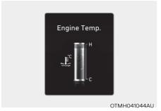
This engine coolant temperature gauge display shows the temperature of the engine coolant when the engine is running.
