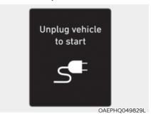
This message is displayed when you start the engine without unplugging the charging cable. Unplug the charging cable, and then start the vehicle.
