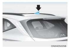
The shark fin antenna receives transmitted data. (for example: AM/FM, GPS)
