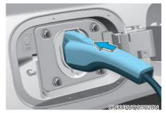
7. Hold the charging connector handle and connect it to the vehicle AC charging inlet. Push the connector until you hear a "clicking" sound. If the charging connector and charging terminal are not connected properly. this may cause a fire.
