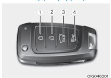
Your HYUNDAI uses a remote key, which you can use to lock or unlock the driver and passenger doors or the tailgate.
