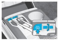
Press the DRIVE/TERRAIN button to change from normal driving mode to multi terrain mode. After the button is pressed, rotate the knob within 4 seconds to select SNOW, MUD or SAND.
