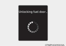
This message is displayed when you attempt to unlock the fuel filler door with the fuel tank pressurized. Wait until the fuel tank is depressurized.
