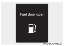
This message is displayed when thefuel filler door opens after the fuel tank is depressurized. If this message is displayed, you can refuel the fuel tank.
