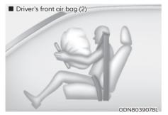
Upon deployment, tear seam molded directly into the pad cover will separate under pressure from the expansion of the air bags. Further opening of the covers allows full inflation of the air bags.
