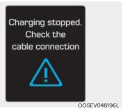
This warning message is displayed when charging is stopped because the charging connector is not correctly connected to the charging inlet
