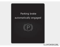
Parking brake automatically engaged When the EPB is applied from Auto Hold, a warning will sound and a message will appear.
