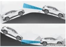
Blind-Spot Collision-Avoidance Assist may not operate properly when driving on an inclined road. The function may not detect the vehicle in the next lane or may incorrectly detect the ground or structure.
