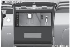
If 'Top View Parking Guidance' is selected, the parking guideline appears on the right side of the Surround View Monitor screen when the front top view and rear top view is displayed.
