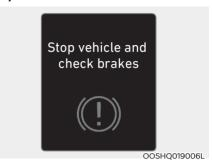
This message is displayed when a failure occurs in the brake system.
