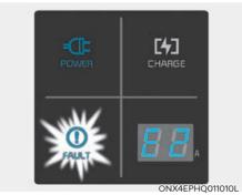
A leakage current occurs with "E2" error code (Power indicator: green ON, Fault indicator: red blink, E2 displayed)
