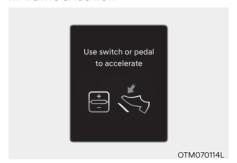
In traffic, your vehicle will stop if the vehicle ahead of you stops. Also, if the vehicle ahead of you starts moving, your vehicle will start as well. In addition, after the vehicle has stopped and a certain time have passed, the 'Use switch or pedal to accelerate' message will appear on the cluster. Depress the accelerator pedal or operate the + switch, - switch or IIO switch to start driving.
