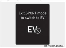
This message is displayed when [HEV] button is pressed but it is impossible to switch from the HEV mode to EV mode because the SPORT mode is engaged.
