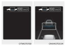
If you press the accelerator pedal above a certain speed while Smart Cruise Control is operating, the vehicle can be speeded up temporarily without altering the set speed. The set speed, distance level and target distance will blink on the cluster. However, if the accelerator pedal is depressed insufficiently, the vehicle may decelerate.
