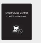
If the Driving Assist button, + switch. - switch or **II** switch is pushed when Smart Cruise Control's operating conditions are not satisfied, the 'Smart Cruise Control conditions not met' will appear on the cluster, and an audible warning will sound.
