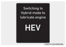
This message is displayed when the vehicle is automatically switched to the HEV mode to lubricate engine while the ignition switch is in the ON position.
