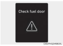
The message is displayed when the fuel filler door is open while in driving or an abnormality has occurred.
