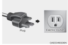
Charging a plug-in hybrid vehicle at home can stress the household electrical system more than a typical household appliance. Most modern residential electrical circuits are rated at 15 or 20 amps. The portable charger is rated to supply a 12A continuous load. To avoid tripping a fuse or breaker in the household, the portable charger charging rate can be reduced. Follow the steps below to set the charging rate of the portable charger.
