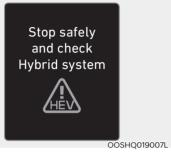
This message is displayed when there is a problem with the hybrid control system. The " "" indicator will blink and a warning chime will sound for approximately 10 seconds until the problem is solved. Refrain from driving when the warning message is displayed. If this occurs, have the vehicle inspected by an authorized HYUNDAI dealer.
