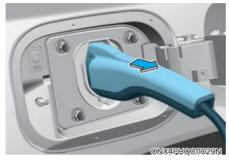
1. Hold the charging connector handle and pull it while pressing the release button
