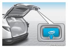
Press the power tailgate inner button for approximately one second when the tailgate is opened.
