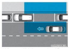
While your vehicle is stopped, and if Safe Exit Warning detects a vehicle approaching the rear corner of your vehicle and a passenger opens a door, Safe Exit Warning may warn you with a warning message and a warning sound to help avoid a collision.
