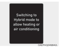
This message is displayed when the vehicle automatically switches to HEV mode to allow heating or air conditioning. It is when the coolant temperature is low (below -14°C (7°F)) and the driver turns on the heating or cooling system.
