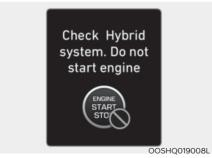
This message is displayed when the hybrid battery power (SOC) level is low. A warning chime will sound until the problem is solved. Refrain from driving when the warning message is displayed. If this occurs, have the vehicle inspected by an authorized HYUNDAI dealer.
