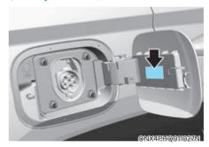
Charging label is located on the charging inlet cover's inside. For more details, refer to "Charging the plug-in hybrid vehicle" in the chapter 1.
