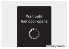
This message is displayed when you attempt to open the fuel filler door with the fuel tank pressurized. Wait until the fuel tank is depressurized.
