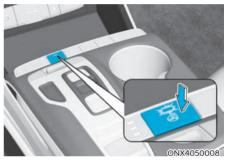
When the Engine Start/Stop is in the ON position or when the engine is running, press the heated steering wheel button to warm the steering wheel.
