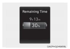
10. After charging has started, the estimated charging time is displayed on the instrument cluster for about 1 minute.
