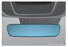
The electric rearview mirror automatically controls the glare from the headlight of the vehicle behind you in nighttime or low light driving conditions.
