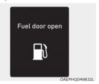
This message is displayed when the fuel filler door opens after the fuel tank is depressurized. If this message is displayed, you can refuel the fuel tank.
