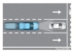
Forward Collision-Avoidance Assist detects a vehicle, a pedestrian, or a cyclist ahead on the road and may warn you of a possible collision with a warning message on the instrument cluster and a warning sound. Also, Forward Collision-Avoidance Assist may assist with braking your vehicle to help reduce collision speed or avoid a collision.
