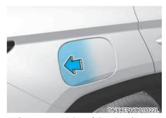
5. Press center edge of the charging door to open the charging door.
