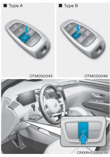
When the tailgate is closed, press the power tailgate open/close button for 1 second. The power tailgate opens with a warning sound.
