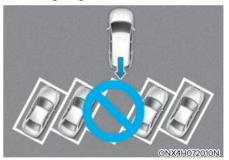
Remote Operation may not operate provide properly in a diagonal parking space.
