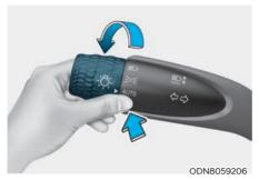
High Beam Assist automatically controls the headlights between high beam and low beam depending on the detected ambient light, such as an oncoming vehicle or leading vehicle.
