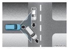
When a vehicle ahead disappears at an intersection, your vehicle may accelerate.
