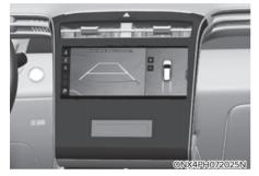
Surround View Monitor uses the wide view cameras and displays images around your vehicle through the infotainment system screen to help with safe parking or driving.
