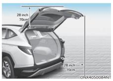
Make sure there are no people or objects around the tailgate before operating the power tailgate. Wait until the tailgate is opened fully and stopped before loading or unloading cargo or passengers from the vehicle.
