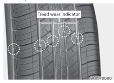
If the tire is worn evenly, a tread wear indicator will appear as a solid band across the tread. This shows there is less than 1.6 mm (1/16 in.) of tread left on the tire. Replace the tire when this happens.
