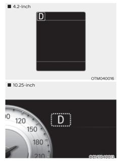
The Transmission Shift Indicator is shown in the upper corner of the cluster display to indicate the current gear or Park(P).
