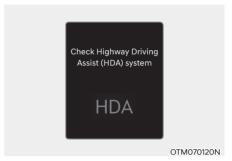
When Highway Driving Assist or Highway Lane Change function is not working properly, the 'Check Highway Driving Assist (HDA) system' warning message will appear, and the Awarning light will illuminate on the cluster. Have the vehicle inspected by an authorized HYUNDAI dealer.
