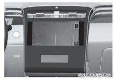
Press the icon. The top view appears on the screen and the distance from the vehicle appears in the back of your vehicle.
