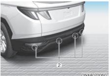
[1]: Wide-rear view camera, [2]: Rear ultrasonic sensors
