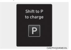
This message is displayed when the charging connector is plugged with the shift lever in R (Reverse), N (Neutral) or D (Drive). Move the shift lever to P (Park) and re-start the charging process.
