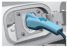
5. Hold the charging connector handle and connect it to the vehicle AC charging inlet. Push the connector until you hear a "clicking" sound. If the charging connector and charging terminal are not connected properly, this may cause a fire.
