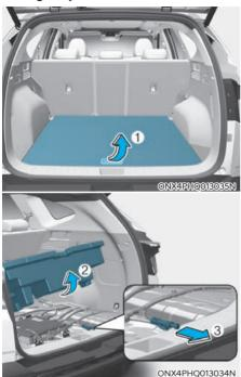
If the charging connector does not disconnect due to battery discharge and electric wire failure, perform the following:
