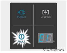
Before plugging charging connector into vehicle (Power indicator : green ON, Fault indicator : red blink)
