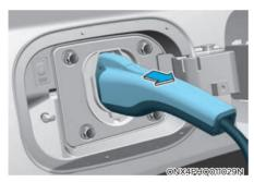
2. Hold the charging connector handle and pull it while pressing the release button.
