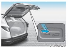
Your vehicle is equipped with the emergency tailgate safety release lever located on the bottom of the tailgate.
