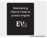
This message is displayed when the [HEV] button is pressed but it is impossible to switch from the HEV mode to EV mode due to engine lubrication.
