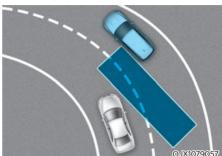
Blind-Spot Collision-Avoidance Assist may not operate properly when driving on a curved road. The function may not detect the vehicle in the next lane.
