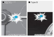
Check if the charging indicator light of the high voltage battery on the instrument cluster is turned ON. Charging is not done when the charging indicator lamp is OFF.
