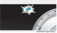
Check if the charging indicator light (\$\square\$) of the high voltage battery in the instrument cluster is turned ON. Charging is not active when the charging indicator light (\$\square\$) is OFF.
