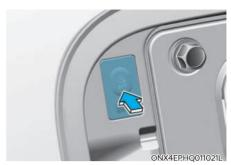
If you press the scheduled charging deactivation (\$\mathbb{C}\$) button to immediately charge the battery, charging must be initiated 3 minutes after the charging cable has been connected. When you press the scheduled charging deactivation (\$\mathbb{C}\$) button for immediate charging, the scheduled charge setting is not completely deactivated. If you need to completely deactivate the scheduled charge setting, use the infotainment system to finalize the deactivation.
