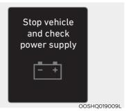
This message is displayed when a failure occurs in the power supply system.
