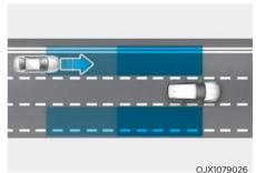
Blind-Spot Collision-Avoidance Assist helps detect and informs the driver that a vehicle is approaching at high speed from the blind spot area.
