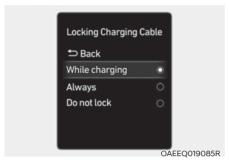
You may select when the charging connector can be locked and unlocked in the charging inlet.
