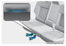
The hybrid battery cooling duct is located of the Passenger's seat (Left hand-driver) and Driver's seat (Right hand-driver). The cooling duct cools down the hybrid battery. When the hybrid battery cooling duct is blocked, the hybrid battery may be overheated.
