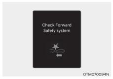
When Forward Collision-Avoidance Assist is not working properly, the 'Check Forward Safety system' warning message will appear, and the /\(\Lambda\) and \(\preceq\) warning lights will illuminate on the cluster. Have the vehicle inspected by an authorized HYUNDAI dealer.
