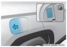
When charging the high voltage battery, the charge level can be checked from outside the vehicle.
