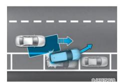
When you are driving forward out of a parking space, if Blind-Spot Collision-Avoidance Assist judges that there is a collision risk with an approaching vehicle in the blind spot, it will help avoid a collision by applying the brake.
