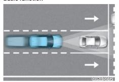
Forward Collision-Avoidance Assist detects a vehicle, a pedestrian, or a cyclist ahead on the road and may warn you of a possible collision with a warning message on the instrument cluster and a warning sound. Also, Forward Collision-Avoidance Assist may assist with braking your vehicle to help reduce collision speed or avoid a collision.
