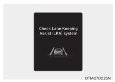
When Lane Keeping Assist is not working properly, the 'Check Lane Keeping Assist (LKA) system' warning message will appear and the yellow / indicator light will illuminate on the cluster. If this occurs, have the vehicle inspected by an authorized HYUNDAI dealer.
