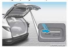
Your vehicle is equipped with the emergency tailgate safety release lever located on the bottom of the tailgate. When someone is inadvertently locked in the luggage compartment, the tailgate can be opened by moving the lever in the direction of the arrow and pushing the tailgate open.
