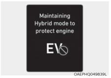
This message is displayed when the [HEV] button is pressed but it is impossible to switch from the HEV mode to EV mode due to engine lubrication.
