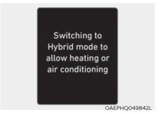
This message is displayed when the vehicle automatically switches to HEV mode to allow heating or air conditioning. It is when the coolant temperature is low (below -14°C (7°F)) and the driver turns on the heating or cooling system.
