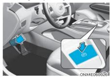
To release EPB (Electronic Parking Brake):
