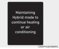
This message is displayed when the vehicle maintains the HEV mode to allow heating or air conditioning. The mode does not change when the driver presses the [HEV] button to switch from the HEV mode to EV mode while the heating and cooling system is on and the coolant temperature is below -14°C (7°F).
