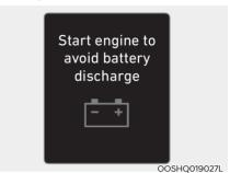
This message is displayed to inform the driver the 12V battery may be discharged if the ignition switch is in ON position (without the findicator ON).
