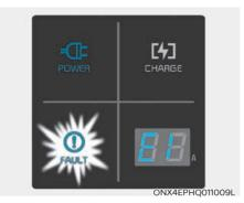
Plugged into vehicle (Power indicator: green ON, Fault indicator: red blink)
