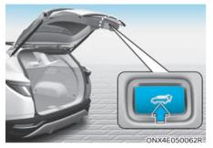
Press the power tailgate open/close button located inside the tailgate for more than 3 seconds.
