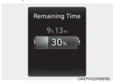
This message is displayed to notify the remaining time to fully charge the battery.
