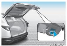
Lower the tailgate lid and press down until it locks. To be sure the tailgate lid is securely fastened, always check by trying to pull it up again without pressing the tailgate handle button.
