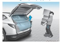
On a vehicle equipped with a smart key, the tailgate can be opened with handsfree activation using the smart tailgate system.
