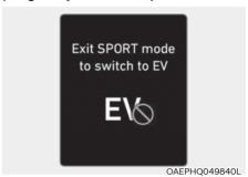
This message is displayed when [HEV] button is pressed but it is impossible to switch from the HEV mode to EV mode because the SPORT mode is engaged.
