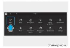
Press [PHEV] on the [Home] screen or the [All menus] screen and the menus related to plug-in hybrid ([ECO driving], [Energy information], [EV range], [Set charging times], [Charging stations],
