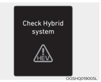
This message is displayed when there is a problem with the hybrid control system. Refrain from driving when the warning message is displayed.
