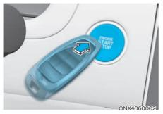
If the smart key battery is weak or the smart key does not work correctly, you can start the vehicle by pressing the Engine Start/Stop button with the smart key in the direction of the picture above.
