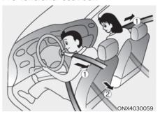
Your vehicle is equipped with driver's and front passenger's Pre-tensioner Seat Belts(Retractor Pretensioner and Emergency Fastening Device System). The purpose of the pre-tensioner is to make sure the seat belts fit tightly against the occupant's body in certain frontal or side collision(s). The Emergency Fastening Device System may be activated in certain crashes where the frontal collision(s) is severe enough.
