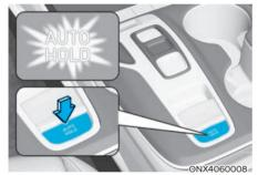
With the driver's door, engine hood and tailgate closed, then press the [AUTO HOLD] switch. The white AUTO HOLD indicator will come on and the system will be in the standby position.
