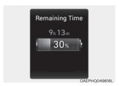
After charging has started, the estimated charging time is displayed on the instrument cluster for about 1 minute.
