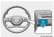
With the engine on, press and hold the Lane Driving Assist button located on the steering wheel to turn on Lane Keeping Assist. The white or green indicator light will illuminate on the cluster.
