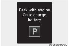
This message is displayed when the hybrid battery power (SOC) level is low. If this occurs, park the vehicle in a safe
