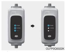
9. Charging starts automatically. Check if the power lamp and charging lamp (orange) are ON.
