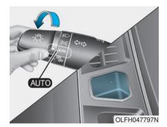
Adaptive front lighting system uses the steering angle and vehicle speed to help maximize your field of vision by swiveling and leveling the headlamp.
