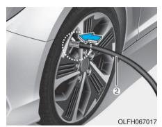
4. Unscrew the valve cap from the valve of the flat tire and screw the filling hose (2) of the sealant bottle onto the valve.
