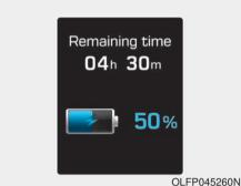
8. After charging has started, the estimated charging time is displayed on the instrument cluster for about 1 minute. It is also displayed, when the driver's door is opened with charging in progress. When scheduled charging is set, the estimated charging time is displayed as "--".
