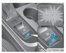
With the driver's door and the engine hood closed, fasten the driver's seat belt or depress the brake pedal and then press the [AUTO HOLD] switch. The white "AUTO HOLD" indicator will come on and the system will be in the standby position.
