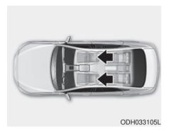
The vehicle's front seats are equipped with adjustable head restraints for both safety and comfort.
