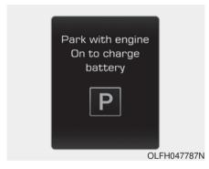
The message is displayed when the charging connector is plugged with the shift lever in R (Reverse), N (Neutral) or D (Drive). Move the shift lever to P (Park) and re-start the charging process.
