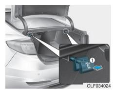
3. Pull on the backseat folding lever (1) located in the trunk.
