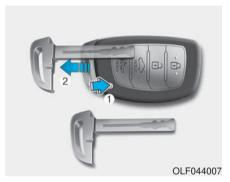
To remove the mechanical key from the smart key fob, press and hold the release button (1) and pull the mechanical key (2) out.
