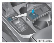
Pressing the HEV button changes the plug-in hybrid system modes, as below.
