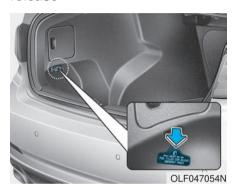
If the fuel filler door does not open using the remote fuel filler door release button, you can open it manually. Pull the handle of the release located on the left side of the luggage compartment outward slightly.
