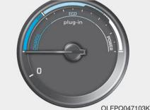
The hybrid system gauge indicates whether the current driving condition is fuel efficient or not.
