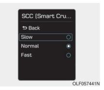
The sensitivity of vehicle speed when following the front vehicle to maintain the set distance can be adjusted. Go to the User Settings Mode (Driving Assist) and select SCC (Smart Cruise Control). You may select one of the three stages you prefer.
