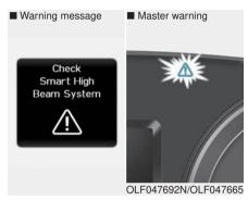
When the Smart High Beam Assist System is not working properly, the warning message will come on for a few second. After the message disappears, the master warning light will illuminate. Take your vehicle to an authorized HYUNDAI dealer and have the system checked.
