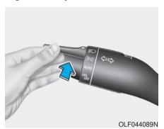
To turn on the high beam headlamp, push the lever away from you. The lever will return to its original position.
