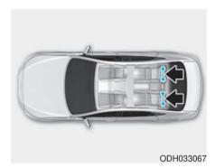
LATCH anchors have been provided in the left and right outboard rear seating positions. Their locations are shown in the illustration. There are no LATCH anchors provided for the center rear seating position.
