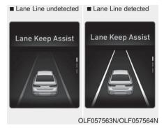
If the speed of the vehicle is over 40 mph (64 km/h) and the system detects lane markers, the color changes from gray to white.
