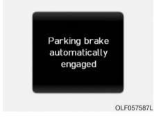
If the driver turns the hybrid system off while Auto Hold is operating, EPB will be automatically applied.
