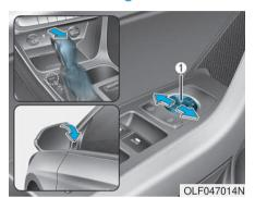
When you move the shift lever to the R (Reverse) position, the outside rearview mirror(s) will rotate downwards to aid with driving in reverse. The position of the outside rearview mirror switch (1) determines whether or not the mirrors will move:
