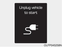
The message is displayed when you start the engine without unplugging the charging cable. Unplug the charging cable, and then start the vehicle.
