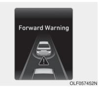
This initial warning message appears on the LCD display with a warning chime.
