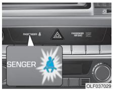
The front passenger's seat belt warning light will activate to the following table when the ignition switch is in "ON" position.
