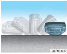
Front air bags may not inflate in rollover accidents because air bag deployment could not provide protection to the occupants.
