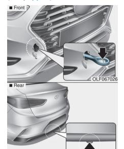
If towing is necessary, we recommend you to have it done by an authorized HYUNDAI dealer or a commercial tow truck service. If towing service is not available in an emergency, your vehicle may be temporarily towed using a cable or chain secured to the emergency towing hook at the rear of the vehicle.
