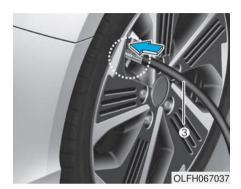
Unscrew the valve cap from the valve of the defective wheel and screw the filling hose (3) of the sealant bottle onto the valve.
