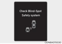
When Safe Exit Assist is not working properly, the 'Check Blind-Spot Safety system' warning message will appear on the cluster, and the system will turn off automatically or the system will be limited. We recommend that the system be inspected by an authorized HYUNDAI dealer.
