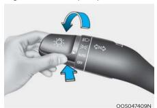
High Beam Assist is a system that automatically adjusts the headlamp range (switches between high beam and low beam) according to the brightness of other vehicles and road conditions.
