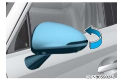
To fold the side view mirrors, grasp the housing of the mirror and then fold it inwards.
