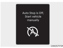
Start vehicle manually", appears on the LCD display with a beep sound, restart the vehicle manually by depressing the brake pedal with the vehicle shifted to P (Park) or N (Neutral). For your safety, restart the vehicle in the P (Park) position.
