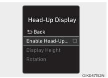
To activate the head up display, select 'Enable Head-Up Display' on the User Settings mode on the instrument cluster LCD display.
