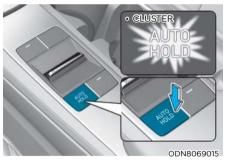
1. With the driver's door and engine hood closed, depress the brake pedal and then press the IAUTO HOLD] switch. The white AUTO HOLD indicator will come on and the system will be in the standby position.
