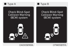
Check Blind-Spot Collision Warning (BCW) system
