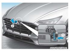
Go to the front of the vehicle, raise the hood slightly, push up the secondary latch (1) inside of the hood center and lift the hood (2). After it has been raised about halfway, it will raise completely by itself.
