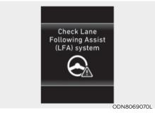
Check LFA (Lane Following Assist) system If there is a problem with the system a message will appear for a few seconds. If the problem continues LFA system failure indicator will illuminate.
