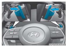
The paddle shifter is available when the gear is in the D (Drive) position.
