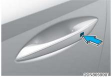
Press the button on the driver's outside door handle or touch the touch sensor on the door handle (the engraved part) while carrying the Smart Key with you or press the Door Unlock button on the Smart Key, the driver's door will unlock.
