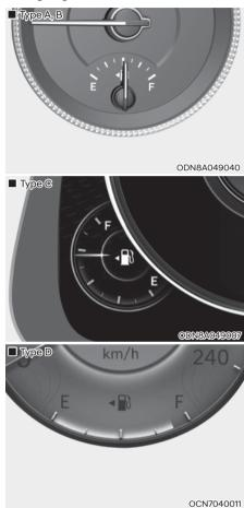
This gauge indicates the approximate amount of fuel remaining in the fuel tank.
