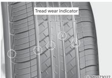
If the tire is worn evenly, a tread wear indicator will appear as a solid band across the tread. This shows there is less than 2/32 inch (1.6 mm) of tread left on the tire. Replace the tire when this happens.
