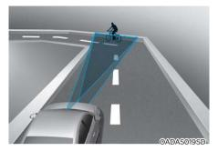
Forward Collision-Avoidance Assist system may recognize a vehicle or pedestrian or cyclist in the next lane or outside the lane when driving on a curved road.
