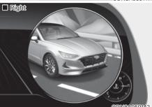
Blind-Spot View Monitor system displays the left or right side of the rear blind spot area of your vehicle in the instrument cluster when the left or right turn signal is on. This function helps you when changing lanes.
