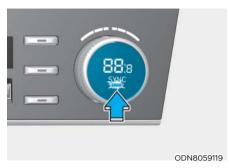
Adjusting the driver and passenger side temperature equally
