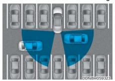
Rear Cross-Traffic Collision Warning system uses rear radar to monitor the approaching cross traffic from the left and right side of the vehicle when your vehicle is in reverse.
