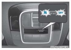
Your vehicle is equipped with an Occupant Classification System (OCS) in the front passenger's seat.
