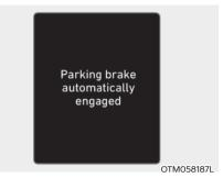
Parking brake automatically engaged When the EPB is applied from Auto Hold, a warning will sound and a message will appear.
