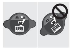
Make sure that the tiny protrusions inside the coolant cap is securely interlocked.
