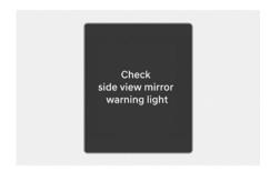
When the side view mirror warning light is not working properly, the "Check side view mirror warning light" warning message appears on the instrument cluster for several seconds, and the master (A) warning light illuminates on the instrument cluster. If this occurs, have your vehicle inspected by an authorized HYUNDAI dealer.
