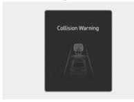
To warn the driver of a collision, the "Collision Warning" warning message appears and the (ﷺ) warning light blinks on the instrument cluster with a warning sound and the steering wheel vibrates.
