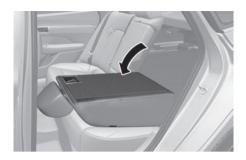
5. To use the rear seat, lift and pull the seatback rearward. Pull the seatback firmly until it clicks into place. Make sure the seatback is locked in place and return the rear seat belt to the proper position.
