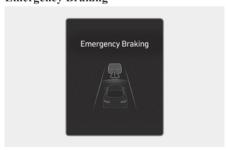
To warn the driver that emergency braking will be assisted, the "Emergency Braking" warning message appears and the (♣) warning light blinks on the instrument cluster with a warning sound and the steering wheel vibrates.
