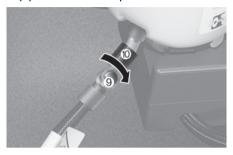
4. Connect the sealant bottle to the compressor.
