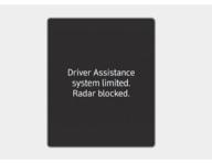
When the rear bumper around the rear corner radar or sensor is covered with foreign material, such as snow or rain, or installing a trailer or carrier, it can reduce the detecting performance and temporarily limit or disable Safe Exit Warning.
