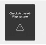
The active air flap system may not operate normally if the air flap is temporarily opened due to foreign factors or if the controller is contaminated by snow or rain, etc.
