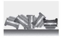
Front airbags may not inflate in rollover accidents because front airbag deployment would not provide additional occupant protection.
