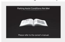
The "Parking Assist Conditions not met" message appears when Parking/View (P) button has been pressed and held while Remote Smart Parking Assist is in standby. After a while, press and hold the Parking/View (P) button again to see if Remote Smart Parking Assist works.
