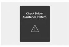
When Lane Keeping Assist is not working properly, the "Check Driver Assistance system." warning message and yellow Lane Keeping Assist (A) warning light appears on the instrument cluster. If this occurs, have your vehicle inspected by an authorized HYUNDAI dealer.
