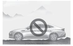
Remote Smart Parking Assist may cancel when the vehicle slips, or the vehicle cannot move due to road conditions such as pebbles or fragmented stones. · Parking behind a truck
