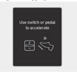
When Highway Driving Assist is operating, your vehicle will stop if the vehicle ahead of you stops. Also, if the vehicle ahead of you starts moving within 30 seconds after the stop, your vehicle will start as well. In addition, after the vehicle has stopped and 30 seconds have passed, the "Use switch or pedal to accelerate" message will appear on the instrument cluster. Depress the accelerator pedal or operate the + switch, - switch or (II'2) switch to start driving.
