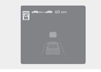
When driving at a speed higher than the displayed speed limit, the speed limit is displayed in red.
