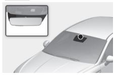
The Auto defogging reduces the possibility of fogging up the inside of the windshield by automatically sensing the moisture on inside the windshield.
