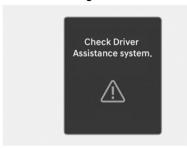
When Lane Following Assist is not working properly, the **Check Driver Assistance system.** warning message will appear on the instrument cluster for several seconds, and the master (△) warning light appears on the instrument cluster. If this occurs, have your vehicle inspected by an authorized HYUNDAI dealer.
