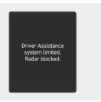
When the rear bumper around the rear corner radar or sensor is covered with foreign material, such as snow or rain, or installing a trailer or carrier, it can reduce the detecting performance and temporarily limit or disable Blind-Spot Collision-Avoidance Assist.
