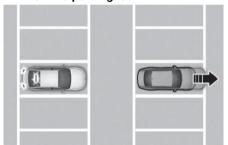
If a vehicle parked in front drives away from you, Leading Vehicle Departure Alert may alert you that the parked vehicle is driving away. When driving at a tollgate or intersection, etc.
