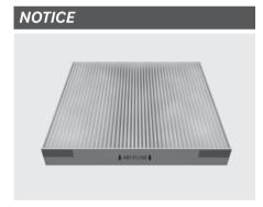
Install a new cabin air filter in the correct direction with the arrow symbol ( $\psi$ ) facing downwards, to prevent noise and efficiency loss.
