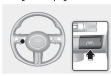
With the engine on, press and hold the Lane Driving Assist (/⊕\) button located on the steering wheel to turn on and off. When Lane Keeping Assist is on, the (/♠\) indicator is on.
