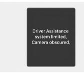
When the front windshield where the front view camera is located, or sensor is covered with foreign material, such as snow or rain, it can reduce the detecting performance and temporarily limit or disable Lane Keeping Assist.
