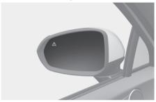
To warn the driver a vehicle is detected, the warning light on the side view mirror illuminates.
