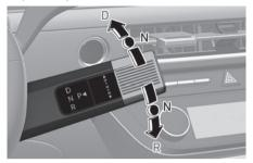
The wheels and transmission are not engaged.
