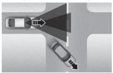
When a vehicle in front of you merges out of the lane, Smart Cruise Control may not immediately detect the new vehicle that is now in front of you.
