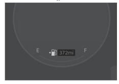
The distance to empty is the estimated distance the vehicle can be driven with the remaining fuel.
