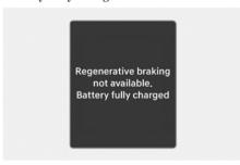
Regenerative braking is temporarily limited to protect the battery because the high voltage battery is fully charged.
