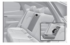
The armrest is located in the center of the rear seat. Pull the armrest down from the seatback to use it.
