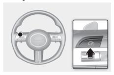
To turn Smart Cruise Control off, press the Driving Assist ( $\bigcap$ ) button.
