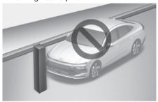
Remote Smart Parking Assist performance may reduce or collision with an obstacle may occur when there is a narrow object, circular pillar, square pillar, or a pillar surrounded by objects such as a fire extinguisher, etc., near the parking space. The driver should park the vehicle manually.
