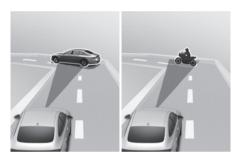
On curves, the smart recuperation system may not detect a vehicle in the same lane, and may accelerate the vehicle by lowering the regenerative braking intensity automatically. Your vehicle speed may decelerate by increasing regenerative braking intensity automatically if a vehicle is detected in an adjacent lane or when a vehicle ahead is detected suddenly. Apply the brake pedal or accelerator pedal depending on the road and driving conditions.
