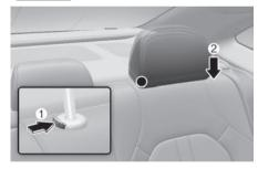
To reinstall the head restraint:
