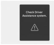
When Safe Exit Warning is not working properly, the "Check Driver Assistance system." warning message will appear on the instrument cluster for several seconds, and the master warning light (A) will appear on the instrument cluster. If this occurs, have your vehicle inspected by an authorized HYUNDAI dealer.
