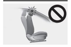
If you recline the seatback towards the front with the head restraint and seat cushion raised, the head restraint may come in contact with the sunvisor or other parts of the vehicle.
