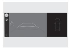
To warn the driver of an approaching vehicle from the rear left/right side of your vehicle, the warning light on the side view mirror blinks and a warning message appears on the instrument cluster. At the same time, an audible warning sounds and the steering wheel vibrates. A warning also appears on the infotainment system.
