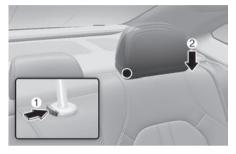
Route the seat belt webbing to the outward of the rear seat to prevent the belts from being damaged.
