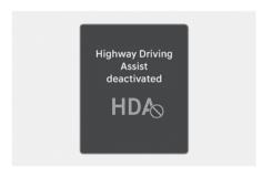
If the driver still does not have their hands on the steering wheel after the hands-off warning, "Highway Driving Assist deactivated" warning message will appear and Highway Driving Assist will be automatically canceled.
