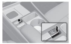
Press the Parking Safety (P<sub>m</sub>) button to turn on Parking Distance Warning. Press the button again to turn off the function.
