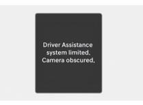
When the front windshield where the front view camera is located is covered with foreign material, such as snow or rain, it can reduce the detecting performance and temporarily limit or disable Intelligent Speed Limit Assist. If this occurs, the "Driver Assistance system limited. Camera obscured." warning message and the speed limit ( $\square$ ) warning light will appear on the instrument cluster.
