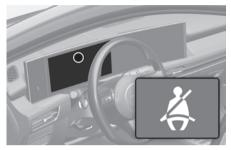
As a reminder to the driver, the driver's seat belt warning light illuminates for about 6 seconds each time the Engine Start/Stop button is in the ON position regardless of seatbelt fastening.
