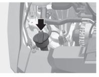
Check the fluid level in the washer fluid reservoir and add fluid if necessary. Plain water may be used if washer fluid is not available. However, use washer solvent with antifreeze characteristics in cold climates to prevent freezing.
