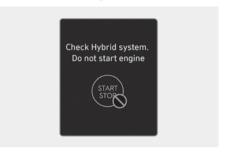
This message appears when the hybrid battery power (SOC) level is low. A warning chime will sound until the problem is solved. Refrain from driving when the warning message appears. If this occurs, we recommend that your vehicle be inspected by an authorized HYUNDAI dealer.
