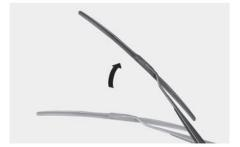
3. Lift up the wiper blade clip (1). Then pull down the wiper blade (2). Remove the wiper blade from the wiper arm.
