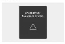
When Intelligent Speed Limit Assist is not working properly, the "Check Driver Assistance system." warning message will appear on the instrument cluster for several seconds, and the master (△) warning light and speed limit (□) warning light will appear on the instrument cluster. If this occurs, have your vehicle inspected by an authorized HYUNDAI dealer.
