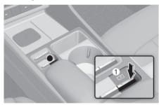
Press the Parking/View button (1) while the gear is in P (Park) to turn on the Rear View Monitor.
