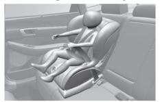
A forward-facing Child Restraint System provides restraint for the child's body with a harness. Keep children in a forward-facing Child Restraint System with a harness until they reach the top height or weight limit allowed by your Child Restraint System's manufacturer.
