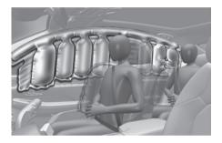
Curtain airbags are located along both sides of the roof rails above the front and rear doors.
