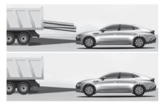
When the vehicle in front of the foregoing vehicle is at a stop and the foregoing vehicle changes the lane, the front sensors may be unable to recognize the stopped vehicle.
