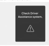
When Blind-Spot Collision-Avoidance Assist is not working properly, the "Check Driver Assistance system." warning message will appear on the instrument cluster for several seconds, and the master (A) warning light will appear on the instrument cluster. If this occurs, have your vehicle inspected by an authorized HYUNDAI dealer.
