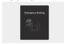
To warn the driver that emergency braking will be assisted, the "Emergency Braking" warning message appears and the (♣) warning light blinks on the instrument cluster with a warning sound and the steering wheel vibrates.
