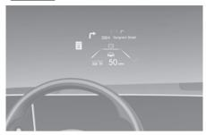
The Head-Up Display is an optional feature that allows the driver to view information projected onto a transparent screen while still keeping your eyes on the road ahead while driving.
