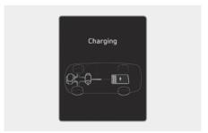
The engine braking is simultaneously used to decelerate the vehicle and to charge up the high voltage battery.
