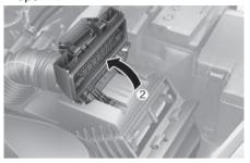
3. Rotate the fixed lever (3) on the filter and loosen the lock.
