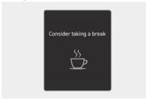
The "Consider taking a break" message will appear and the inattentive driving (\(\frac{\top}{\top}\)) warning light will blink on the instrument cluster with a warning sound to suggest that the driver take a break, when the driver's attention level is below a certain level.
