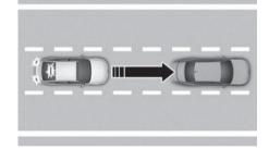
If the vehicle in front abruptly departs, Leading Vehicle Departure Alert may not operate properly.  When a pedestrian or bicycle is between you and the vehicle ahead
