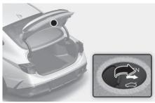
Your vehicle is equipped with the emergency trunk safety release lever located on the bottom of the trunk.
