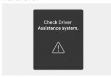
When Driver Attention Warning is not working properly, the "Check Driver Assistance system." warning message will appear on the instrument cluster for several seconds, and the master (A) warning light and the inattentive driving (b) warning light will appear on the instrument cluster. If this occurs, have your vehicle inspected by an authorized HYUNDAI dealer.
