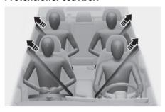
Your vehicle is equipped with driver's, front passenger's and rear passengers pretensioner seat belts (retractor pretensioner). The pretensioner makes sure the seat belts fit tightly against your body in certain frontal or side collision(s). The pretensioner seat belts may be activated in some crashes where the frontal or side collision(s) is severe enough, together with the airbags.
