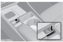
Press and hold the Parking Safety (P<sub>\*\*</sub>) button more than 2 seconds, to turn the Parking Collision-Avoidance Assist on or off.
