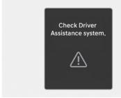
When Highway Driving Assist is not working properly, the "Check Driver Assistance system." warning message and yellow Lane Keeping Assist (/=\) warning light appears on the instrument cluster. If this occurs, have your vehicle inspected by an authorized HYUNDAI dealer.
