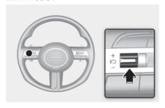
Press the (IIO) switch to temporarily pause the set speed limit. The set speed limit will turn off but the Speed Limit (STLIMIT) indicator will stay on.
