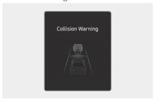
To warn the driver of a collision, the "Collision Warning" warning message appears and the (♣) warning light blinks on the instrument cluster with a warning sound and the steering wheel vibrates.
