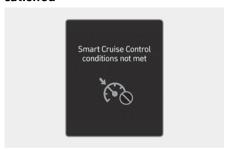
If the Driving Assist button, + switch, - switch or (II'D) switch is operated when Smart Cruise Control operating conditions are not satisfied, the "Smart Cruise Control conditions not met" will appear on the instrument cluster, and an audible warning will sound.
