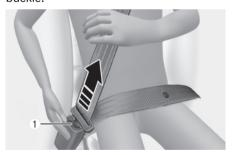
Once released, the belt should automatically draw back into the retractor. If this does not happen, check the belt to be sure it is not twisted, then try again.
