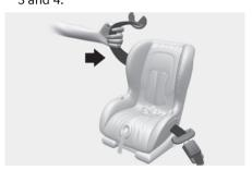
5. Remove as much slack from the belt as possible by pushing down on the Child Restraint System while feeding the shoulder belt back into the retractor.
