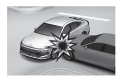
Front airbags may not inflate in side impact collisions, because occupants move in the direction of the collision. Side and curtain airbags may inflate depending on the severity of impact.
