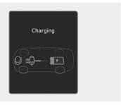
The engine charges up the high voltage battery. The motor power is used to drive the vehicle.
