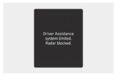
When the rear bumper around the rear-side radar or sensor is covered with foreign material, such as snow or rain, or installing a trailer or carrier, it can reduce the detecting performance and temporarily limit or disable Rear Cross-Traffic Collision-Avoidance Assist.
