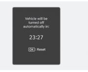
When all the conditions are satisfied, the Vehicle Auto-Shut Off operates and turns the engine off automatically after 60 minutes.
