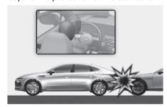
Front airbags are not designed to inflate in rear collisions, because occupants are moved backward by the force of the impact.
