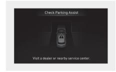
When Remote Smart Parking Assist is not working properly, the "Check Parking Assist" warning message will appear on the infotainment system. If the message appears, stop using Remote Smart Parking Assist, and we recommend that your vehicle be inspected by an authorized HYUNDAI dealer.
