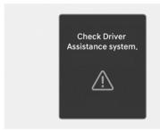
When High Beam Assist is not working properly, the "Check Driver Assistance system" warning message may appear, and the Awarning light may illuminate on the instrument cluster. Have the system inspected by an authorized HYUNDAI dealer.
