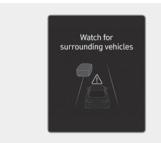
In the following situation, the "Watch for surrounding vehicles" warning message will appear on the instrument cluster, and an audible warning will sound to warn the driver of road conditions ahead.
