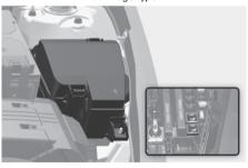
Pull the suspected fuse straight out. Use the removal tool (1) provided in the engine compartment fuses panel cover.
