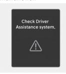
When Blind-Spot Collision-Avoidance Assist is not working properly, the "Check Driver Assistance system." warning message will appear on the instrument cluster for several seconds, and the master (A) warning light will appear on the instrument cluster. If this occurs, have your vehicle inspected by an authorized HYUNDAI dealer.
