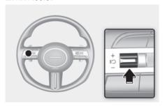
Press the (IIO) switch to temporarily pause the set speed limit. The set speed limit will turn off but the Speed Limit (STLIMIT) indicator will stay on.
