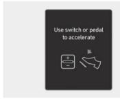
In traffic, your vehicle will stop if the vehicle ahead of you stops. Also, if the vehicle ahead of you starts moving, your vehicle will start as well. In addition, after the vehicle has stopped and a certain time have passed, the "Use switch or pedal to accelerate" message will appear on the instrument cluster. Depress the accelerator pedal or operate the + switch, - switch or (IIO) switch to start driving.
