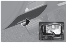
Refer to the label on the inside of the fuse panel cover to locate the suspected fuse location.
