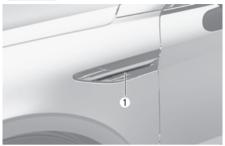
If the side repeater light (1) does not operate, have the system inspected by an authorized HYUNDAI dealer.
