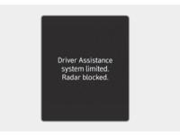
When the rear bumper around the rear corner radar or sensor is covered with foreign material, such as snow or rain, or installing a trailer or carrier, it can reduce the detecting performance and temporarily limit or disable Safe Exit Warning.
