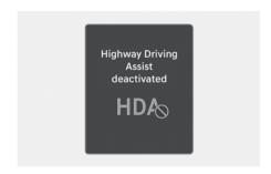
If the driver still does not have their hands on the steering wheel after the hands-off warning, "Highway Driving Assist deactivated" warning message will appear and Highway Driving Assist will be automatically canceled.
