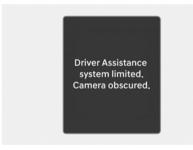
When the front windshield where the front view camera is located, or sensor is covered with foreign material, such as snow or rain, it can reduce the detecting performance and temporarily limit or disable Lane Keeping Assist.
