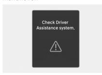
When Intelligent Speed Limit Assist is not working properly, the "Check Driver Assistance system." warning message will appear on the instrument cluster for several seconds, and the master (⚠) warning light and speed limit (☐) warning light will appear on the instrument cluster. If this occurs, have your vehicle inspected by an authorized HYUNDAI dealer.
