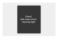
When the side view mirror warning light is not working properly, the "Check side view mirror warning light" warning message will appear on the instrument cluster for several seconds, and the master warning light (A) will appear on the instrument cluster. If this occurs, have your vehicle inspected by an authorized HYUNDAI dealer.
