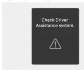
When Highway Driving Assist is not working properly, the "Check Driver Assistance system." warning message and yellow Lane Keeping Assist (A) warning light appears on the instrument cluster. If this occurs, have your vehicle inspected by an authorized HYUNDAI dealer.
