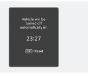
When all the conditions are satisfied, the Vehicle Auto-Shut Off operates and turns the engine off automatically after 60 minutes.
