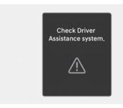
When Lane Keeping Assist is not working properly, the "Check Driver Assistance system." warning message and yellow Lane Keeping Assist (A) warning light appears on the instrument cluster. If this occurs, have your vehicle inspected by an authorized HYUNDAI dealer.
