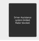
When the front radar cover or sensor is covered with snow, rain, or foreign material, it can reduce the detecting performance and temporarily limit or disable Smart Cruise Control.
