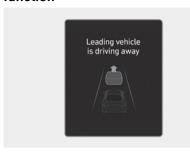
When a detected vehicle in front departs from a stop, Leading Vehicle Departure Alert will inform the driver by displaying the "Leading vehicle is driving away" message on the instrument cluster and an audible warning will sound.
