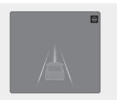
If the vehicle ahead and/or both lane markings are detected and your vehicle speed is below 120 mph (200 km/h), the green (②) indicator light appears on the instrument cluster, and Lane Following Assist helps center the vehicle in the lane by assisting the steering wheel.
