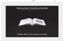
The "Parking Assist Conditions not met" message appears when Parking/View (EP) button has been pressed and held while Remote Smart Parking Assist is in standby. After a while, press and hold the Parking/View (EP) button again to see if Remote Smart Parking Assist works.
