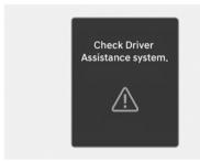
When Smart Cruise Control is not working properly, the "Check Driver Assistance system." warning message and the master (A) warning light will appear on the instrument cluster. Have your vehicle inspected by an authorized HYUNDAI dealer.
