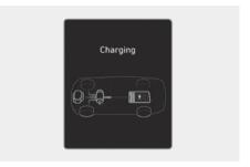
The engine and regenerative brake system charges up the high voltage battery. (Engine and Wheel → Battery)
