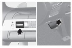
Press the (IIO) switch or depress the brake pedal to temporarily cancel Smart Cruise Control.
