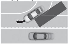
Blind-Spot Collision-Avoidance Assist may not operate properly when driving where the road merges or divides. The function may not detect the vehicle in the next lane.
