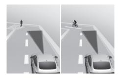
Forward Collision-Avoidance Assist may not detect a vehicle, a powered two-wheeler, a pedestrian, or a cyclist in front of you when driving on curved roads adversely affecting the performance of the sensors. This may result in no warning, braking assist when necessary.
