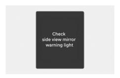
When the side view mirror warning light is not working properly, the "Check side view mirror warning light" warning message appears on the instrument cluster for several seconds, and the master (A) warning light illuminates on the instrument cluster. If this occurs, have your vehicle inspected by an authorized HYUNDAI dealer.
