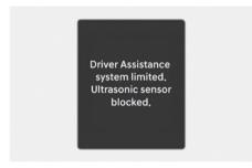
The "Driver Assistance system limited. Camera blocked." or "Driver Assistance system limited. Ultrasonic sensor blocked." warning message will appear on the cluster if the following situations occur:
