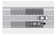
Blind-Spot Collision-Avoidance Assist helps detect and informs the driver that a vehicle is in the blind spot.
