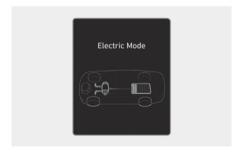
Only the motor power is used to drive the vehicle. (Battery → Wheel)
