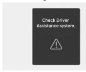
When Lane Following Assist is not working properly, the **Check Driver Assistance system.** warning message will appear on the instrument cluster for several seconds, and the master (△) warning light appears on the instrument cluster. If this occurs, have your vehicle inspected by an authorized HYUNDAI dealer.
