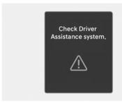
When Safe Exit Warning is not working properly, the "Check Driver Assistance system." warning message will appear on the instrument cluster for several seconds, and the master warning light (A) will appear on the instrument cluster. If this occurs, have your vehicle inspected by an authorized HYUNDAI dealer.
