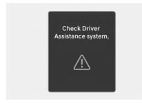
When Driver Attention Warning is not working properly, the "Check Driver Assistance system." warning message will appear on the instrument cluster for several seconds, and the master (A) warning light and the inattentive driving (D) warning light will appear on the instrument cluster. If this occurs, have your vehicle inspected by an authorized HYUNDAI dealer.
