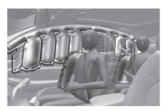
Side and curtain airbags are designed to inflate when an impact is detected by side collision sensors depending on the severity of impact resulting from a side impact collision.
