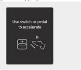
When Highway Driving Assist is operating, your vehicle will stop if the vehicle ahead of you stops. Also, if the vehicle ahead of you starts moving within 30 seconds after the stop, your vehicle will start as well. In addition, after the vehicle has stopped and 30 seconds have passed, the "Use switch or pedal to accelerate" message will appear on the instrument cluster. Depress the accelerator pedal or operate the + switch, - switch or (II'2) switch to start driving.
