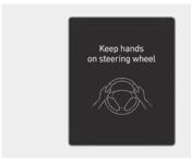
If the driver takes their hands off the steering wheel for several seconds, the "**Keep hands on steering wheel**" warning message appears on the instrument cluster, and an audible warning sounds in stages.
