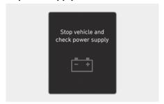
This message appears when a failure occurs in the power supply system. If this occurs, we recommend that your vehicle be inspected by an authorized HYUNDAI dealer.
