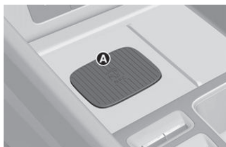
[A] Vehicle authentication pad (Wireless charging pad)
