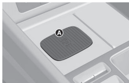
[A] Vehicle authentication pad (wireless charging pad)
