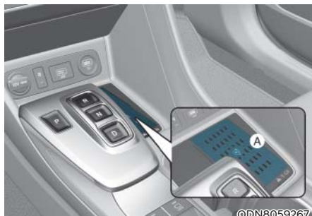
[A] : Wireless Charging Pad (In-vehicle Authentication Pad)
