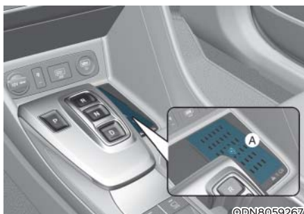
[A] : Wireless Charging Pad (In-vehicle Authentication Pad)
