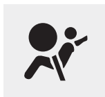
SRS warning light
