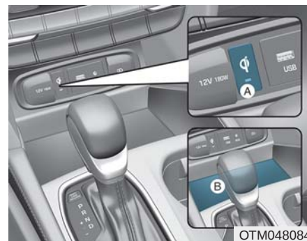
[A]: Indicator light, [B]: Charging pad
