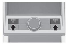
While the vehicle is running, press the switch to warm the driver's seat or front passenger's seat.
