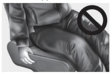
Do not use car seat accessories such as thick blankets and cushions which cover up the car seat surface.
