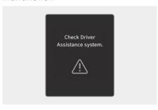
When Intelligent Speed Limit Assist is not working properly, the "Check Driver Assistance system." warning message will appear on the instrument cluster for several seconds, and the master (△) warning light and (□) warning light will illuminate on the instrument cluster. If this occurs, have your vehicle inspected by an authorized HYUNDAI dealer.
