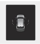
This warning appears if any door or hood or liftgate is left open. The warning indicates which door is open on the cluster display.
