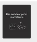
In traffic, your vehicle will stop if the vehicle ahead of you stops. Also, if the vehicle ahead of you starts moving, your vehicle will start as well. In addition, after the vehicle has stopped and a certain time have passed, the "Use switch or pedal to accelerate" message will appear on the instrument cluster. Depress the accelerator pedal or operate the + switch, - switch or IIO switch to start driving.
