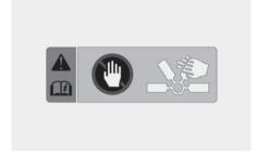
When using the V2L, the cooling fan in the vehicle motor compartment can operate automatically even if the vehicle is turned off. Do not put your hand near the cooling fan when the V2L is operating.
