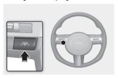
With the vehicle on, press and hold the Lane Driving Assist button (/⊕\) located on the steering wheel to turn on Lane Keeping Assist. The (/═\) indicator light illuminates on the instrument cluster.
