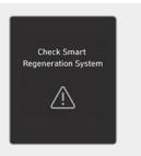
When the front radar is covered or blocked, the smart regeneration system may be temporarily disabled. The "Check Smart Regeneration System" warning message may appear, and the regenerative braking level is displayed on the instrument cluster.
