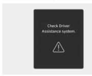
When Safe Exit Warning is not working properly, the "Check Driver Assistance system." warning message will appear on the instrument cluster for several seconds, and the master (△) warning light will appear on the instrument cluster. If this occurs, have your vehicle inspected by an authorized HYUNDAI dealer.
