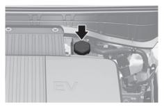
Check the fluid level in the reservoir periodically. The fluid level should be between MAX and MIN marks on the side of the reservoir.
