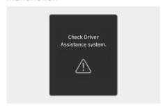
When Forward Collision-Avoidance Assist is not working properly, the **Check Driver Assistance system.** warning message will appear, and the warning lights will illuminate on the instrument cluster. Have your vehicle inspected by an authorized HYUNDAI dealer.
