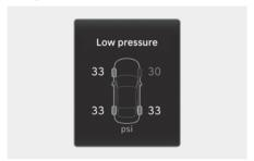
The tire pressure of each tire is displayed. For more information, refer to the "Tire Pressure Monitoring System (TPMS)" section in chapter 8.
