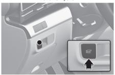
When the liftgate is closed, press the power liftgate open/close button for 1 second. The liftgate opens with a warning sound.
