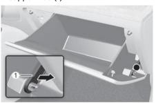
2. Press both sides of the glove box inward to release.
