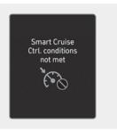
If the Driving Assist button, + switch, - switch or IIO switch is operated when Smart Cruise Control operating conditions are not satisfied, the "Smart Cruise Ctrl. conditions not met" will appear on the instrument cluster, and an audible warning will sound.
