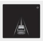
If the vehicle ahead and/or both lane markings are detected and your vehicle speed is below 120 mph (200 km/h), the green (♠) indicator light appears on the cluster, and Lane Following Assist helps center the vehicle in the lane by assisting the steering wheel.
