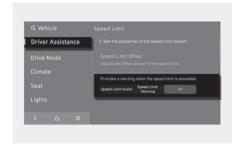
With the vehicle on, press the SETUP button and then select or deselect Vehicle > Driver Assistance > Speed Limit from the infotainment system to set whether to use each function.
