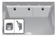
First secure the child restraint with the LATCH lower anchors or the seat belt. If the child restraint manufacturer recommends that the top tether strap be attached, attach and tighten the top tether strap to the top tether strap anchor.
