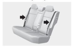
4. Pull up the seatback folding lever, then fold the seat toward the front of the vehicle.
