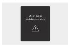
When Smart Cruise Control is not working properly, the "Check Driver Assistance system." warning message will appear, and the "A" warning light will illuminate on the instrument cluster. Have your vehicle inspected by an authorized HYUNDAI dealer.
