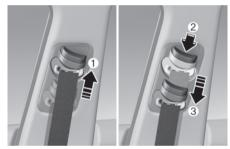
Pull it up (1) to raise the height. To lower it, push it down (3) while pressing the height adjuster button (2). Release the button to lock the anchor in place. Try pushing the height adjuster down to make sure that it is locked in place.
