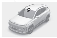
[A] Front view camera Refer to the illustration above for the detailed location of the detecting sensor.
