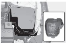
Inside the fuse panel cover, you can find the fuse label describing fuse names and ratings.
