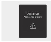
When Blind-Spot Collision Warning is not working properly, the "Check Driver Assistance system." warning message will appear on the instrument cluster for several seconds, and the master (△) warning light will appear on the instrument cluster. If this occurs, have your vehicle inspected by an authorized HYUNDAI dealer.
