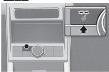
When the Start/Stop button is in the ON position or when the vehicle is in the ready mode (READY indicator ON), press the steering wheel heater button to warm the steering wheel. The indicator on the button illuminates.
