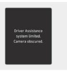
When the front windshield where the front view camera is located is covered with foreign material, such as snow or rain, it can reduce the detecting performance and temporarily limit or disable Intelligent Speed Limit Assist. If this occurs, the "Driver Assistance system limited. Camera obscured." warning message and ( $\boxminus$ ) warning light will appear on the instrument cluster.
