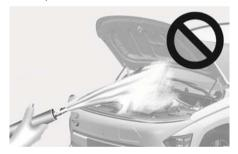
Never allow water or other liquids to come in contact with electrical/electronic components inside the vehicle as water or other liquids may flow in to the motor compartment through the front trunk and damage electrical/electronic components.
