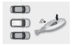
Press and hold the Remote Start button ( ) within 4 seconds until the vehicle starts.
