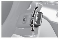
To shift the gear to N (Neutral), rotate the rotary shifter to N (Neutral) while depressing the brake pedal.
