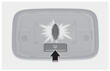
⊽: Press the button to turn on and off the rear room lamp.
