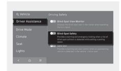
With the vehicle on, press the SETUP button, and then select Vehicle > Driver Assistance > Driving Safety > Blind-Spot Safety in the infotainment system to set whether to use each function.
