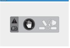
Keep hands, clothing, and tools away from the rotating fan blades of the cooling fan. The electric motor for the cooling fan may continue to operate or start up when the vehicle is off and can cause serious injury.
