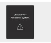
When Lane Following Assist is not working properly, the "Check Driver Assistance system." warning message will appear on the instrument cluster for several seconds, and the master (A) warning light appears on the instrument cluster. If this occur, have your vehicle inspected by an authorized HYUNDAI dealer.
