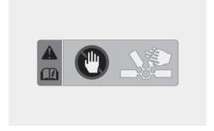
Do not put your hand near the cooling fan in the motor compartment while charging. It may operate automatically to control the battery temperature, even if the vehicle is turned off.
