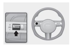
Press the II 2 switch to temporarily pause the set speed limit. The set speed limit will turn off but the Speed Limit (©'LIMIT) indicator will stay on.
