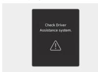
When Lane Keeping Assist is not working properly, the "Check Driver Assistance system." warning message appears and the yellow Lane Keeping Assist (/=\) indicator light illuminates on the instrument cluster. If this occurs, have your vehicle inspected by an authorized HYUNDAI dealer.
