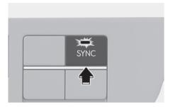
Adjusting the temperature, air flow direction, and fan speed equally
