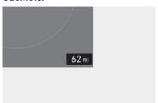
The odometer indicates the total distance that the vehicle has been driven and should be used to determine when periodic maintenance is required.
