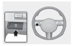
Press the button repeatedly to cycle through the headway settings from Distance  $4 \rightarrow$  Distance  $3 \rightarrow$  Distance  $2 \rightarrow$  Distance  $1 \rightarrow$  Distance  $4 \rightarrow$
