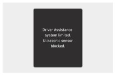
The "Driver Assistance system limited. Camera obscured." or "Driver Assistance system limited. Ultrasonic sensor blocked." warning message appears on the instrument cluster if the following situations occur:
