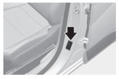
All specifications (sizes and pressures) can be found on a label attached to the driver's side center pillar.
