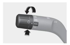
High Beam Assist automatically switches between high beam and low beam depending on the detected brightness from the lights of oncoming vehicles or vehicles in front.
