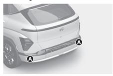
[A] Rear corner radar Refer to the illustration above for the detailed location of the detecting sensors.
