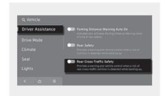
With the vehicle on, press the SETUP button, and then select Vehicle > Driver Assistance > Parking Safety > Rear-Cross Traffic Safety in the infotainment system to turn on Rear Cross-Traffic Collision-Avoidance Assist and deselect to turn off the function.
