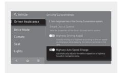
With the vehicle on, press the SETUP button and then select Vehicle > Driver Assistance > Driving Convenience > Highway Auto Speed Change from the infotainment system to turn on Navigation based Smart Cruise Control and deselect to turn off the function.
