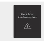
When High Beam Assist is not working properly, the "Check Driver Assistance system." warning message may appear, and the \(\text{\text{\text{\text{\text{M}}}}\) warning light may illuminate on the instrument cluster. Have the system inspected by an authorized HYUNDAI dealer.
