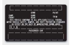
The certification label is located on the driver's door sill at the center pillar and shows the maximum allowable weight of the fully loaded vehicle. This is called the GVWR (Gross Vehicle Weight Rating). The GVWR includes the weight of the vehicle, all occupants, fuel and cargo. This label also tells you the maximum weight that can be supported by the front and rear axles, called Gross Axle Weight Rating (GAWR).
