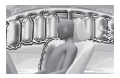
Side and curtain airbags are designed to inflate when an impact is detected by side collision sensors depending on the severity of impact resulting from a side collision.
