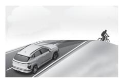
Forward Collision-Avoidance Assist may not detect other vehicles, powered two-wheelers, pedestrians or cyclists in front of you while driving uphill or downhill, adversely affecting the performance of the sensors.
