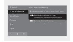
With the vehicle on, press the SETUP button and select or deselect Vehicle > Driver Assistance > Driver Attention Warning and then enable Leading Vehicle Departure alert in the infotainment system to set whether to use each function.
