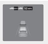
If you want to speed up temporarily without altering the set speed while Smart Cruise Control is operating, depress the accelerator pedal. While the accelerator pedal is depressed, the set speed, distance level and target distance will blink on the instrument cluster.
