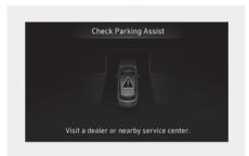
When Remote Smart Parking Assist is not working properly, the "Check Parking Assist" warning message will appear on the infotainment system. If the message appears, stop using Remote Smart Parking Assist, and have your vehicle inspected by an authorized HYUNDAI dealer.
