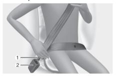
Pull the belt out of the retractor and insert the metal tab (1) into the buckle (2). An audible "click" sounds when the tab locks into the buckle. Make sure the seat belt is not twisted.
