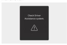
When Driver Attention Warning is not working properly, the "Check Driver Assistance system." warning message will appear on the cluster for several seconds, and the master (A) warning light and the inattentive driving (A) warning light will appear on the instrument cluster. If this occurs, have your vehicle inspected by an authorized HYUNDAI dealer.
