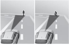
Forward Collision-Avoidance Assist may detect a vehicle, powered two-wheeler, pedestrian or cyclist in the next lane or outside the lane when driving on a curved road.
