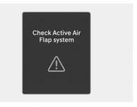
The active air flap system may not operate normally if the air flap is temporarily opened due to foreign factors or if the controller is contaminated by snow or rain, etc.
