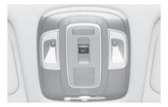
The sunroof can only be operated when the Start/Stop button is in the ON or START position.
