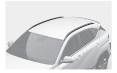
Your vehicle may come equipped with roof side rails. If your vehicle is equipped with roof rack rails, you can add roof rack crossbars as an accessory (not shown).
