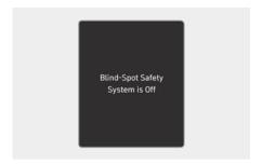
When the vehicle is restarted with Blind-Spot Collision-Avoidance Assist off, the "Blind-Spot Safety System is Off" message will appear on the instrument cluster.
