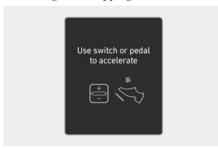
When Highway Driving Assist is operating, your vehicle will stop if the vehicle ahead of you stops. Also, if the vehicle ahead of you starts moving within 30 seconds after the stop, your vehicle will start as well. In addition, after the vehicle has stopped and 30 seconds have passed, the "Use switch or pedal to accelerate" message will appear on the instrument cluster. Depress the accelerator pedal or operate the + switch, - switch or IIO switch to start driving.
