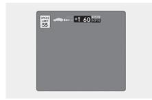
If the speed limit of the road changes during the operation of Manual Speed Limit Assist or Smart Cruise Control, an arrow in the direction of up or down is displayed to inform the driver that the set speed needs to be changed. At this time, the driver can change the set speed according to the speed limit by using the + or - switch on the steering wheel.
