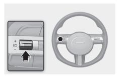
Press the **II 2** switch or depress the brake pedal to temporarily cancel Smart Cruise Control.
