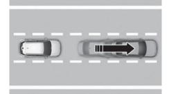
If the vehicle in front abruptly departures, Leading Vehicle Departure Alert may not operate properly.
