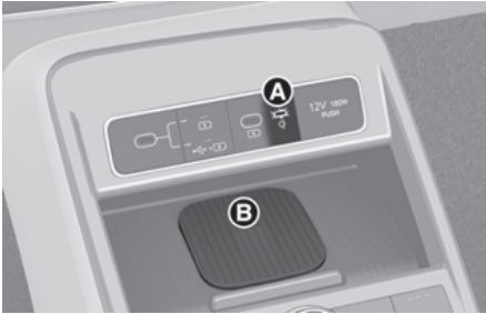
[A] Indicator light [B] Charging pad
