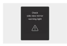
When the side view mirror warning light is not working properly, the "Check side view mirror warning light" warning message will appear on the instrument cluster for several seconds, and the master (A) warning light will illuminate on the instrument cluster. If this occurs, have your vehicle inspected by an authorized HYUNDAI dealer.
