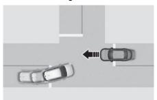
Junction Turning function can help avoid a collision with an oncoming vehicle, a powered-two-wheeler in an adjacent lane when turning left at a crossroad with the turn signal on by applying emergency braking.
