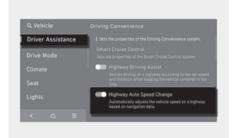
With the vehicle on, press the SETUP button and then select Vehicle > Driver Assistance > Driving Convenience > Highway Auto Speed Change from the infotainment system to turn on Navigation based Smart Cruise Control and deselect to turn off the function.
