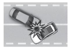
In an angled collision, the force of impact may direct the occupants in a direction where the airbags would not be able to provide any additional benefit, and thus the sensors may not deploy any airbags.
