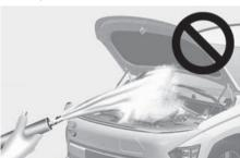
Never allow water or other liquids to come in contact with electrical/electronic components inside the vehicle as water or other liquids may flow in to the motor compartment through the front trunk and damage electrical/electronic components.
