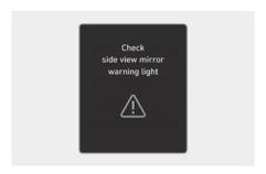
When the side view mirror warning light is not working properly, the "Check side view mirror warning light" warning message appears on the instrument cluster for several seconds, and the master (A) warning light illuminates on the instrument cluster. If this occur, have your vehicle inspected by an authorized HYUNDAI dealer.
