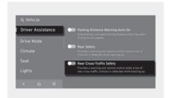
With the vehicle on, press the SETUP button, and then select Vehicle > Driver Assistance > Parking Safety > Rear-Cross Traffic Safety in the infotainment system to turn on Rear Cross-Traffic Collision-Avoidance Assist and deselect to turn off the function.
