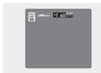
If the speed limit of the road changes during the operation of Manual Speed Limit Assist or Smart Cruise Control, an arrow in the direction of up or down is displayed to inform the driver that the set speed needs to be changed. At this time, the driver can change the set speed according to the speed limit by using the + or - switch on the steering wheel.
