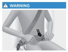
Improperly positioned seat belts may increase the risk of serious injury in an accident or sudden stop. Take the following precautions when adjusting the seat belt:
