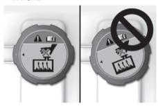
Make sure that the tiny protrusions inside the coolant cap is securely interlocked.
