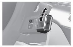
To shift the gear to D (Drive), rotate the rotary shifter to D (Drive) while depressing the brake pedal.
