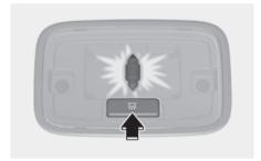
$\overline{\times}$ : Press the button to turn on and off the rear room lamp.
