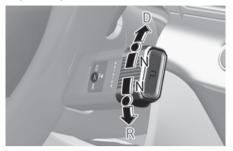
To shift the gear to N (Neutral), rotate the rotary shifter to N (Neutral) while depressing the brake pedal.
