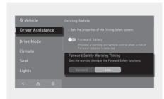
With the vehicle on, press the SETUP button, and then select Vehicle > Driver Assistance > Driving Safety > Forward Safety Warning Timing in the infotainment system to change the initial warning activation time for Forward Collision-Avoidance Assist. The warning time can be set to either "Standard" or "Late"
