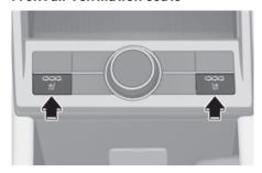
While the vehicle running, press the switch to cool the driver's seat or front passenger's seat.
