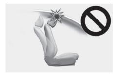
If you adjust the seatback towards the front with the head restraint and seat cushion raised, the head restraint may come in contact with the sunvisor or other parts of the vehicle.
