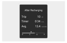
Trip distance, total driving time, average energy consumption, and instant energy consumption after the vehicle has been recharged are displayed. To reset manually, press the **OK** button on the steering wheel for more than 1 second when "After Recharging" appears.
