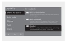
With the vehicle on, press the SETUP button and then the select **Driver**Assistance > Driving Safety > Safe Exit in the infotainment system to turn on Safe Exit Warning and deselect to turn off the function.
