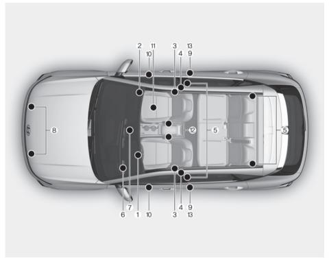
The SRS consists of the following components:
