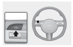
Press the Driving Assist ((?)) button to turn Manual Speed Limit Assist off. The Speed Limit (() LIMIT) indicator will go off.
