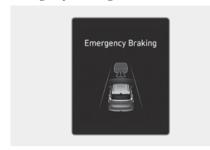
To warn the driver that emergency braking will be assisted, the "Emergency Braking" warning message will appear on the cluster, an audible warning will sound, and the steering wheel will vibrate.
