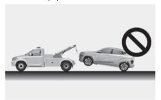
Do not lift using the trailer hitch or body and chassis part.
