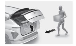
On a vehicle equipped with a smart key, the liftgate can be opened with hands-free activation using the smart liftgate system.
