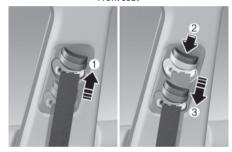
Pull it up (1) to raise the height. To lower it, push it down (3) while pressing the height adjuster button (2). Release the button to lock the anchor in place. Try pushing the height adjuster down to make sure that it is locked in place.
