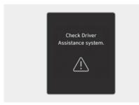
When Forward Collision-Avoidance Assist is not working properly, the **Check Driver Assistance system.** warning message will appear, and the warning lights will illuminate on the instrument cluster. Have your vehicle inspected by an authorized HYUNDAI dealer.
