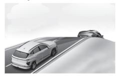
During uphill or downhill driving, the Smart Cruise Control may not detect a moving vehicle in your lane, and cause your vehicle to accelerate to the set speed. Also, vehicle speed will rapidly decrease when the vehicle ahead is detected suddenly.
