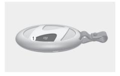
Press and hold the Door Unlock (1) button on the smart key for more than 3 seconds and the windows move down after the doors are unlocked. Window movement stops when you release the door unlock button.
