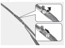
4. Install a new wiper blade assembly in the reverse order of removal
