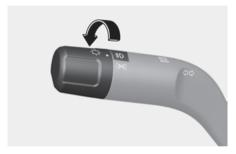
The headlight, parking light, license plate light and instrument panel lamp are turned ON.
