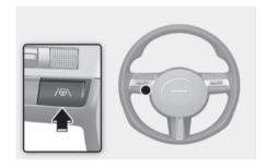
With the vehicle on, tap the Lane Driving Assist button located on the steering wheel to turn on Lane Following Assist. The gray or green  $(\Theta)$  indicator light will illuminate on the instrument cluster.
