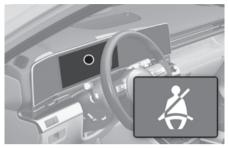
As a reminder to the driver, the driver's seat belt warning light illuminates for about 6 seconds each time the Start/Stop button is in the ON position regardless of seatbelt fastening.
