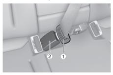
Insert the tongue plate (1) into the buckle (2) until an audible "click" is heard, indicating the latch is locked. Pull the shoulder portion of the belt to snug the belt across your hips and remove slack. Make sure the seat belt is not twisted.
