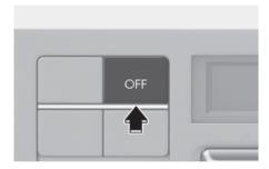
Press the **OFF** button to turn the climate control system off. You can still operate the mode and air intake buttons as long as the Start/Stop button is in the ON position.
