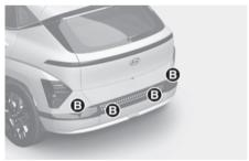
[A] Wide-rear view camera[B] Rear ultrasonic sensors
