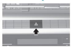
The hazard warning flasher warns other drivers to exercise extreme caution when approaching, overtaking, or passing your vehicle. It should be used whenever making emergency repairs or when stopped near the edge of a roadway.
