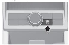
Press the Parking Safety (P<sup>\*\*</sup>) button to turn on Forward/Reverse Parking Distance Warning. Press the button again to turn off the function.
