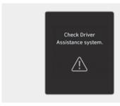
When Highway Driving Assist is not working properly, the "Check Driver Assistance system." warning message and yellow Lane Keeping Assist (A) warning light appears on the instrument cluster. If this occurs, have your vehicle inspected by an authorized HYUNDAI dealer.
