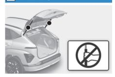
Always close the liftgate before driving. Do not grab or hold on to the liftgate support struts or they may be damaged. Deformation of the liftgate support struts may result in vehicle damage and personal injury.
