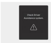
When Safe Exit Warning is not working properly, the "Check Driver Assistance system." warning message will appear on the instrument cluster for several seconds, and the master (A) warning light will appear on the instrument cluster. If this occurs, have your vehicle inspected by an authorized HYUNDAI dealer.
