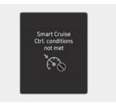
If the Driving Assist button, + switch, - switch or IIO switch is operated when Smart Cruise Control operating conditions are not satisfied, the "Smart Cruise Ctrl. conditions not met" will appear on the instrument cluster, and an audible warning will sound.
