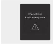
When High Beam Assist is not working properly, the "Check Driver Assistance system." warning message may appear, and the \(\triangle \) warning light may illuminate on the instrument cluster. Have the system inspected by an authorized HYUNDAI dealer.
