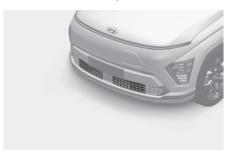
Active air flap system controls the air flap below the front bumper to cool the vehicle parts and improve energy efficiency.
