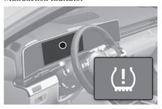
The TPMS Malfunction Indicator (①) illuminates after it blinks for about one minute when there is a problem with the Tire Pressure Monitoring System.
