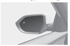
To warn the driver a vehicle is detected, the warning light on the side view mirror illuminates. Vehicle detection operates under following conditions.
