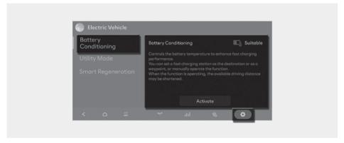
2. On the Home screen, select **Electric Vehicle** > ♥ > **Battery Conditioning** and select **Active** to use manually.
