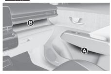
[A] Driver seat door, passenger seat door[B] Passenger seat open tray
