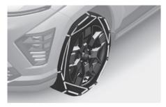
Since the sidewalls of radial tires are thinner than other types of tires, they may be damaged by mounting some types of tire chains on them. Therefore, the use of snow tires is recommended instead of tire chains. If tire chains must be used, use genuine Hyundai parts and install the tire chain after reviewing the instructions provided with the tire chains. Damage to your vehicle caused by improper tire chain use is not covered by your vehicle manufacturer's warranty.
