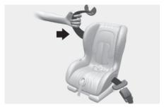
Remove as much slack from the belt as possible by pushing down on the Child Restraint System while feeding the shoulder belt back into the retractor.
