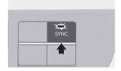
Adjusting the temperature, air flow direction, and fan speed equally
