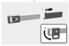
Turn the knob (2) of the mechanical key after removing the key protector (1).
