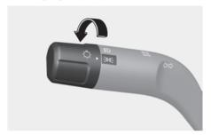
The parking light, license plate light, and instrument panel lamp are turned ON.
