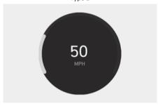
The speedometer indicates the speed of the vehicle and is calibrated in mi. per hour (MPH).
