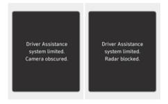
When the front windshield where the front view camera is located, front radar cover, bumper (if equipped) or sensor is covered with foreign material, such as snow or rain, it can reduce the detecting performance and temporarily limit or disable Forward Collision-Avoidance Assist.
