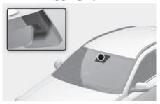
The Auto defogging reduces the likelihood of fogging up the inside of the windshield by sensing moisture on inside of the windshield.
