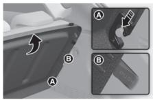
To release the cargo area cover, press the stopper [B], lower the cover, and pull out the cover diagonally.
