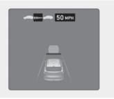
If you want to speed up temporarily without altering the set speed while Smart Cruise Control is operating, depress the accelerator pedal. While the accelerator pedal is depressed, the set speed, distance level and target distance will blink on the instrument cluster.
