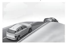
When coasting uphill or downhill, the front sensors may not detect the vehicle ahead or suddenly detect the vehicle ahead at the end of the incline or at the point where the incline changes. The regenerative braking intensity is adjusted automatically changing your vehicle speed. Brake as needed to reduce your driving speed.
