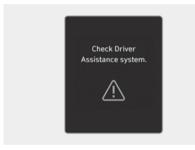
When Blind-Spot Collision Warning is not working properly, the "Check Driver Assistance system." warning message will appear on the instrument cluster for several seconds, and the master (△) warning light will appear on the instrument cluster. If this occurs, have your vehicle inspected by an authorized HYUNDAI dealer.
