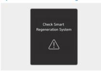
When the front radar is covered or blocked, the smart regeneration system may be temporarily disabled. The "Check Smart Regeneration System" warning message may appear, and the regenerative braking level is displayed on the instrument cluster.
