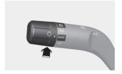
To turn on the high beam headlight, push the lever away from you. The lever returns to its original position.
