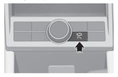
Press the Parking Safety (P<sup>n</sup>) button to turn on Forward/Reverse Parking Distance Warning. Press the button again to turn off the function.
