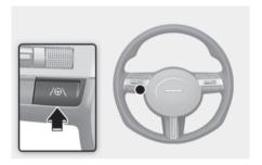
• With the vehicle on, press and hold the Lane Driving Assist button (/⊕\) located on the steering wheel to turn on Lane Keeping Assist. The (/≔\) indicator light illuminates on the instrument cluster. The Lane Driving Assist button also controls the Lane Following Assist when tapped (short press instead of a press and hold).
