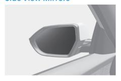
Your vehicle is equipped with both left-hand and right-hand side view mirrors. The mirrors can be adjusted remotely with mirror adjustment control switch. Adjust the side view mirrors to your desired position before driving. The side view mirrors can be folded manually to help prevent damage when going through an automatic car wash or when passing through a narrow street.
