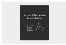
In traffic, your vehicle will stop if the vehicle ahead of you stops. Also, if the vehicle ahead of you starts moving, your vehicle will start as well. In addition, after the vehicle has stopped and a certain time have passed, the "Use switch or pedal to accelerate" message will appear on the instrument cluster. Depress the accelerator pedal or operate the + switch, - switch or IIO switch to start driving.
