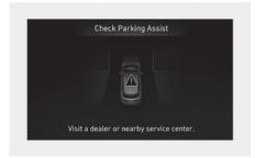
When Remote Smart Parking Assist is not working properly, the "Check Parking Assist" warning message will appear on the infotainment system. If the message appears, stop using Remote Smart Parking Assist, and have your vehicle inspected by an authorized HYUNDAI dealer.
