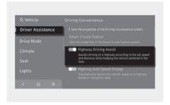
With the vehicle on, press the **SETUP** button and then select or deselect Vehicle > Driver Assistance > Driving Convenience > Highway Driving **Assistance** from the infotainment system to set whether to use each function.
