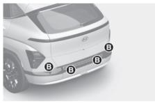
[A] Front ultrasonic sensors[B] Rear ultrasonic sensors
