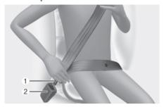
Pull the belt out of the retractor and insert the metal tab (1) into the buckle (2). An audible "click" sounds when the tab locks into the buckle. Make sure the seat belt is not twisted.
