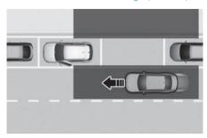
While your vehicle is stopped, and if Safe Exit Warning detects a vehicle approaching the rear corner of your vehicle and a passenger opens a door, Safe Exit Warning may warn you with a warning message and a warning sound to help avoid a collision.
