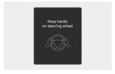
If the driver takes their hands off the steering wheel for several seconds, the "Keep hands on steering wheel" warning message appears on the instrument cluster, and an audible warning sounds in stages.
