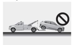
Do not tow vehicles with sling-type equipment. Only use wheel lift or flatbed equipment.
