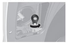
6. Install a new bulb and reinstall in the reverse order.
