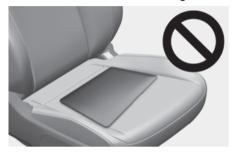
If large quantity of liquid has been spilled on the passenger seat, the airbag warning light may illuminate or malfunction. Therefore, make sure the seat has been completely dried before driving the vehicle.
