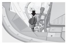
Check the fluid level in the washer fluid reservoir and add fluid if necessary. Plain water may be used if washer fluid is not available. However, use washer solvent with antifreeze characteristics in cold climates to prevent freezing.
