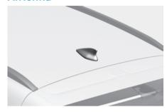
The shark fin antenna receives transmitted data (for example, AM/FM, SXM).
