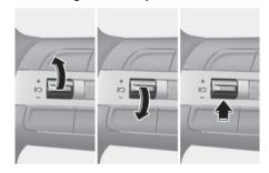
To resume Manual Speed Limit Assist after the function was paused, operate the +,-,119 switch.
