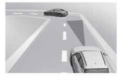
The front sensors may not detect the vehicle ahead if you are coasting on a curve. The regenerative braking intensity may automatically decrease and accelerate the vehicle.
