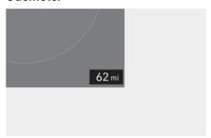
The odometer indicates the total distance that the vehicle has been driven and should be used to determine when periodic maintenance is required.
