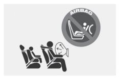
Even though your vehicle is equipped with the OCS, never install a child restraint in the front passenger's seat. An inflating airbag can forcefully strike a child or child restraint resulting in serious or fatal injury.
