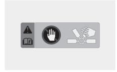
When using the V2L, the cooling fan in the vehicle motor compartment can operate automatically even if the vehicle is turned off. Do not put your hand near the cooling fan when the V2L is operating.
