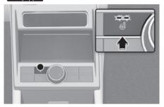
When the Start/Stop button is in the ON position or when the vehicle is in the ready mode (READY indicator ON), press the steering wheel heater button to warm the steering wheel. The indicator on the button illuminates.
