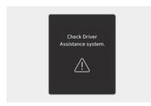
When Driver Attention Warning is not working properly, the "Check Driver Assistance system." warning message will appear on the cluster for several seconds, and the master (A) warning light and the driver's attention (b) warning light will appear on the instrument cluster. If this occurs, have your vehicle inspected by an authorized HYUNDAI dealer.
