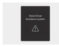
When Smart Cruise Control is not working properly, the "Check Driver Assistance system." warning message will appear, and the "A" warning light will illuminate on the instrument cluster. Have your vehicle inspected by an authorized HYUNDAI dealer.
