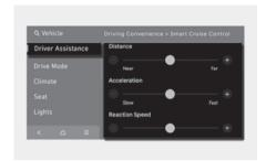
With the vehicle on, press the SETUP button and then select Vehicle > Driver Assistance > Driving Convenience > Smart Cruise Control is selected from the infotainment system, you can change the vehicle distance, the acceleration, and the reaction speed manually.
