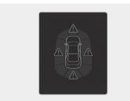
When the Parking Distance Warning is operating, if the function is not working normally or the ultrasonic sensor is blocked, the master warning light (△) appears in the direction of the corresponding sensor. You can check the warning in the Utility view on the cluster.
