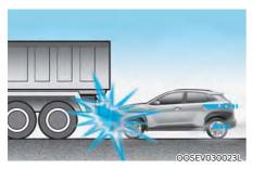
Just before impact, drivers often brake heavily. Such heavy braking lowers the front portion of the vehicle causing it to "ride" under a vehicle with a higher ground clearance. Air bags may not inflate in this "under-ride" situation because deceleration forces that are detected by sensors may be significantly reduced by such "underride" collisions.
