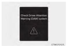
When Driver Attention Warning is not working properly, the 'Check Driver Attention Warning (DAW) system' warning message will appear on the cluster for several seconds, and the master (A) warning light will illuminate on the cluster. If this occurs, have the vehicle inspected by an authorized HYUNDAI dealer.
