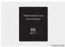
When Smart Cruise Control is not working properly, the 'Check Smart Cruise Control system' warning message will appear, and the \( \underset \) warning light will illuminate on the cluster. Have the vehicle inspected by an authorized HYUNDAI dealer.
