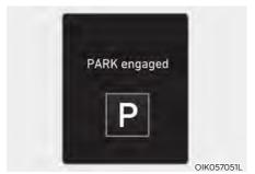
The message appears on the LCD display when the P (Park) position is engaged.
