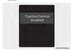
Press the ESC OFF button briefly. The ESC OFF indicator light and message "Traction Control disabled" will illuminate. In this state, the traction control function of ESC is disabled, but the brake control function of ESC (braking management) still operates.
