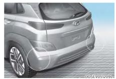
Refer to the picture above for the detailed location of the detecting sensors.
