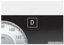
The indicator in the instrument cluster displays the gear position when the START/STOP button is in the ON position.
