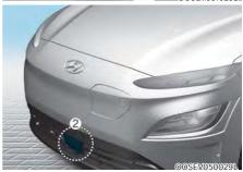
[1]: Front view camera, [2]: Front radar Refer to the picture above for the detailed location of the detecting sensors.
