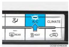
A/C button will turn on (indicator light will illuminate) when the climate control system is controlled automatically (AUTO turned on) and the temperature is set to cool.
