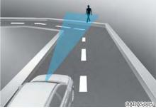
Forward Collision-Avoidance Assist may detect a vehicle, pedestrian in the next lane or outside the lane when driving on a curved road.
