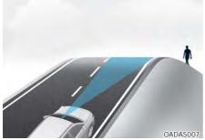
Forward Collision-Avoidance Assist may not detect other vehicles or pedestrians in front of you while driving uphill or downhill, adversely affecting the performance of the sensors.
