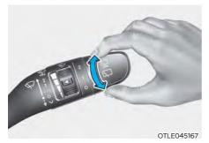
The rear window wiper and washer switch is located at the end of the wiper and washer switch lever.
