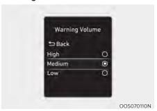
Select 'Driver Assistance → Warning Volume' from the cluster or infotainment system Settings menu to change the Warning Volume to 'High', 'Medium', or 'Low' for Forward/Reverse Parking Distance Warning.
