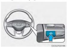
With the vehicle on, press and hold the Lane Driving Assist button located on the steering wheel to turn on Lane Keeping Assist. The white /=\text{indicator light will illuminate on the cluster.
