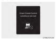
If the Driving Assist button, + switch, - switch or || 5 switch is pushed when Smart Cruise Control operating conditions are not satisfied, the 'Smart Cruise Control conditions not met' will appear on the cluster, and an audible warning will sound.
