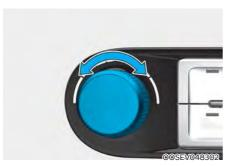
Turn the temperature control knob to the desired temperature. If the temperature is set to the lowest setting (17 °C), the air conditioning system will operate continuously. After the interior has cooled sufficiently, adjust the knob to a higher temperature set point whenever possible.
