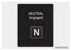
The message appears on the LCD display when the N (Neutral) position is engaged.
