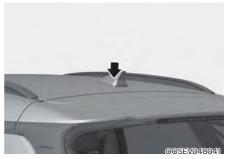
The roof antenna receives data transmitted from base stations and satellites (for example, AM/FM, DAB, GPS).
