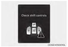
The message appears on the LCD display when there is problem with the shift buttons.
