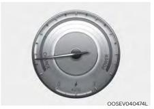
The Power/Charge gauge shows the energy consumption rate of the vehicle and the charge/discharge status of the regenerative brakes.
