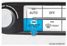
If you press the DRIVER ONLY button (\$\mathbb{G}^{DRIVER}\$) and the indicator light illuminates, cold air mostly blows in the direction of the driver's seat. However, some of the cold air may come out of other seating position ducts to keep indoor air pleasant.
