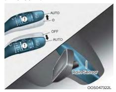
The rain sensor located on the upper end of the windshield glass senses the amount of rainfall and controls the wiping cycle for the proper interval. The wiper operation time will be automatically controlled depends on rainfall.
