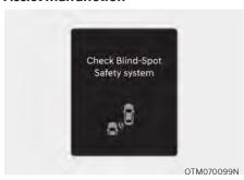
When Blind-Spot Collision-Avoidance Assist is not working properly, the 'Check Blind-Spot Safety system' warning message will appear on the cluster, and the master (1) warning light will illuminate on the cluster. If this occurs, have the vehicle be inspected by an authorized HYUNDAI dealer.
