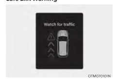
Collision warning when exiting vehicle
