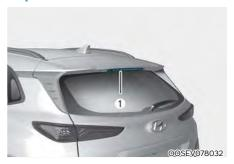
If the high mounted stop lamp (LED) does not operate, contact an authorized HYUNDAI dealer.
