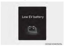
When the high voltage battery level reaches below approximately 8%, this warning message is displayed.
