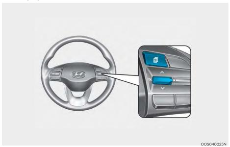
The LCD display modes can be changed by using the control buttons.
