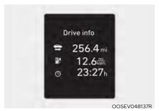
This display shows the trip distance (1), the average energy consumption (2), and the total driving time (3).
