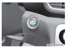
Whenever the front door is opened, the START/STOP button will illuminate and will go off 30 seconds after the door is closed.
