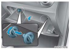
1. With the glove box open, remove the stoppers on both sides.
