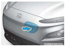
Unlock the vehicle before opening the charging door. Push on the charging door in the area indicated by the arrow to open the door.
