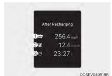
Trip distance (1), average energy consumption (2), and total driving time (3) after the vehicle has been rrecharged are displayed.
