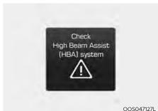
When High Beam Assist is not working properly, the warning message will come on for a few seconds. After the message disappears, the master warning light (1) will illuminate.
