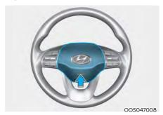
To sound the horn, press the area indicated by the horn symbol on your steering wheel. The horn will operate only when this area is pressed.
