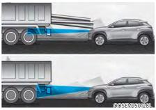
If the vehicle in front of you has cargo that extends rearward from the cab, or when the vehicle in front of you has higher ground clearance, additional special attention is required. Forward Collision-Avoidance Assist may not be able to detect the cargo extending from the vehicle. In these instances, you must maintain a safe braking distance from the rearmost object, and if necessary, steer your vehicle and depress the brake pedal to reduce your driving speed in order to maintain distance.
