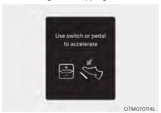
When Highway Driving Assist is operating, your vehicle will stop if the vehicle ahead of you stops. Also, if the vehicle ahead of you starts moving within 30 seconds after the stop, your vehicle will start as well. In addition, after the vehicle has stopped and 30 seconds have passed, the 'Use switch or pedal to accelerate' message will appear on the cluster. Depress the accelerator pedal or operate the + switch, - switch or II 3 switch to start driving.
