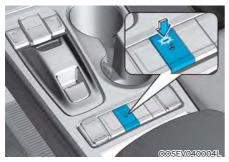
When the vehicle is ON, press the heated steering wheel button to warm the steering wheel.
