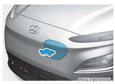
Unlock the vehicle before opening the charging door. From the outside the vehicle, push on the charging door in the area indicated by the arrow to open the door.
