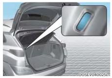
The luggage compartment lamp comes on when the liftgate is opened.
