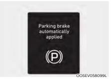
Parking brake automatically applied If EPB is applied while Auto Hold is activated, a warning will sound and a message will appear.
