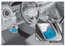
To release EPB (Electronic Parking Brake):
