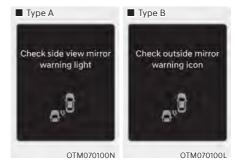
When the outside rearview mirror warning light is not working properly, the 'Check side view mirror warning light' warning message will appear on the cluster for several seconds, and the master (A) warning light will illuminate on the cluster. If this occurs, have the vehicle be inspected by an authorized HYUNDAI dealer.
