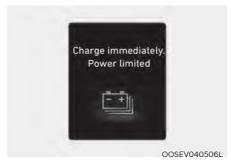
When the high voltage battery level reaches below approximately 5%, this warning message is displayed.
