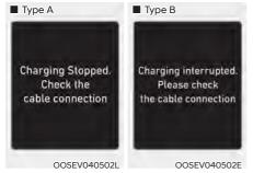
This warning message is displayed when charging is stopped because the charging connector is not correctly connected to the vehicle charging port.
