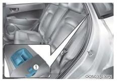
2. Make sure to insert the belt into the guide (1) and check that the seat belt is not twisted.
