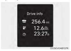
The trip computer mode displays information related to vehicle driving parameters including Energy consumption, tripmeter information and vehicle speed.
