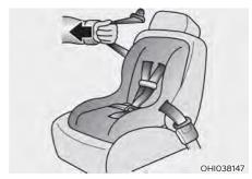
4. Pull the shoulder portion of the seat belt all the way out. When the shoulder portion of the seat belt is fully extended, it will shift the retractor to the "Automatic Locking" (child restraint) mode.
