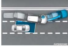
When changing lanes by detecting the lane ahead, if Blind-Spot Collision-Avoidance Assist judges that there is a collision risk with an approaching vehicle in the blind spot, it can help avoid collision by assisting with steering.
