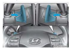
The paddle shifter is used to adjust the regenerative braking level from 0 to 3 during decelerating or braking.
