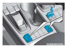
While the vehicle is running, push either of the switches to warm the driver's seat or front passenger's seat.
