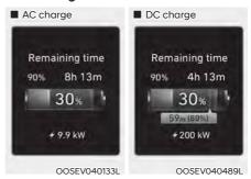
This message is displayed to notify the remaining time to charge the battery to the selected target battery charge level.
