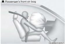
After complete inflation, the air bag immediately starts deflating, enabling the driver to maintain forward visibility and the ability to steer or operate other controls.
