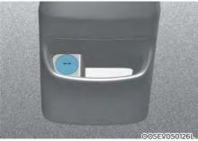
To use the USB and iPod®, open the front console cover by slightly pressing the lower part of the cover (1).
