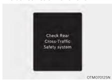
When Rear Cross-Traffic Collision-Avoidance Assist is not working properly, the 'Check Rear Cross-Traffic Safety system' warning message will appear on the cluster for several seconds, and the master (八) warning light will illuminate on the cluster. If the master warning light illuminates, have the vehicle inspected by an authorized HYUNDAI dealer.
