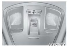
The sunroof can be operated for approximately 30 seconds after the Start/Stop button is in the ACC or OFF position.
