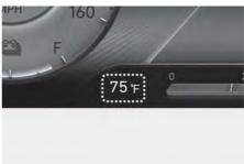
This gauge indicates the current outside air temperatures either in Celsius (°C) or Fahrenheit.
