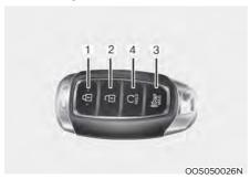
Your HYUNDAI uses a Smart Key, which you can use to lock or unlock doors (and liftgate) and start the vehicle.
