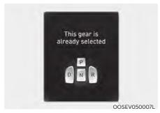
The message appears on the LCD display when the selected gear button is pressed again.
