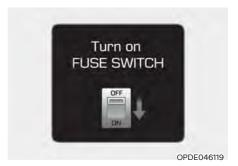
This warning message is displayed if the fuse switch located on the fuse box under the steering wheel is OFF.
