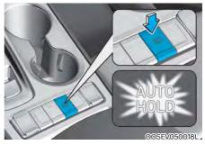
1. With the driver's door and liftgate closed, depress the brake pedal and then press the [AUTO HOLD] switch. The white AUTO HOLD indicator will come on and the system will be in the standby position.
