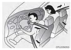
Your vehicle is equipped with driver's and front passenger's Pre-tensioner Seat Belts (Retractor Pretensioner and Emergency Fastening Device System). The purpose of the pre-tensioner is to make sure the seat belts fit tightly against the occupant's body in certain frontal or side collision(s). The Emergency Fastening Device System may be activated in certain crashes where the frontal or side collision(s) is severe enough, together with the air bags.
