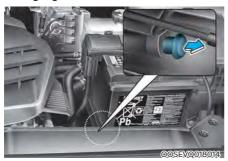
If for some reason the charging connector fails to disconnect normally, the connector may be released manually using the Charging Connector Manual Release. Open the hood and slightly pull the manual release shown in the figure. The charging connector can then be disconnected.
