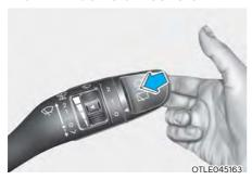
In the OFF (O) position, pull the lever gently toward you to spray washer fluid on the windshield and to run the wipers 1-3 cycles.
