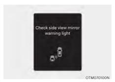
When the outside rearview mirror warning light is not working properly, the 'Check side view mirror warning light' warning message will appear on the cluster for several seconds, and the master (A) warning light will illuminate on the cluster. If the master warning light illuminates, have the vehicle inspected by an authorized HYUNDAI dealer.
