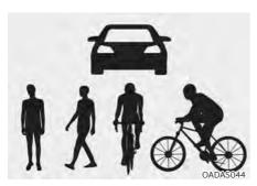
The illustration above shows the image the front view camera and front radar is capable of detecting as a vehicle, pedestrian and cyclist.
