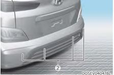
[1]: Front ultrasonic sensors, [2]: Rear ultrasonic sensors
