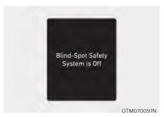
When the vehicle is restarted with Blind-Spot Collision-Avoidance Assist off, the 'Blind-Spot Safety System is Off' message will appear on the cluster.
