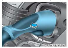
1. Hold the charging connector handle and pull it while pressing the release button (1).
