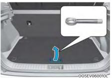
Open the liftgate, and remove the towing hook from the tool case. The tool case is placed under the luggage tray.
