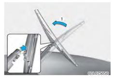
1. Raise the wiper arm and pull out the wiper blade assembly.
