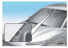
Auto defogging reduces the possibility of fogging up the inside of the windshield by automatically sensing the moisture on inside the windshield.
