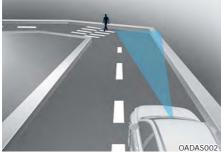
Forward Collision-Avoidance Assist may not detect other vehicles, pedestrians in front of you on curved roads adversely affecting the performance of the sensors. This may result in no warning, braking assist or steering assist (if equipped) when driving.
