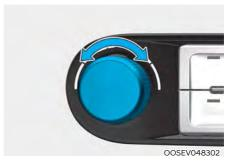
The temperature will increase by turning the knob to the right. The temperature will decrease by turning the knob to the left.
