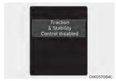
Press and hold the ESC OFF button continuously for more than 3 seconds. The ESC OFF indicator light and message "Traction & Stability Control disabled" illuminates and a warning chime sounds. In this state, both the traction control function of ESC and the brake control function of ESC are disabled.
