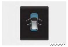
This warning is displayed indicating which door, or hood, or liftgate is open.
