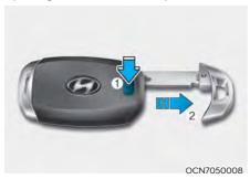
Move the release lever in the direction of the arrow (1) and then remove the mechanical key (2). Insert the mechanical key into the key hole on the door.
