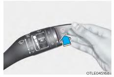
Push the lever away from you to spray rear washer fluid and to run the rear wiper 1~3 cycles. The spray and wiper operation will continue until you release the lever.
