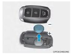
If the Smart Key is not working properly, try replacing the battery with a new one. Battery Type: CR2032
