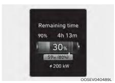
8. After charging has started, the estimated charging time is displayed on the instrument cluster for about 1 minute.
