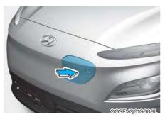
Unlock the vehicle before opening the charging door. From the outside the vehicle, push on the charging door in the area indicated by the arrow to open the door.
