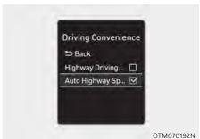
With the vehicle on, select 'Driver Assistance → Driving Assist → Auto Highway Speed Control' from the Settings menu to turn on Navigationbased Smart Cruise Control and deselect to turn off the function.
