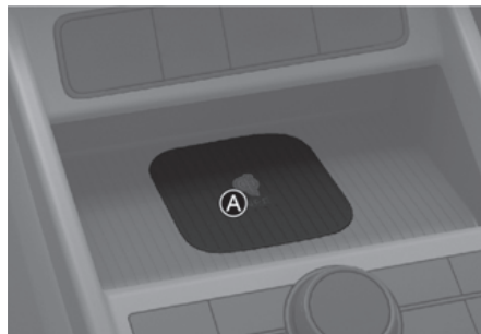
[A] Vehicle authentication pad (Wireless charging pad)
