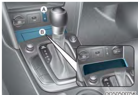
[A] : Indicator light, [B] : Charging pad
