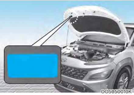
The refrigerant label provides information such as refrigerant type and amount. (R-1234yf)
