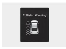
When an approaching vehicle from the rear is detected while a door is being opened, the warning light on the side view mirror may blink, a warning message may appear on the instrument cluster, and an audible warning may sound.
