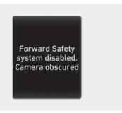
When the front view camera is covered or blocked, Forward Collision-Avoidance Assist may be temporarily limited or disabled.
