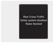
If the rear corner radar is blocked or covered, or when the rear bumper around the rear corner radar or sensor is covered by any foreign material, such as snow, rain, or dirt, or when a trailer or hitch mounted carrier is installed, the detecting performance may reduce and temporarily limit or disable Rear Cross-Traffic Collision-Avoidance Assist.
