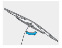
4. While pushing the clip (1), pull down the wiper blade (2).
