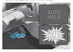
2. When you stop the vehicle completely by depressing the brake pedal, Auto Hold maintains the brake pressure to hold the vehicle stationary. The indicator changes from white to green. The vehicle remains stationary even if you release the brake pedal.
