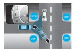
If a STOP, YIELD or Roundabout sign is detected and the ISG system is deactivated by ISG inhibition at traffic signs, a message will appear on the cluster display (if equipped) when the "AUTO STOP" page on the instrument cluster is selected.
