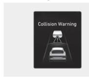
If Forward Collision-Avoidance Assist judges that a collision may occur, the message may appear on the instrument cluster and an audible warning is heard and the steering wheel may vibrate when:
