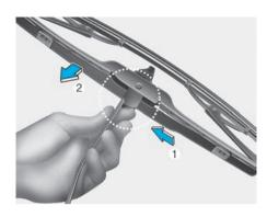
Remove the wiper blade from the wiper arm.
