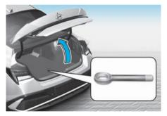
Remove the hole cover by pressing the lower part of the cover on the bumper.
