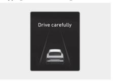
After your vehicle has stopped following an Emergency Braking event, the "**Drive carefully**" warning message may appear on the instrument cluster.
