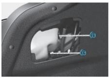
5. Remove the rear combination light assembly from the body of the vehicle.
