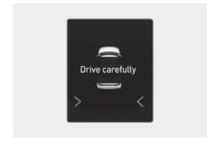
After your vehicle is stopped following an Emergency Braking event, the "Drive carefully" warning message may appear on the instrument cluster.
