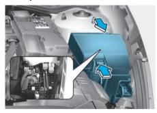
Inside the fuse panel cover, you can find the panel label describing fuse names and ratings.
