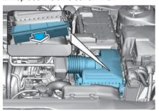
3. Insert the air cleaner cover in the hinge (2) and engage the clip (1) after closing the cover.
