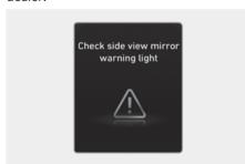
When the side view mirror warning light is not working properly, the "Check side view mirror warning light" warning message will appear on the instrument cluster for several seconds, and the master (小) warning light will illuminate on the instrument cluster. Have the vehicle inspected by an authorized HYUNDAI dealer.
