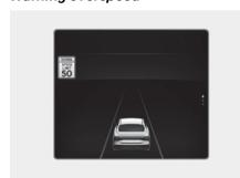
When driving at a speed higher than the displayed speed limit, the speed limit appears in red.
