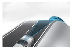
During uphill or downhill driving, Smart Cruise Control may not detect a moving vehicle in your lane, and cause your vehicle to accelerate to the set speed. Also, your vehicle speed rapidly decreases when a vehicle ahead is detected suddenly.
