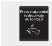
If you did not apply the brake pedal when you release Auto Hold by pressing the AUTO HOLD switch, a warning sounds and a message appears.
