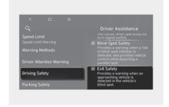
With the ignition switch ON, go to User settings > Driver Assistance > Driving Safety > Exit Safety from the settings menu in the instrument cluster or Settings > Vehicle > Driver Assistance > Driving Safety > Exit Safety from the Settings menu in the infotainment system to turn this function on and off.
