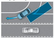
Blind-Spot Collision-Avoidance Assist may not detect a vehicle in an adjacent lane when the road merges or divides and may not activate a warning or brake your vehicle.
