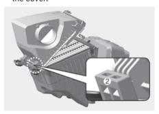
4. Check that the cover is firmly installed.
