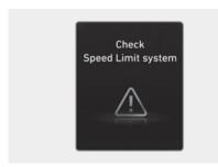
When Intelligent Speed Limit Assist is not working properly, the "Check Speed Limit Assist System" warning message may appear, and the (A) warning light may illuminate on the instrument cluster. Have the vehicle inspected by an authorized HYUNDAI dealer.
