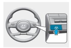
With the ignition switch ON, press the Lane Driving Assist button on the steering wheel to turn on Lane Following Assist. The white or green indicator light illuminates on the instrument cluster. Press the button again to turn off the function.
