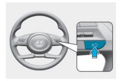
Press the **II** Dutton to temporarily cancel the set speed limit. The set speed turns off, but the Manual Speed Limit Assist ( TIMIT ) indicator light stays on.
