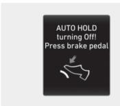
When the conversion from Auto Hold to EPB is not working properly, a warning sounds and a message appears.
