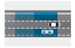
Blind-Spot Collision-Avoidance Assist helps detect and warns you that a vehicle is in the blind spot area.
