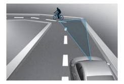
Forward Collision-Avoidance Assist may not detect other vehicles, powered two-wheeler, pedestrians or cyclists in front of you when driving on a curve and may not activate a warning or brake your vehicle when needed.
