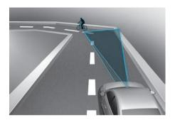
Forward Collision-Avoidance Assist may not detect other vehicles, powered two-wheelers, pedestrians or cyclists in front of you when driving on a curved roads adversely affecting the performance of the sensors. This may result in no warning, braking assist when necessary.
