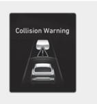
While Smart Cruise Control is operating and the collision risk of the vehicle ahead is high, the "Collision Warning" warning message may appear on the instrument cluster, and an audible alert sounds and the steering wheel may vibrate.
