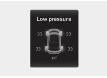
TPMS is not a substitute for manually checking the tire pressure with a tire gauge. Changes in temperature affect tire pressure. Refer to "Check tire pressure" in the Maintenance chapter for proper tire inflation and tire pressure measurement procedure.
