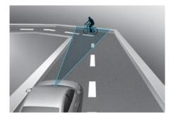
If a vehicle, powered two-wheeler, pedestrian or cyclist is detected in the next lane or outside the lane when driving on a curved road, Forward Collision-Avoidance Assist may warn you and may brake your vehicle even when not needed.
