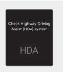
When Highway Driving Assist is not working properly, the "Check Highway Driving Assist (HDA) system" warning message may appear, and the \(\begin{align\*}\) warning light may illuminate on the instrument cluster. Have the vehicle inspected by an authorized HYUNDAI dealer.
