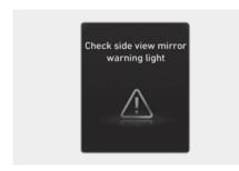
When the side view mirror warning light is not working properly, the "Check side view mirror warning light" warning message may appear, and the \( \text{\Lambda} \) warning light may illuminate on the instrument cluster. Have the vehicle inspected by an authorized HYUNDAI dealer.
