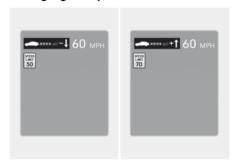
If the speed limit changes when using Manual Speed Limit Assist or Smart Cruise Control, an arrow in the direction of up or down appears to inform you to change the set speed by pushing the + or - switch.
