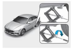
9. Loosen the wheel nuts with the wheel lug wrench and remove them with your fingers. Remove the wheel from the studs and lay it flat on the ground out of the way. Remove any dirt or debris from the studs, mounting surfaces, and spare tire.
