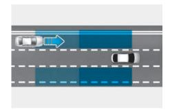
Blind-Spot Collision-Avoidance Assist helps detect and warns you that a vehicle is approaching at high speed from the blind spot area.
