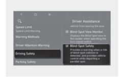
With the ignition switch ON, go to User settings > Driver Assistance > Driving Safety > Blind-Spot Safety from the settings menu in the instrument cluster or Settings > Vehicle > Driver Assistance > Driving Safety > Blind-Spot Safety from the settings menu in the infotainment system to select the following:
