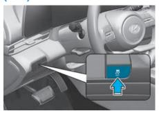
Electronic Stability Control helps stabilize the vehicle during cornering maneuvers.
