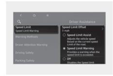
With the ignition switch ON, select or deselect **User Settings** > **Driver Assistance** > **Speed Limit** from the User Settings menu in the instrument cluster or **Settings** > **Vehicle** > **Driver Assistance** > **Speed Limit** from the Settings menu in the infotainment system to set whether to use each function.
