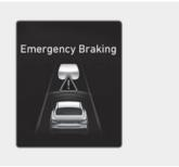
If Forward Collision-Avoidance Assist judges avoiding a collision may be difficult, it applies higher brake force that may help avoid a collision with the vehicle, pedestrian or cyclist detected ahead.
