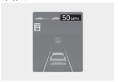
Manual Speed Limit Assist or Smart Cruise Control assists the vehicle to adjust its speed according to the speed limit. When the cruising speed is set as same as the speed limit, the vehicle automatically adjusts its speed if the speed limit changes. The function operates on the road which has a speed limit of 44 mph (70 km/h) or higher. When the function is active, the cruising speed on the instrument cluster appears in green.
