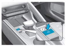
Press the Parking/View button (1) while the gear is in P (Park) to turn on Rear View Monitor.
