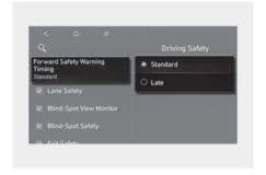
With the ignition switch ON, go to User Settings > Driver Assistance > Driving Safety > Forward Safety Warning Timingfrom the settings menu in the instrument cluster or Settings > Vehicle > Driver Assistance > Driving Safety > Forward Safety Warning Timing settings menu in the infotainment system to change the initial warning activation time. Warning Timing is set to Standard at the factory.
