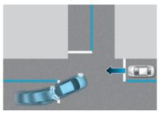
Junction Turning function can help avoid a collision with an oncoming vehicle in an adjacent lane when turning left at a crossroad with the turn signal on by applying emergency braking.
