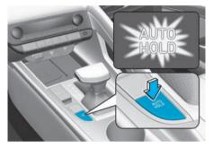
1. Press the AUTO HOLD switch. The white AUTO HOLD indicator comes on and the system is in standby.
