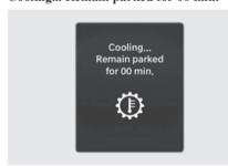
If you move the vehicle to a safe location and shift the gear to P (Park) with the engine running, the above warning message appears.
