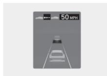
If you depress the accelerator pedal above a certain speed while Smart Cruise Control is operating, your vehicle can speed up temporarily without changing the set speed. The set speed, distance level, and target distance blink on the instrument cluster while depressing the accelerator pedal. Your vehicle speed may decrease if the accelerator pedal is not depressed far enough.
