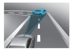
On a curved road, Smart Cruise Control may not detect a vehicle in the same lane, and may accelerate to the set speed. Your vehicle speed may be reduced if a vehicle is detected in an adjacent lane and your vehicle speed may rapidly decrease when a vehicle ahead is detected suddenly.
