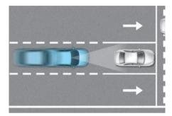
Forward Collision-Avoidance Assist uses the front view camera to help detect a vehicle, a pedestrian ahead on the road. The function may warn you with a warning message on the instrument cluster and an audible warning if a collision is imminent. If necessary, it may assist with braking your vehicle to help reduce collision speed and avoid a collision.
