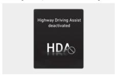
If the driver still does not have their hands on the steering wheel after the hands-off warning, the "**Highway Driving Assist deactivated**" warning message may appear and Highway Driving Assist is automatically canceled.
