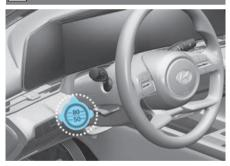
Detach the speed restriction label from the sealant bottle, and place it in a highly visible place inside the vehicle such as on the steering wheel to remind the driver not to drive too fast.
