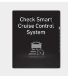
When Smart Cruise Control is not working properly, the "Check Smart Cruise Control system" warning message may appear, and the A warning light may illuminate on the instrument cluster. Have the vehicle inspected by an authorized HYLINDAL dealer.
