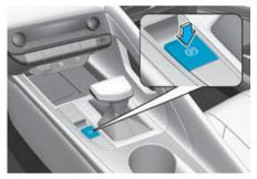
To release EPB (Electronic Parking Brake):
