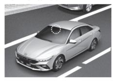
The front view camera is mounted near the top of the windshield inside your vehicle.
