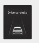
After your vehicle has stopped following an Emergency Braking event, the "Drive carefully" warning message may appear on the instrument cluster.
