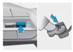
Press the **II** button or depress the brake pedal to temporarily cancel Smart Cruise Control.
