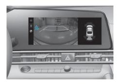
To warn you of an approaching vehicle from the rear left or right of your vehicle, the warning light on the side view mirror may blink, a warning message may appear on the instrument cluster, and an audible warning may sound and the steering wheel may vibrate.
