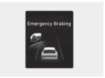
If Forward Collision-Avoidance Assist judges avoiding a collision may be difficult, it applies higher brake force that may help avoid a collision with the oncoming vehicle detected.
