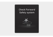
When Forward Collision-Avoidance Assist is not working properly, the "Check Forward Safety system" warning message may appear, and the A and warning lights may illuminate on the instrument cluster. Have the vehicle inspected by an authorized HYUNDAI dealer.
