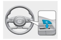
2. Push the + switch up or - switch down to change the set speed.
