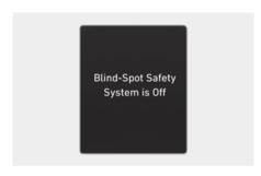
When the engine is restarted with Blind-Spot Collision-Avoidance Assist off, the "Blind-Spot Safety System is Off" message will appear on the instrument cluster. If you select Blind-Spot Safety, warning light on the side view mirror will blink for three seconds. In addition, if the vehicle is turned on, when Blind-Spot Safety is selected, the warning light on the side view mirror will blink for three seconds.
