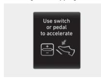
When Highway Driving Assist is operating, your vehicle stops if the vehicle ahead of you stops. Also, if the vehicle ahead of you starts moving within 30 seconds after the stop, your vehicle starts as well. If your vehicle has stopped and 30 seconds have passed, the "Use switch or pedal to accelerate" message appears on the instrument cluster. Depress the accelerator pedal or operate the +/- switch IID button to accelerate.
