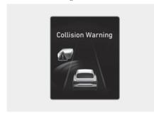
If Forward Collision-Avoidance Assist judges that a collision may occur, the message may appear on the instrument cluster and an audible warning is heard and the steering wheel may vibrate when:
