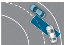
Blind-Spot Collision-Avoidance Assist may detect a vehicle in the same lane when driving on a curved road and activate a warning or brake your vehicle.
