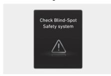
When Safe Exit Warning is not working properly, the "Check Blind-Spot Safety system" warning message will appear on the instrument cluster for several second, and the master (小) warning light will appear on the instrument cluster. Have the vehicle inspected by an authorized HYUNDAI dealer.
