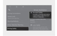
With the ignition switch ON, go to User Settings > Driver Assistance > Driving Safety from the settings menu in the instrument cluster or Settings > Vehicle > Driver Assistance > Driving Safety from the settings menu in the infotainment system to select the following:
