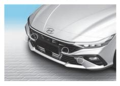
These ultrasonic sensors are mounted to the front bumper outside your vehicle.
