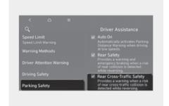
With the ignition switch ON, go to User settings > Driver Assistance > Parking Safety > Rear Cross-Traffic Safety from the settings menu in the instrument cluster or Settings > Vehicle > Parking Safety > Rear Cross-Traffic Safety from the settings menu in the infotainment system to turn on Rear Cross-Traffic Collision-Avoidance Assist and deselect to turn Rear Cross-Traffic Collision-Avoidance Assist on and off.
