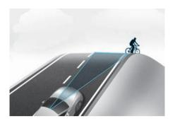
Forward Collision-Avoidance Assist may not detect other vehicles, powered two-wheeler, pedestrians or cyclists in front of you while driving uphill or downhill.
