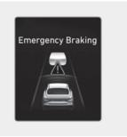
If Forward Collision-Avoidance Assist judges avoiding a collision may be difficult, it applies higher brake force that may help avoid a collision with the vehicle, pedestrian, or cyclist detected ahead.
