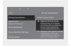
With the ignition switch ON, go to User Settings > Driver Assistance > Driving Convenience from the settings menu in the instrument cluster or Settings > Vehicle > Driver Assistance > Driving Convenience from the settings menu in the infotainment system to set whether to use each function.
