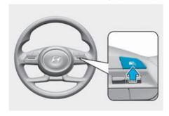
2. Press the Driving Assist (\*) button at the desired speed. The set speed and Cruise (\*CRUISE) indicator light illuminates on the instrument cluster.
