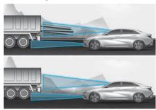
Forward Collision-Avoidance Assist may not be able to detect all potential hazards, like if the vehicle in front of you has cargo that extends rearward past the end of the vehicle or if the vehicle in front of you has higher ground clearance. Always maintain a safe distance from the vehicles ahead. Adjust your vehicle speed or steer your vehicle depending on the road conditions.
