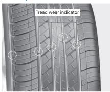
If the tire is worn evenly, a tread wear indicator appears as a solid band across the tread. This shows there is less than 1/16 in. (1.6 mm) of tread left on the tire. Replace the tire when this happens.
