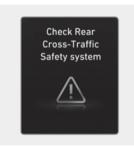
When the Rear Cross-Traffic Collision-Avoidance Assist is not working properly, the "Check Rear Cross-Traffic Safety system" warning message may appear, and the \(\hat{\Lambda}\) warning light may illuminate on the instrument cluster. Have the vehicle inspected by an authorized HYLINDAL dealer.
