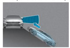
Rear Cross-Traffic Collision-Avoidance Assist may be limited when your vehicle is on a uphill or downhill slope, and may not detect any vehicle approaching from the left or right. If this occurs, the function may activate a warning and brake your vehicle even when not needed.
