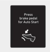
If you shift the gear from N to D (Manual mode) or R without depressing the brake pedal after stopping engine automatically, the engine does not restart automatically and a warning chime alarms. When this happens, press the brake pedal for auto start.
