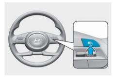
Press the Driving Assist (%) button to turn off Cruise Control. The Cruise (%) CRUISE) indicator light goes off.
