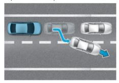
When a vehicle in front of you merges out of the lane, Smart Cruise Control may not immediately detect a new vehicle that is now in front of your vehicle.
