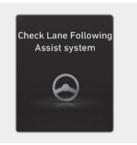
When Lane Following Assist is not working properly, the "Check Lane Following Assist system" message may appear, and the \(\tilde{\Lambda}\) warning light may illuminate on the instrument cluster. Have the vehicle inspected by an authorized HYUNDAI dealer.
