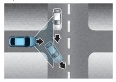
When a vehicle ahead turns at an intersection and is no longer detected, your vehicle may accelerate.
