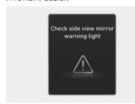
When the side view mirror warning light is not working properly, the "Check side view mirror warning light" warning message will appear on the instrument cluster for several seconds, and the master (小) warning light will illuminate on the instrument cluster. Have the vehicle inspected by an authorized HYUNDAI dealer.
