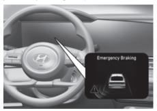
To warn you of a potential collision, the warning light on the side view mirror may blink, a warning message may appear on the instrument cluster, and an audible warning may sound and the steering wheel may vibrate.
