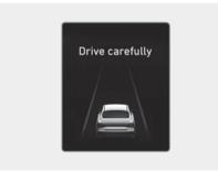
After your vehicle has stopped following an Emergency Braking event, the "Drive carefully" warning message may appear on the instrument cluster.
