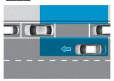
Safe Exit Warning uses the rear corner radars to help detect a vehicle approaching the rear of your vehicle, after the vehicle is stopped and a passenger opens a door.
