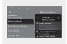
The Warning Methods can be set with the vehicle on. Select **User Settings > Driver Assistance > Warning Methods** from the settings menu in the instrument cluster or Press **Settings** and select **Vehicle > Driver Assistance > Warning Methods** from the infotainment system to change the following settings:
