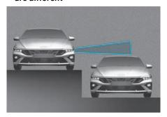
Blind-Spot Collision-Avoidance Assist may not operate properly when driving where the heights of the lanes are different. The function may not detect a vehicle on a road with a different lane height (underpass joining section, grade separated intersections, etc.) and not activate a warning or brake your vehicle.
