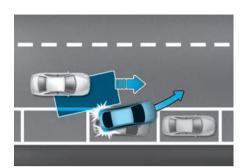
Blind-Spot Collision-Avoidance Assist may brake your vehicle if there is a detected collision risk when driving forward out of a parking space.
