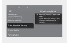
If Leading Vehicle Departure Alert is selected, the function informs you when a detected vehicle in front departs from a stop.
