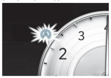
The engine will stop and the green Auto Stop ((A)) indicator on the instrument cluster will appear.
