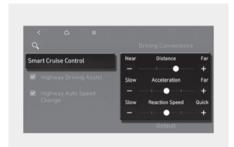
With the ignition switch ON, go to User settings > Driver Assistance > Smart Cruise Control from the settings menu on the instrument cluster or Settings > Vehicle > Driver Assistance > Driving Convenience > Smart Cruise Control in the infotainment system to change Distance, Acceleration, Reaction Speed manually.
