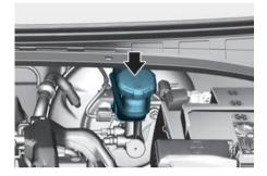
Check the fluid level in the reservoir periodically. The fluid level must be between the MAX and the MIN marks on the side of the reservoir.
