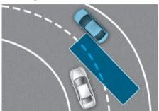
Blind-Spot Collision-Avoidance Assist may not detect a vehicle in an adjacent lane when driving on a curved road and may not activate a warning or brake your vehicle.
