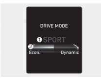
The drive mode selected by the driver (1) and the driving style gauge (2) showing the driver's driving style are displayed on the screen.
