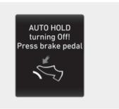
When the conversion from Auto Hold to EPB is not working properly, a warning sounds and a message appears.
