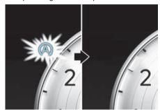
The engine will start and the green Auto Stop indicator ((A)) on the instrument cluster will change to white.
