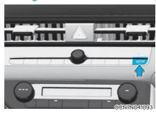
1. Press the SETUP button on the main keyboard.
