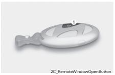
Press and hold the Door Unlock (1) button on the smart key for more than 3 seconds and the front seat windows move down after the doors are unlocked. Window movement stops when you release the door unlock button.
