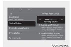
The Warning Methods can be set with the engine on. Select Setup > Vehicle > Driver Assistance > Warning Methods from the settings menu in the infotainment system to change the following settings:
