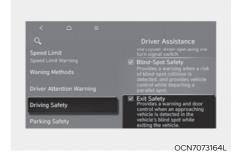
With the engine on, select **Setup** > **Vehicle** > **Driver Assistance** > **Driving Safety** > **Exit Safety** from the Settings menu in the infotainment system to turn on Safe Exit Warning and deselect to turn off the function.
