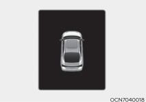
If the driver turns off the engine when the sunroof is not fully closed, the warning chime will sound for several seconds and the sunroof open warning will appear on the cluster display.
