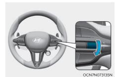
Push the - switch down and release it immediately. The set speed will decrease by 1 mph (1 km/h) each time the switch is operated in this manner.
