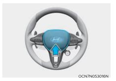
To sound the horn, press the area indicated by the horn symbol on your storying wheel (see illustration). The
