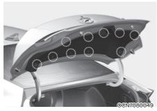
Loosen the retaining screw of the trunk lid cover and then remove the cover.
