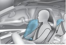
Your vehicle is equipped with a side air bag in each front and outboard second row seat. The purpose of the air bag is to provide the vehicle's additional protection than that offered by the seat belt alone.
