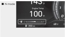
This gauge indicates the approximate amount of fuel remaining in the fuel tank.
