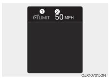
[1]: Manual Speed Limit Assist enabled indicator [2]: Set speed
