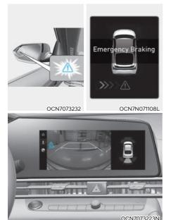
To warn the driver of an approaching detected vehicle from the rear left/right side of your vehicle, the warning light on the side view mirror will blink and a warning message will appear on the instrument cluster. At the same time, an audible warning will sound.
