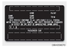
The certification label is located on the driver's door sill at the center pillar and shows the maximum allowable weight of the fully loaded vehicle. This is called the GVWR (Gross Vehicle Weight Rating). The GVWR includes the weight of the vehicle, all occupants, fuel and cargo.
