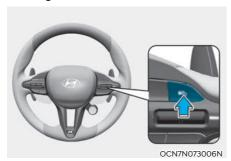
Press the Driving Assist (ﷺ) button to turn Cruise Control off. The Cruise (ﷺ) indicator will go off. Always press the Driving Assist (ﷺ) button to turn Cruise Control off when not in use.
