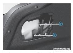
3. Loosen the assembly retaining nuts.
