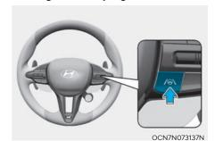
With the vehicle on, press and hold the Lane Driving Assist button located on the steering wheel to turn on and off. When Lane Keeping Assist is on, the grey or green indicator is on.
