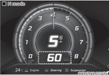
The speedometer indicates the speed of the vehicle and is calibrated in miles per hour (MPH) and/or kilometers per hour (km/h).
