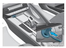
5. Plug the compressor power cord (3) into the vehicle power outlet.
