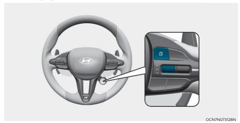
The cluster display modes can be changed by using the control buttons.
