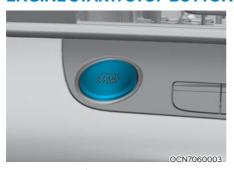
Whenever the front door is opened, the Engine Start/Stop button will illuminate and will go off 30 seconds after the door is closed.
