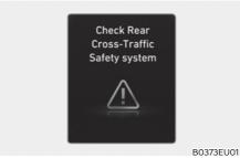
When Rear Cross-Traffic Collision-Avoidance Assist is not working properly, the 'Check Rear Cross-Traffic Safety system' warning message will appear on the instrument cluster for several seconds, and the master \( \infty\) warning light will illuminate on the instrument cluster. If this occurs, have the vehicle inspected by an authorized HYUNDAI dealer.
