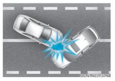
In an angled collision, the force of impact may direct the occupants in a direction where the air bags would not be able to provide any additional benefit, and thus the sensors may not deploy any air bags.
