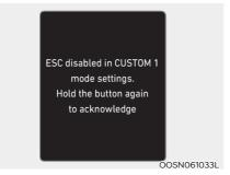
When N1 or N2 button is set to CUSTOM mode, you cannot turn CUSTOM mode on by pressing either N1 or N2 button if ESC OFF setting is saved within CUSTOM mode. If N1 or N2 button is pressed, a message "ESC disabled in CUSTOM 1 (or 2) mode settings. Hold the button again to acknowledge" appears on the cluster display. To turn on CUSTOM mode with ESC OFF setting, press and hold N1 or N2 button.
