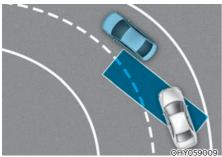
Blind-Spot Collision-Avoidance Assist may not operate properly when driving on a curved road. Blind-Spot Collision-Avoidance Assist may recognize a vehicle in the same lane.
