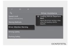
With the engine on, select Settings > Vehicle > Driver Assistance > Driver **Attention Warning** from the settings menu in the infotainment system to set whether to use the function.
