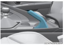
Check the stroke of the parking brake by counting the number of "clicks" heard while fully applying it from the released position. Also, the parking brake alone should securely hold the vehicle on a fairly steep grade. If the stroke is more or less than specified, have the system serviced by an authorized HYUNDAI dealer.
