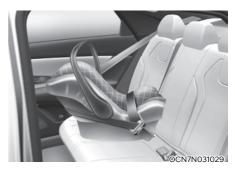
A rear-facing child seat provides restraint with the seating surface against the back of the child. The harness system holds the child in place, and in an accident, acts to keep the child positioned in the seat and reduce the stress to the neck and spinal cord.
