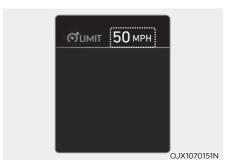
3. The set speed limit will be displayed on the instrument cluster.
