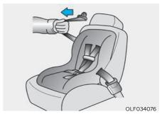
Pull the shoulder portion of the seat belt all the way out. When the shoulder portion of the seat belt is fully extended, it will shift the retractor to the "Automatic Locking" (child restraint) mode.
