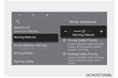
The Warning Methods can be set with the engine on. Select **Setup** > **Vehicle** > **Driver Assistance** > **Warning Methods** from the settings menu in the infotainment system to change the
