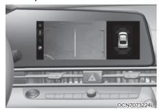
When you touch the icon (3), the top view is displayed on the screen and shows the distance from the vehicle in the back of your vehicle while parking.
