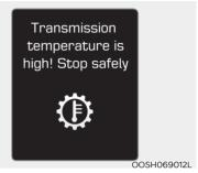
Repeated stop-and-go launches on steep grades, sudden take off or acceleration, or other harsh driving conditions may increase the clutch and transmission temperature.
