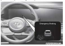
To warn you of a potential collision, the warning light on the side view mirror may blink, a warning message may appear on the instrument cluster, and an audible warning may sound and the steering wheel will vibrate.
