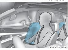
Your vehicle is equipped with a side airbag in each front seat and rear seat. The purpose of the airbag is to provide the vehicle's driver and the front passenger with additional protection than that offered by the seat belt alone.
