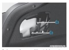
3. Loosen the assembly retaining nuts.
