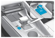
To apply the EPB (Electronic Parking Brake):
