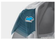
Remove the rear combination light assembly from the body of the vehicle.
