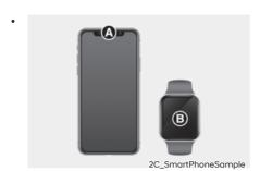
The NFC Antenna position on Apple iPhone is located at the top of the rear [A] and Apple WATCH is located at the center of the screen [B].
