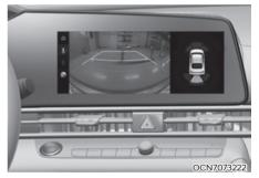
Shift the gear to R (Reverse), the rear view will appear on the screen.
