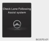
When Lane Following Assist is not working properly, the "Check Lane Following Assist system" message may appear, and the A warning light may illuminate on the instrument cluster. Have the vehicle inspected by an authorized HYUNDAI dealer.
