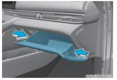
Push in both sides of the glove box as shown. This will ensure that the glove box stopper pins will get released from its holding location allowing the glove box to hang.
