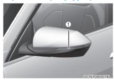
If the LED lamp (1) does not operate, have the vehicle checked by an authorized HYUNDAI dealer.
