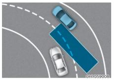
Blind-Spot Collision-Avoidance Assist may not operate properly when driving on a curved road. Blind-Spot Collision-Avoidance Assist may not detect the vehicle in the next lane. Always pay attention to road and driving conditions while driving.
