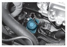
In normal driving conditions, the actuator fluid level does not go down rapidly. However, oil consumption rate may rise as vehicle mileage increases, and leak-age in actuator related parts may result in increased consumption of the engine clutch actuator oil. Regularly check and make sure the engine clutch actuator oil fluid level is between MIN and MAX marks
