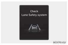
When Lane Keeping Assist is not working properly, the 'Check Lane Keeping Assist (LKA) system' warning message will appear and the yellow / indicator light will illuminate on the cluster. If this occurs, have the vehicle inspected by an authorized HYUNDAI dealer.
