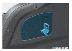
Remove the service cover by pulling out the service cover.
