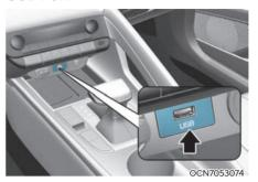
The USB port can be used while the engine is running.
