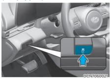
The Electronic Stability Control (ESC) system helps to stabilize the vehicle during cornering maneuvers. ESC checks where you are steering and where the vehicle is actually going. ESC applies braking pressure to any one of the vehicle's brakes and intervenes in the engine management system to assist the driver with keeping the vehicle on the intended path. It is not a substitute for safe driving practices. Always adjust your speed and driving to the road conditions.
