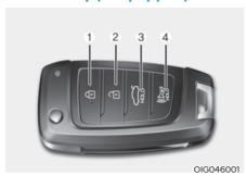
Your HYUNDAI uses a remote key, which you can use to lock or unlock the driver and passenger doors or the rear trunk.
