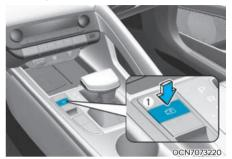
Press the Parking/View button (1) while the gear is in P (Park) to turn on Rear View Monitor.
