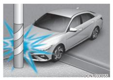
Airbags may not inflate if the vehicle collides with objects such as utility poles or trees, where the point of impact is concentrated and the collision energy is absorbed by the vehicle structure.
