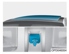
If you push the sunroof control lever upward towards the roof of the vehicle, the sunshade will slide open then the sunroof glass will tilt open.
