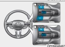
To change the trip mode, toggle the "\( \chi, \vec \)" switch on the steering wheel.
