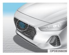
The Smart Cruise Control uses a sensor to detect distance to the vehicle ahead.
