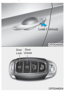
Press the button on the driver's outside door handle while carrying the Smart Key with you or press the Door Unlock button on the Smart Key, the driver's door will unlock.
