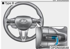
Push the toggle switch down (SET-) and hold it. Your vehicle will gradually slow down. Release the toggle switch at the speed you want to maintain.
