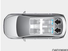
LATCH anchors have been provided in the left and right outboard rear seating positions. Their locations are shown in the illustration. There are no LATCH anchors provided for the center rear seating position.
