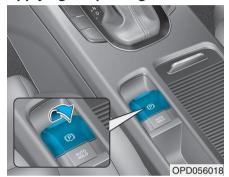
To apply the EPB (Electronic Parking Brake):
