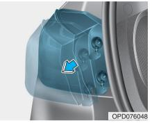
5. Remove the rear combination lamp assembly from the body of the vehicle.
