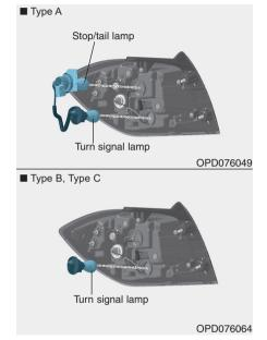
Remove the socket from the assembly by turning the socket counterclockwise until the tabs on the socket align with the slots on the assembly.
