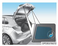
Type A - Tail lamp and backup lamp Type B, Type C - Backup lamp
