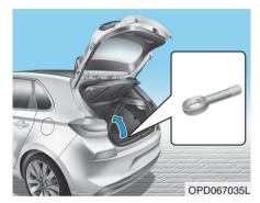
1. Open the tailgate and remove the towing hook from the tool case.
