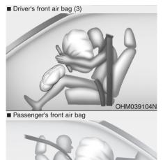
After complete inflation, the air bag immediately starts deflating, enabling the driver to maintain forward visibility and the ability to steer or operate other controls.
