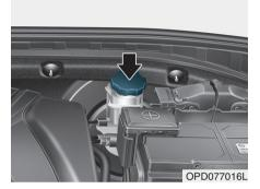
Check the fluid level in the reservoir periodically. The fluid level should be between MAX and MIN marks on the side of the reservoir.
