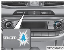
As a reminder to the front passenger, the front passenger's seat belt warning lights will illuminate for approximately 6 seconds each time you place the ignition switch to the ON position regardless of belt fastening. If you continue not to fasten the seat belt and you drive over 9 km/h (6 mph), the warning light will stay illuminated
