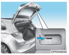
Your vehicle is equipped with an Emergency Tailgate Safety Release lever located inside the tailgate. When someone is inadvertently locked in the luggage compartment, the tailgate can be opened manually from inside the luggage compartment by performing the following steps:
