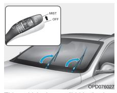
This vehicle has a "hidden" wiper design which means that the wipers cannot be lifted when they are in their bottom resting position.
