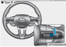
Push the toggle switch up (RES+) and hold it, while monitoring the SET speed on the instrument cluster. Release the toggle switch when the desired speed is shown and the vehicle will accelerate to that speed.
