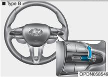
Push the toggle switch up (RES+). If the vehicle speed is over 30 km/h (20 mph), the vehicle will resume the preset speed.
