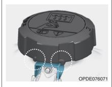
2. Make sure that the tiny protrusions inside the coolant cap is securely interlocked.
