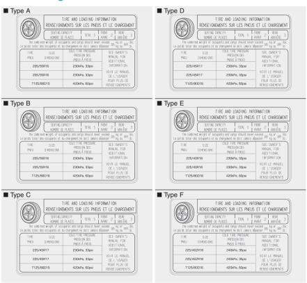
The label located on the driver's door sill gives the original tire size, cold tire pressures recommended for your vehicle, the number of people that can be in your vehicle and vehicle capacity weight.
