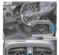
The outlet vents can be opened (இ) or closed (○) separately using the thumbwheel.
