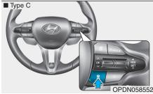
When the Smart Cruise Control System is ON, you can set and maintain the distance from the vehicle ahead of you without pressing the accelerator or brake pedal.
