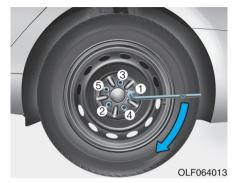
13. Use the wheel lug nut wrench to tighten the lug nuts in the order shown. Double-check each lug nut until they are tight. After changing tires, have an authorized HYUNDAI dealer tighten the lug nuts to their proper torque as soon as possible. The wheel lug nut should be tightened to 11~13 kgf·m (79~94 lbf·ft).
