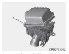
Be sure to insert the hinge (A) before locking the cover with the cover attaching clips.
