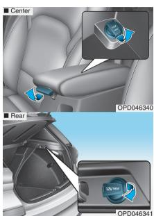
The power outlet is designed to provide power for mobile telephones or other devices designed to operate with vehicle electrical systems. The devices should draw less than 180 W (Watts) with the engine running.
