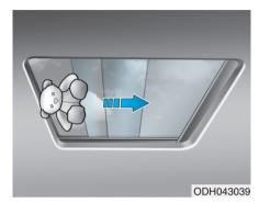
If the sunroof senses any obstacle while it is closing automatically, it will reverse direction then stop to allow the object to be cleared.
