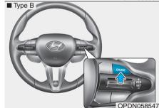
1. Push the CRUISE button on the steering wheel to turn the system on. The cruise ( CRUISE) indicator will illuminate.
