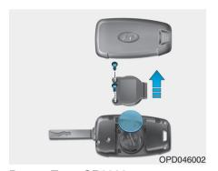
Battery Type: CR2032 To replace the battery:
