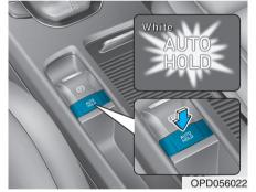
1. With the driver's door, engine hood and tailgate closed, fasten the driver's seat belt or depress the brake pedal and then press the [AUTO HOLD] switch. The white AUTO HOLD indicator will come on and the system will be in the standby position.
