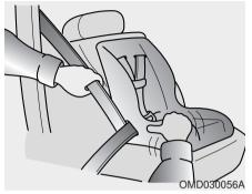
To remove the child restraint, press the release button on the buckle and then pull the lap/shoulder belt out of the restraint and allow the seat belt to retract fully.
