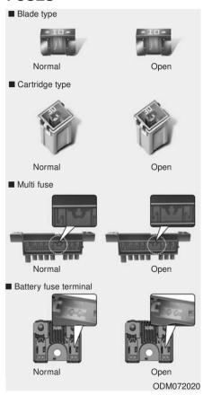
The electrical system is protected by fuses.
