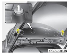
4. Using a flat-blade screwdriver, gently pry the tailgate upper trim.
