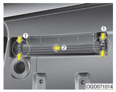
3. Remove the climate control air filter cover (2) while pressing the lock (1).
