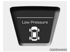
When the tire pressure monitoring system warning indicator is illuminated, one or more of your tires is significantly under-inflated.
