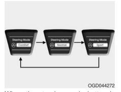
When the steering mode button is pressed, the selected steering mode will appear on the LCD display.
