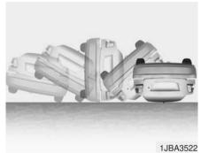
Airbags may not inflate in most rollover accidents, even though the vehicle is equipped with side impact air bags and curtain air bags.
