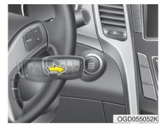
When the battery is weak, if the engine start/stop button is depressed, the indicator will blink and you will not be able to start the engine. However, you may still be able to start the engine by pressing the engine start/stop button with the smart key. If smart key system related parts need repair, the indicator blinks.
