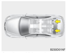
Securing a child restraint seat with child seat lower anchor system
