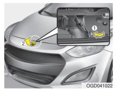
2. Go to the front of the vehicle, raise the hood slightly, pull the secondary latch (1) inside of the hood center and lift the hood (2).
