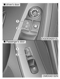
With central door lock switch (if equipped)
