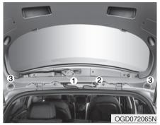
5. Disconnect the connector(1) and remove the washer hose(2) and the plug holes(3).
