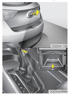
If you move the shift lever to the R (Reverse) position with the ignition switch on, the back-up light will illuminate, the rearview camera cover will open and then the rearview camera will activate.
