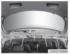
6. Remove the mounting nuts.
