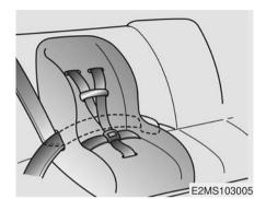
Placing a passenger seat belt into the automatic locking mode
