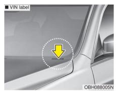
The vehicle certification label attached on the driver's side center pillar contains the vehicle identification number (VIN). The VIN is also on a plate attached to the top of the dashboard. The number on the plate can easily be seen through the windshield from outside.
