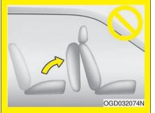
Never let the rear seat touch the front passenger seat when folding the rear seat. The occupant classification system (OCS) may malfunction, the PASS AIR BAG "OFF" indicator may turn on even though the front passenger's seat is occupied by an adult, or the SRS air bag warning light on the instrument panel may illuminate.
