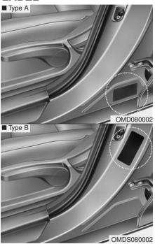
The vehicle certification label attached on the driver's side center pillar contains the vehicle identification number (VIN).
