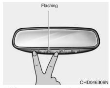
1. When programming the buttons for the first time, press and hold the left and center buttons (全, 金) simultaneously until the indicator light begins to flash after approximately 20 seconds. (This procedure erases the factory-set default codes. Do not perform this step to program additional hand-held transmitters.)
