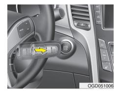
When the battery is weak, if the engine start/stop button is depressed, the indicator will blink and you will not be able to start the engine. However, you may still be able to start the engine by pressing the engine start/stop button with the smart key. If smart key system related parts need repair, the indicator blinks.
