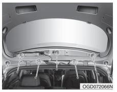
6. Remove the mounting nuts.
