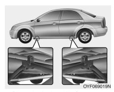
Place the jack at the front or rear jacking position closest to the tire you are changing. Place the jack at the designated locations under the frame.
