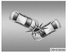
In an angled collision, the force of impact may direct the occupants in a direction where the air bags would not be able to provide any additional benefit, and thus the SRS may not deploy any air bags.
