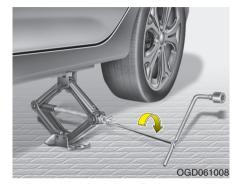
8. Insert the jack handle into the jack and turn it clockwise, raising the vehicle until the tire just clears the ground by approximately 1.2 in (30 mm). Before removing the wheel lug nuts, make sure the vehicle is stable and that there is no chance for movement or slippage.
