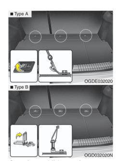
Securing a child restraint seat with "Tether Anchor" system
