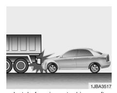
Just before impact, drivers often brake heavily. Such heavy braking lowers the front portion of the vehicle causing it to "ride" under a vehicle with a higher ground clearance. Air bags may not inflate in this "under-ride" situation because forces that are detected by sensors may be reduced by such "underride" collisions.
