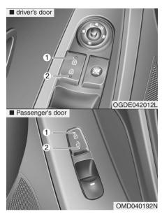
With central door lock switch (if equipped)
