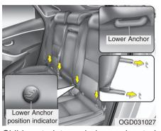
Child restraint symbols are located on the outboard left and right rear seat backs to indicate the position of the lower anchors for child restraints.
