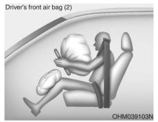
Upon deployment, tear seams molded directly into the pad covers will separate under pressure from the expansion of the air bags. Further opening of the covers then allows full inflation of the air bags.
