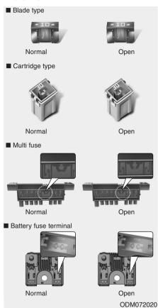
The electrical system is protected by fuses.
