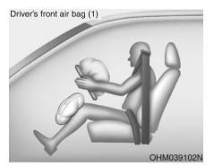
The front air bag modules are located in the center of the steering wheel, in the front passenger's panel above the glove box and in the driver's side knee bolster. When the SRSCM detects a sufficiently severe impact to the front of the vehicle, it will automatically deploy the front air bags.
