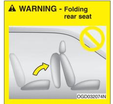
Never let the rear seat touch the front passenger seat when folding the rear seat. The occupant classification system (OCS) may malfunction, the PASS AIR BAG "OFF" indicator may turn on even though the front passenger's seat is occupied by an adult, or the SRS air bag warning light on the instrument panel may illuminate.
