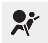
SRS warning light
