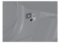
2 Locate the hood latch lever, push it to the side, and then raise the hood. Once you have raised the hood slightly, you can release the lever.
