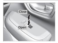
**To open:** Push the switch down. **To close:** Pull the switch up.
