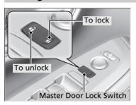
Press the master door lock switch in as shown to lock or unlock all the doors, fuel fill door, and tailgate.
