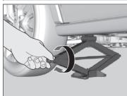
the image until the top of the jack contacts the jacking point.
