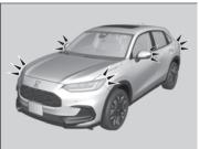
If the engine stop successfully, the exterior lights flash once.
