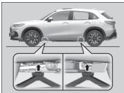
**1.** Place the jack under the jacking point closest to the tire to be changed.
