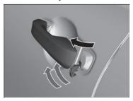
Pull and hold the outer handle. Insert the built-in key into the key cylinder from below the handle and then turn it.
