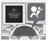
■ When the power mode is set to ON The indicator comes on for a few seconds, then goes off. This tells you the system is working properly.
