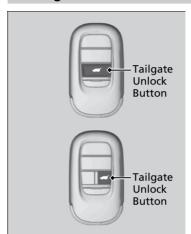
Press the tailgate unlock button to unlock the tailgate.
