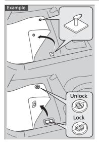
The driver's floor mat hooks over the floor anchors, which keep the mat from sliding forward.
