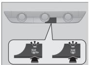
The rear defogger and heated door mirror\* automatically switch off after 10-30 minutes depending on the outside temperature. However, if the outside temperature is 32°F (0°C) or below, it does not automatically switch off.
