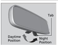
Flip the tab to switch the position. The night position will help reduce the glare from headlights behind you when driving after dark.
