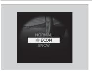
Facilitates fuel-efficient driving.
