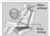
The driver's and front passenger's knee airbag deploy at the same time as the driver's and front passenger's airbag respectively.
