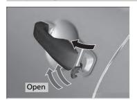
Pull and hold the outer handle. Insert the key into the key cylinder completely from below the handle.
