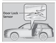
The vehicle will automatically lock after you lock the doors in advance then close the doors and tailgate.
