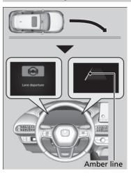
The front wide view camera behind the rearview mirror monitors left and right lane markings in white or yellow, the outer edge of the pavement (into grass or gravel road shoulder) or a detected oncoming vehicle. If your vehicle approaches any detected lane markings, the outer edge of the pavement (into grass or gravel road shoulder) or a detected oncoming vehicle when the turn signals have not been engaged, the system activates.
