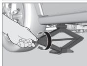
2. Turn the end bracket clockwise as shown in the image until the top of the jack contacts the jacking point.
