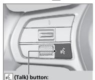
Press and hold to operate Android Auto with your voice. Press and release to activate standard voice recognition system.
