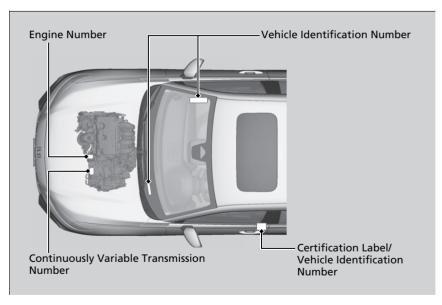
➤ Vehicle Identification Number (VIN), Engine Number, and Transmission Number
