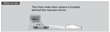
The system starts monitoring the roadway ahead when your vehicle speed is about 3 mph (5 km/h) or above and will search for a vehicle, pedestrian, or moving bicycle in front of you.
