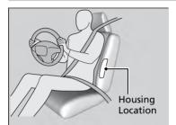
The side airbags are housed in the outside edge of the driver's and passenger's seat-backs and next to the outer rear seating positions.
