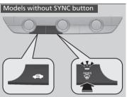
Pressing the button turns the air conditioning system on and automatically switches the system to fresh air mode.
