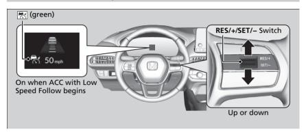
When driving at about 25 mph (40 km/h) or above: Take your foot off the pedal and press the RES/+/SET/– switch up or down when you reach the desired speed. The moment you release the switch, the set speed is fixed, and ACC with Low Speed Follow begins.
