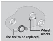
**4.** Place a wheel block or rock in front and rear of the wheel diagonal to the flat tire.
