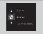
1. Press the (home) button and roll the left selector wheel to select **Settings**, then press the left selector wheel.
