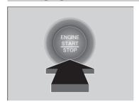
If you carry the keyless remote and press **ENGINE START/STOP** button without depressing the brake pedal, the power mode will change in this order: VEHICLE OFF→ACCESSORY→ON→ VEHICLE OFF.
