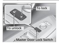
Press the master door lock switch in as shown to lock or unlock all the doors, fuel fill door, and tailgate.
