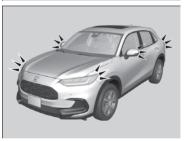
If the engine stop successfully, the exterior lights flash once.
