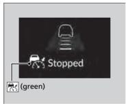
If no vehicle is ahead of you before you resume driving, depress the accelerator pedal and ACC with Low Speed Follow will operate again within the prior set speed.
