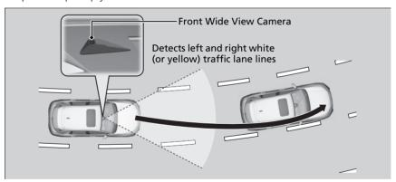
When you use the turn signal to indicate a lane change, Traffic Jam Assist is temporarily deactivated. It is reactivated once the vehicle is traveling in the center of the lane and the system has detected the traffic lane lines.
