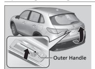
When all the doors are unlocked or press the tailgate unlock button on the remote transmitter, the tailgate is unlocked. Press the tailgate outer handle and lift open the tailgate.
