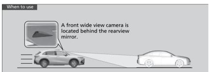
Vehicle speed for ACC with Low Speed Follow: A vehicle is detected ahead within ACC with Low Speed Follow range – ACC with Low Speed Follow operates at speeds up to 90 mph (145 km/h).
