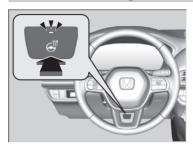
The heated steering wheel can be used when the power mode is in ON.
