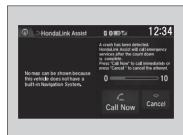
If your vehicle's airbags deploy or if the unit detects that the vehicle is severely impacted, your vehicle automatically will attempt to connect to the HondaLink operator. If connected, information about your vehicle, its location, and its condition will be sent to the operator; you also can speak to the operator when connected.
