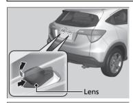
**1.** Push the lens on the left and pull out the lens and the socket attached to it.
