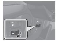
2 Locate the hood latch lever, push the lever, and lift up the hood.
