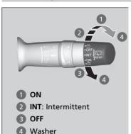
The rear wiper and washer can be used when the ignition switch is in ON  $[II]^{*1}$ .
