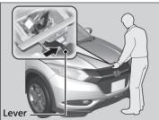
**3.** Pull up the hood latch lever in the center of the hood to release the lock mechanism, and open the hood.
