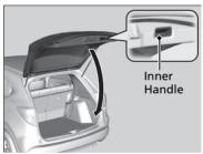
To close the tailgate, grab the inner handle, pull the tailgate down, and push it closed from outside
