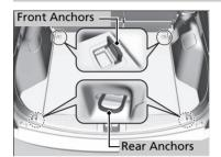
The tie-down anchors on the cargo area floor can be used to install a net for securing items.
