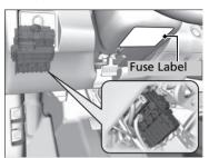
Located behind the instrument panel. Fuse locations are shown on the label under the steering column.
