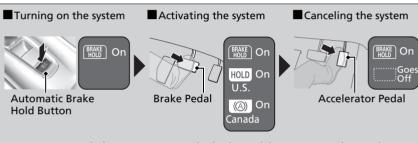
Fasten your seat belt properly, then start the engine. Press the automatic brake hold button.
