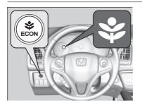
The **ECON** button turns the ECON mode on and off. The ECON mode helps you improve your fuel economy by adjusting the performance of the engine, transmission, heating and cooling system\*/climate control system\*, and cruise control.
