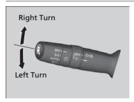
The turn signals can be used when the ignition switch is in ON II \*1.
