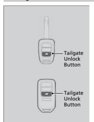
Press the tailgate unlock button to unlock the tailgate.
