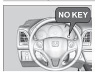
Warning buzzers may sound from inside and/ or outside the vehicle to remind you that the smart entry remote is out of the vehicle. If the buzzer continues even after the remote is put back inside, place it to be within its operational range.
