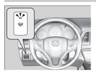
Press the heated windshield button to deice the windshield when the ignition switch is turned to ON  $\boxed{II}^{*1}$ .
