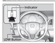
Press the LDW button to turn the system on and off.
