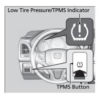
Press and hold the TPMS button until the low tire pressure/TPMS indicator blinks twice, indicating the calibration process has begun.
