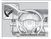
When the ignition switch is in ON III\*1, you can use the (a) (select/reset) knob to adjust instrument panel brightness.
