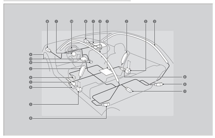
The front, front side, and side curtain airbags are deployed according to the direction and severity of impact. Both side curtain airbags are deployed in a rolloyer. The airbag system includes:
