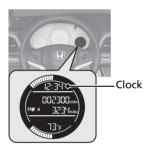
The clock in the information display is automatically updated along with the audio system's clock display.
