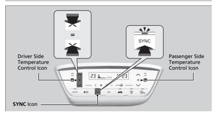
You can set the temperature synchronously for the driver side and the passenger side in synchronized mode.
