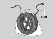
**5.** Bore through the bag, and pass the holding belt through the hole of the bag and the wheel of the flat tire as shown.
