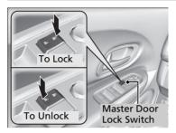
Press the master door lock switch in as shown to lock or unlock all the doors and the tailgate.
