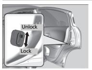
Slide the lever in the rear door to the lock position, and close the door.
