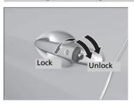
If the remote battery or the vehicle battery is dead, use the key instead of the remote. Fully insert the key and turn it.
