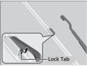
**2.** Press and hold the tab, then slide the holder off the wiper arm.
