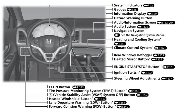
$<sup>{\</sup>bf *1:}\ Models\ with\ the\ smart\ entry\ system\ have\ an\ {\bf ENGINE\ START/STOP}\ button\ instead\ of\ an\ ignition\ switch.$
