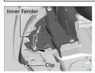
**1.** Remove the clip using a flat-tip screwdriver, and push up the inner fender.
