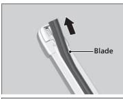
**3.** Slide the wiper blade out of the holder by pulling the tabbed end out.
