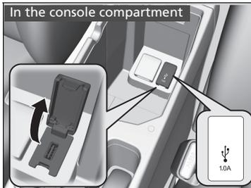
Install the iPod USB connector or the USB flash drive to the USB port.
