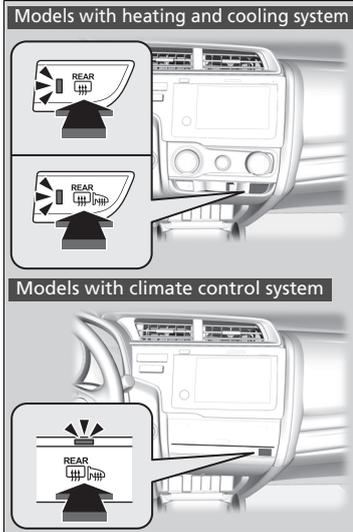
Press the rear defogger and heated door mirror button or touch the icon to defog the rear window and mirrors when the ignition switch is in ON
