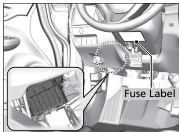
Located behind the instrument panel. Fuse locations are shown on the label under the steering column. Locate the fuse in question by the fuse number and label number.
