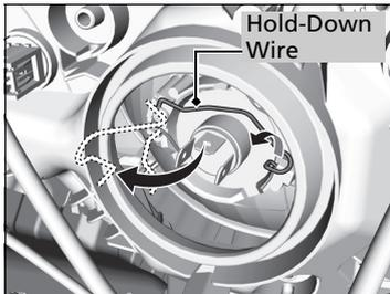
3. Remove the hold-down wire, then remove the bulb.
