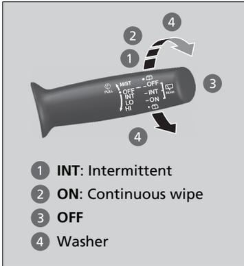
The rear wiper and washer can be used when the ignition switch is in ON \*1.
