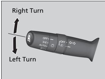
The turn signals can be used when the ignition switch is in ON
