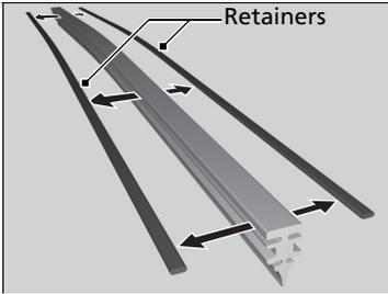
4. Remove the retainers from the wiper blade and mount to a new rubber blade.
