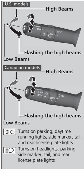
Rotating the light switch turns the lights on and off, regardless of the position of the ignition switch\*<sup>1</sup>.
