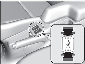
While in **HI**, the heater cycles on and off.
