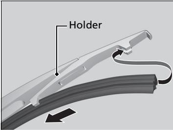
5. Slide the wiper blade onto the holder.
