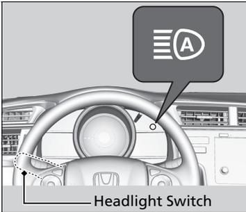
To activate the system, turn the headlight switch to **AUTO** and then set the headlights to low beam. The auto high-beam indicator will come on.
