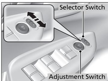
You can adjust the door mirrors when the ignition switch is in ON
