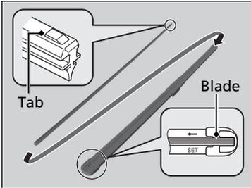
4. Slide the new wiper blade onto the holder from the bottom end.
