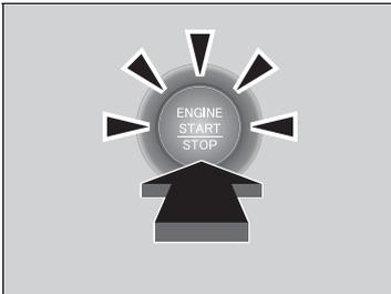
1. Touch the center of the **ENGINE START/STOP** button with the **H** logo on the smart entry remote while the **ENGINE START/STOP** button is flashing. The buttons on the smart entry remote should be facing you.
