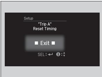
6. Press the button until **Exit** appears on the display, then press the **SEL/RESET** button.
