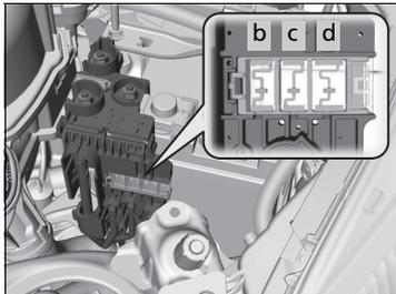
Pull up the cover on the ⊕ terminal, then remove it while pulling out the tab as shown.
