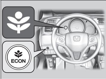
The **ECON** button turns the ECON mode on and off. The ECON mode helps you improve your fuel economy by adjusting the performance of the engine, transmission, climate control system\*, and cruise control\*.
