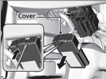
Remove the cover by putting the flat-tip screwdriver into the side slot as shown.
