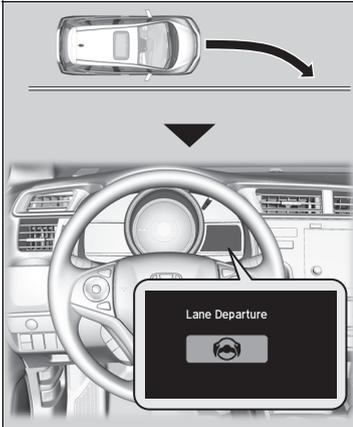
The front camera behind the rearview mirror monitors left and right lane markings (in white or yellow). If your vehicle is getting too close to detected lane markings without a turn signal activated, the system, in addition to a visual alert, applies steering torque and alerts you with rapid vibrations on the steering wheel, to help you remain within the detected lane.
