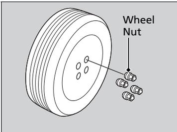
1. Remove the wheel nuts and flat tire.
