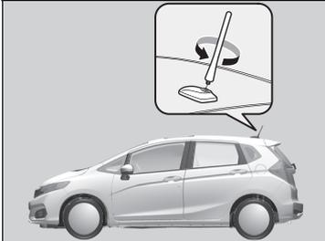
Your vehicle is equipped with a removable antenna at the rear of the roof.
