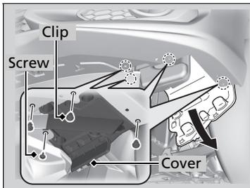
1. Remove the screws using a Phillips-head screwdriver and remove the holding clips using a flat-tip screwdriver.
