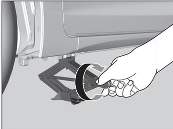
2. Turn the end bracket as shown in the image until the top of the jack contacts the jacking point.
