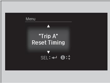
4. Press the button until **"Trip A" Reset Timing** appears on the display, then press the **SEL/RESET** button.
