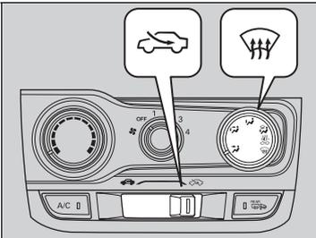
1. Selecting turns the air conditioning system on.
