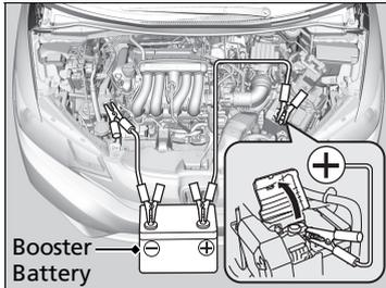
1. Connect the first jumper cable to your vehicle's battery  $\oplus$  terminal.
