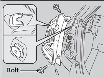
1. Use a Phillips-head screwdriver to remove the bolts.
