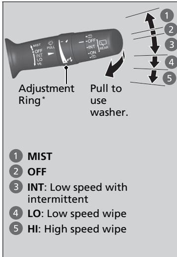
The windshield wipers and washers can be used when the ignition switch is in ON \*1.
