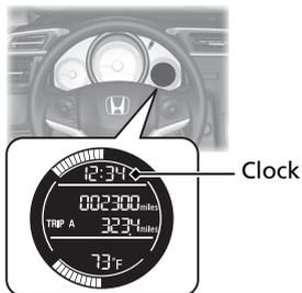
The clock in the information display is automatically updated along with the audio system's clock display.
