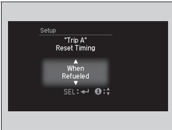
5. Press the button and select **When Refueled**, then press the **SEL/RESET** button.
