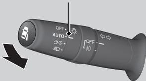
Disable or re-enable the system when the vehicle is parked and the ignition switch is in ON **II**\*<sup>1</sup> and the light switch is in the **AUTO** position.
