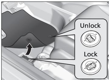
The driver's floor mat hooks over floor anchors, which keep the mat from sliding forward. To remove a mat for cleaning, turn the anchor knobs to the unlock position. When reinstalling the mat after cleaning, turn the knobs to the lock position.
