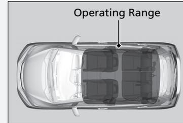
The engine may also run if the smart entry remote is close to the door or window, even if it is outside the vehicle.
