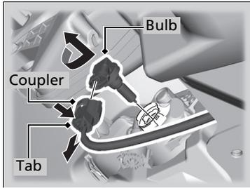
3. Push the tab to remove the coupler.
