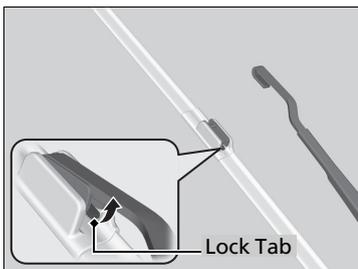
2. Press and hold the tab, then slide the holder off the wiper arm.
