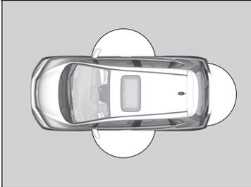
When you carry the smart entry remote, you can lock/unlock the doors and the tailgate. You can lock/unlock the doors and the tailgate within a radius of about 32 inches (80 cm) of the outside door handle or tailgate release button.
