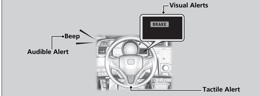
At system's earliest collision alert stage, you can change the distance (**Long/Normal/Short**) between vehicles at which alerts will come on through multi-information display setting options.
