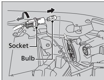
1. Turn the socket counter-clockwise and remove it.
