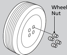
1. Remove the wheel nuts and flat tire.
