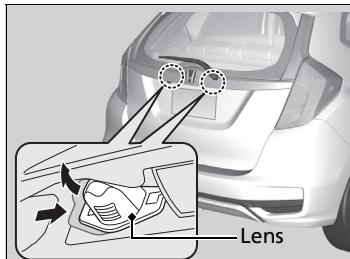
1. Push the lens on the left and pull out the lens and the socket attached to it.
