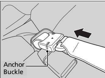
2. Line up the triangle marks on the small latch plate and anchor buckle.
