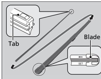
**4.** Slide the new wiper blade onto the holder from the bottom end.
