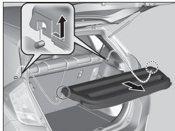
3. Disengage the support rods, then remove the cargo area cover.
