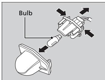
2. Remove the license plate light assembly by squeezing the tabs on both sides of the socket.
