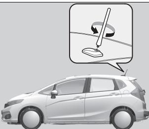
Your vehicle is equipped with a removable antenna at the rear of the roof.
