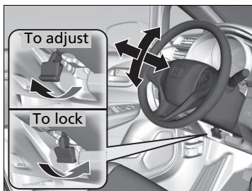
1. Pull the steering wheel adjustment lever up.
