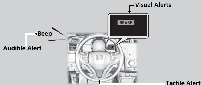
At system's earliest collision alert stage, you can change the distance (**Long** / **Normal/Short**) between vehicles at which alerts will come on through multi-information display setting options.
