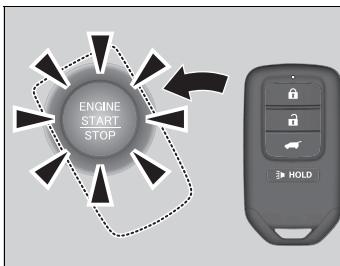
1. Touch the center of the **ENGINE START/STOP** button with the **H** logo on the smart entry remote while the **ENGINE START/STOP** button is flashing. The buttons on the smart entry remote should be facing you.
