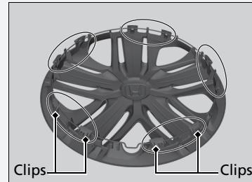
Align the valve mark on the wheel cover to the tire valve on the wheel, then install the wheel cover.
