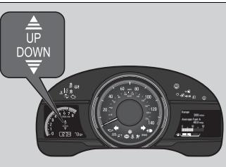
Come on to inform you that upshifting or downshifting is necessary to prevent the engine from over revving or stalling.
