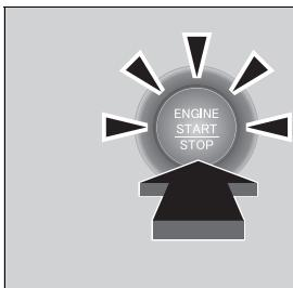
2. Depress the brake pedal (continuously variable transmission) or clutch pedal (manual transmission) and press the **ENGINE START/STOP** button within 10 seconds after the beeper sounds and the **ENGINE START/STOP** button changes from flashing to on.
