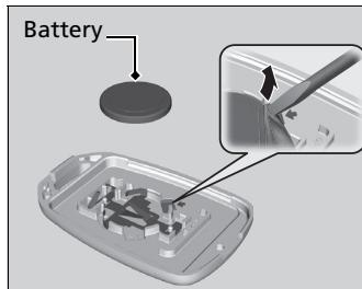
» Replacing the Button Battery
