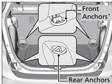
The tie-down anchors on the cargo area floor can be used to install a net for securing items.
