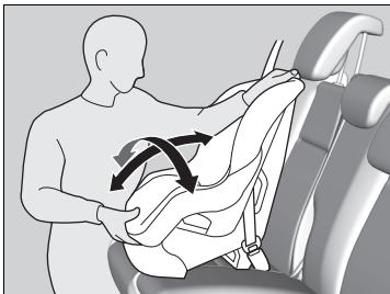
7. Make sure the child seat is firmly secured by rocking it forward and back and side to side; less than one inch of movement should occur near the seat belt.
