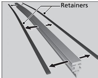
**4.** Remove the retainers from the wiper blade and mount to a new rubber blade.
