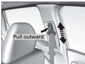
1. Move the anchor up and down while pulling the release outward.
