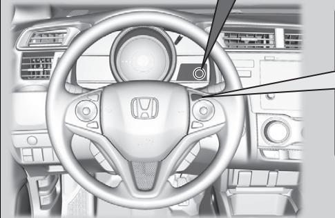
■ Press the **MAIN** button on the steering wheel.
