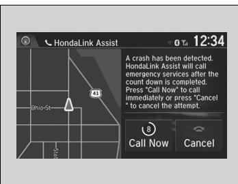
If your vehicle's airbags deploy or if the unit detects that the vehicle is severely impacted, your vehicle automatically will attempt to connect to the HondaLink® operator. If connected, information about your vehicle, its location, and its condition can be sent to the operator\*<sup>1</sup>; you also can speak to the operator when connected.
