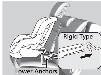
3. Place the child seat on the vehicle seat, then attach the child seat to the lower anchors according to the instructions that came with the child seat.
