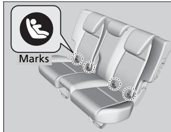
1. Locate the lower anchors under the marks.
