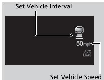
When ACC starts operating, the vehicle icon, interval bars and set speed appear on the multi-information display.
