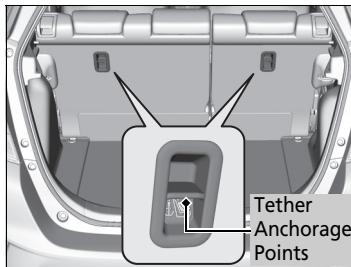
A tether anchorage point is provided behind each rear seating position.
