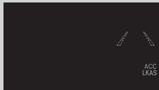
When the LKAS is suspended, the lane lines on the multi-information display change to contour lines, and the beeper sounds (if activated).
