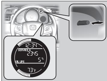
1. Turn the ignition switch to ON **II**<sup>\*1</sup>.
