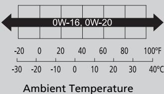
Use a Genuine Honda Motor Oil or another commercial engine oil of suitable viscosity for the ambient temperature as shown.
