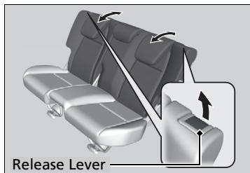
Pull the lever on the right to change the angle of the right half of the seat-back, and left for the left half.
