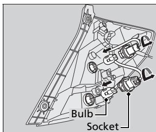
3. Turn the socket counter-clockwise and remove it. Remove the old bulb.
