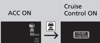
Press and hold the
