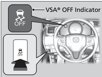
This button is on the driver side control panel. To partially disable VSA<sup>®</sup> functionality/features, press and hold it until you hear a beep.
