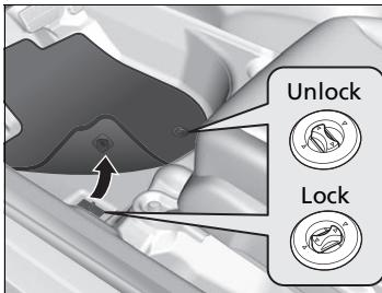
The driver's floor mat hooks over floor anchors, which keep the mat from sliding forward. To remove a mat for cleaning, turn the anchor knobs to the unlock position. When reinstalling the mat after cleaning, turn the knobs to the lock position.
