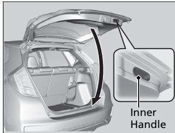
To close the tailgate, grab the inner handle, pull the tailgate down, and push it closed from outside.
