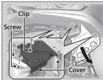
1. Remove the screws using a Phillips-head screwdriver and remove the holding clips using a flat-tip screwdriver.
