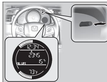
1. Turn the ignition switch to ON **II**<sup>\*1</sup>.
