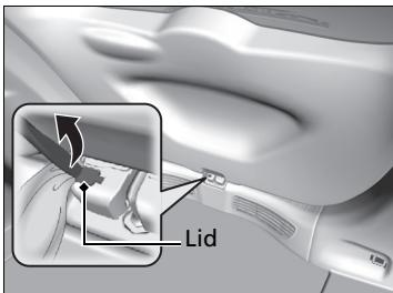
1. Wrap a cloth around the flat-tip screwdriver. Put it into the lid as shown in the image, and open the lid.
