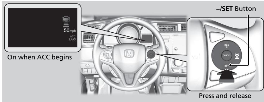
Take your foot off the pedal and press down the **-/SET** button when you reach the desired speed. The moment you release the button, the set speed is fixed, and ACC begins.
