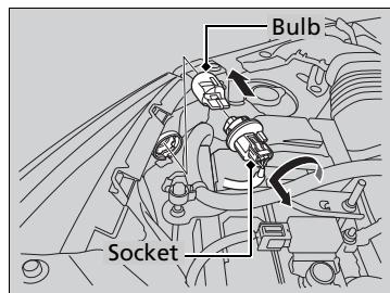
1. Turn the socket counter-clockwise and remove it.
