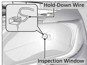
5. Reinstall the hold-down wire. Hook the end of the wire on the knob in the slot.
