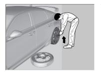
**7.** Loosen each wheel nut about one turn using the wheel nut wrench.
