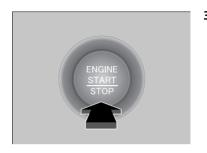
**3.** Press the **ENGINE START/STOP** button without depressing the accelerator pedal.
