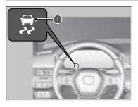
When VSA activates, you may notice that the engine does not respond to the accelerator. You may also notice some noise from the hydraulic brake system. You will also see the indicator blink.
