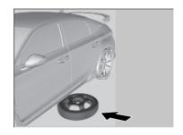
**6.** Place the compact spare tyre (wheel side up) under the vehicle body, near the tyre that needs to be replaced.
