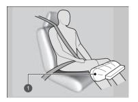
Deployed Passenger's Knee Airbag
