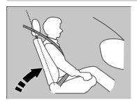
Adjust the driver's seat-back to a comfortable, upright position, leaving ample space between your chest and the airbag cover in the centre of the steering wheel.
