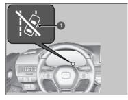
Road Departure Mitigation System Steering Assist Auto OFF indicator If the system operates several times without detecting driver response, the system beeps to alert you. After that, the Road Departure Mitigation System Steering Assist Auto OFF indicator comes on, the Road Departure Mitigation steering assist is temporarily stopped, and the system will only alert you with the warning sound.
