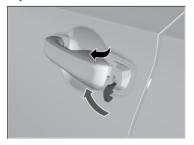
Insert the key into the key cylinder from below the handle and then turn it.
