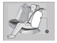
Deployed Side Airbag
