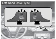
The rear demister and heated door mirrors\* automatically switch off after 10-30 minutes depending on the outside temperature. However, if the outside temperature is 0°C or below, they do not automatically switch off.
