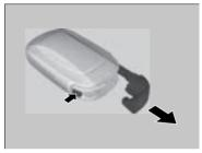
Battery type: Manganese dioxide Lithium battery CR2032
