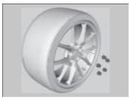
1. Remove the wheel nuts and flat tyre.
